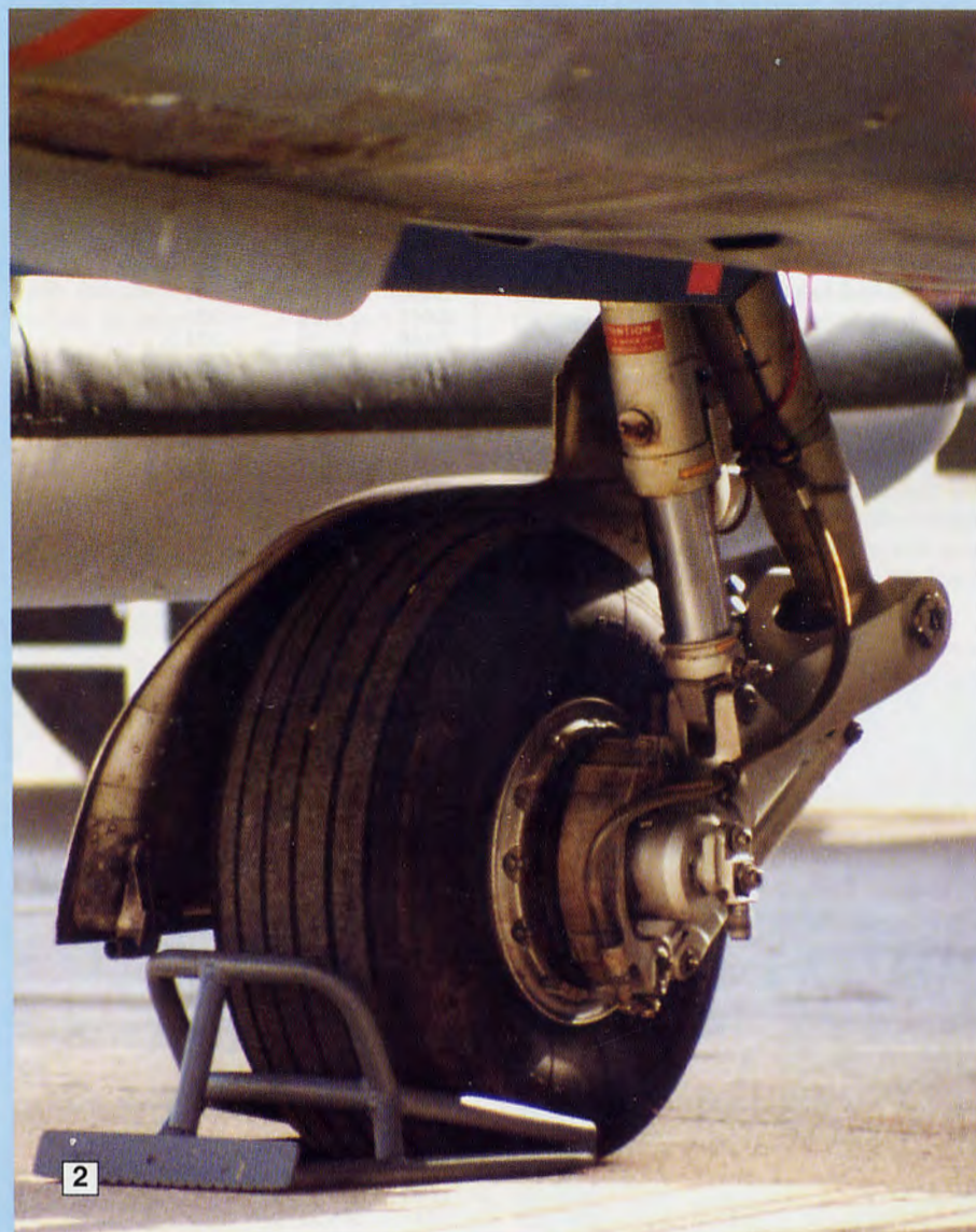
1. The nose wheel undercarriage of the G.91R showing the width of the nose wheel tyre and large heavy duty strut. 2. The port main undercarriage wheel again emphasising the size of the tyre and struts. 3. The G.91Rs canopy and ejector seat. The top of the cockpit entry ladder is just visible. 4. The G.91 flaps were large for short field landing capability.
