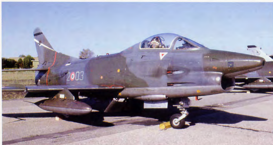
Above: This 'Gina' shows signs of heavy use and recent firing of its 12.7mm Brownings. Note low visibility markings and codes and the late style raised cockpit canopy which indicates that it has been retrofitted with a zero-zero ejector seat. Below: A G.91R of the 14 o Gruppo, 2 o Stormo AMI in early style markings. Note the stencil type unit numbers on the fuselage (Giuseppe Fassari)
