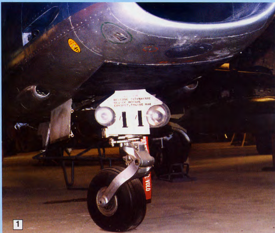
1. The nose wheel undercarriage of the G.91R showing the width of the nose wheel tyre and large heavy duty strut. 2. The port main undercarriage wheel again emphasising the size of the tyre and struts. 3. The G.91Rs canopy and ejector seat. The top of the cockpit entry ladder is just visible. 4. The G.91 flaps were large for short field landing capability.
