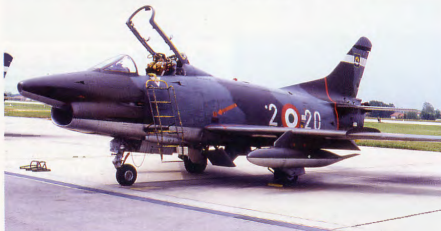
Above: This 'Gina' shows signs of heavy use and recent firing of its 12.7mm Brownings. Note low visibility markings and codes and the late style raised cockpit canopy which indicates that it has been retrofitted with a zero-zero ejector seat. Below: A G.91R of the 14 o Gruppo, 2 o Stormo AMI in early style markings. Note the stencil type unit numbers on the fuselage (Giuseppe Fassari)
