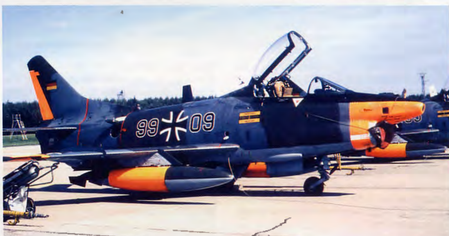
Above: G.91R/3. 99+09, operated by Condor Flug. Target towing equipment was usually fitted to the port side of the wing (Giuseppe Fassari) Below: Port side view of an unarmed G.91R/3 operated by Condor Flug, 99+11, clearly displaying the tow-target fitted to the outer port pylon (José C.C. Silva Collection)
