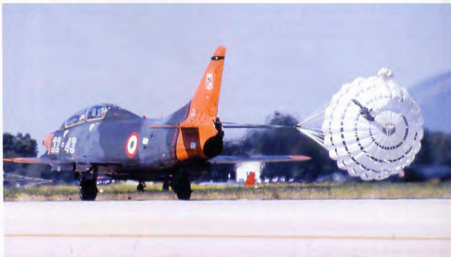
G.91T of the 32° Stormo deploys its braking parachute after landing. These aircraft were assigned to front line units to aid in continuity and conversion training of their aircrews (Giuseppe Fassari)
