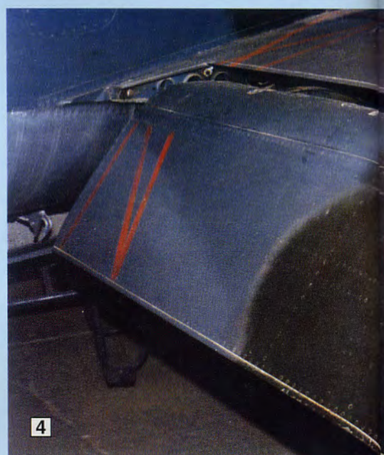
1. The nose wheel undercarriage of the G.91R showing the width of the nose wheel tyre and large heavy duty strut. 2. The port main undercarriage wheel again emphasising the size of the tyre and struts. 3. The G.91Rs canopy and ejector seat. The top of the cockpit entry ladder is just visible. 4. The G.91 flaps were large for short field landing capability.
