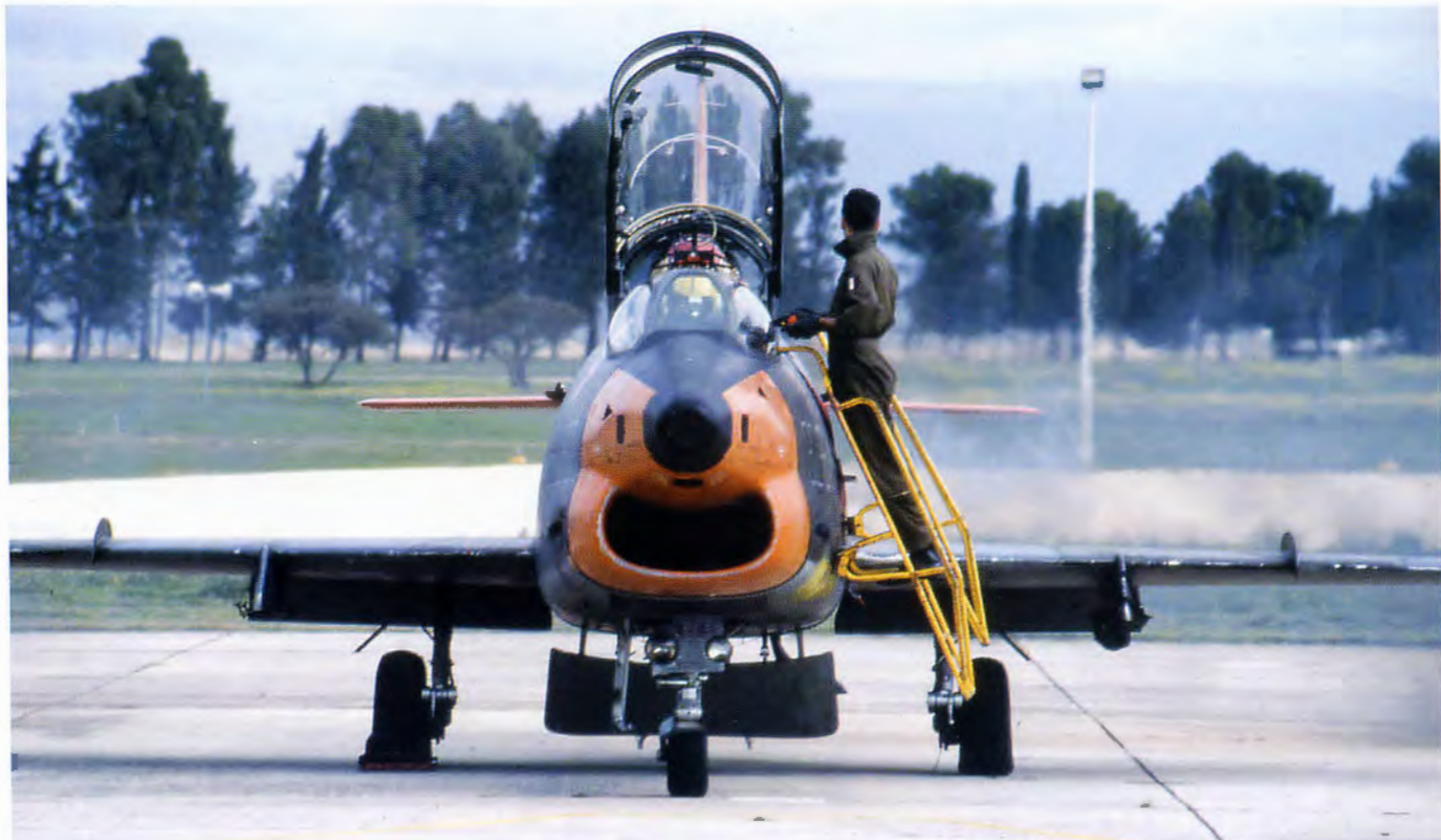
Interesting front view of a FIAT G.91T. Of note are the large airbrakes underneath the fuselage, here seen fully extended (Giuseppe Fassari)
