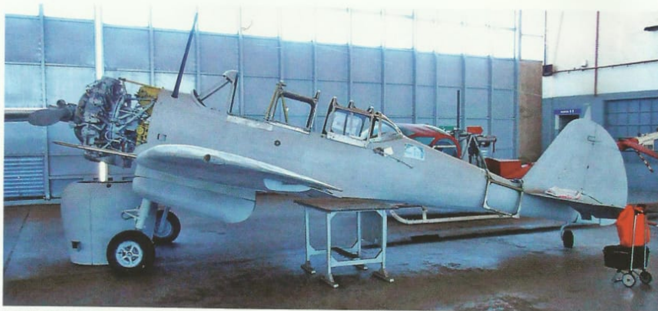
Now basically complete, the Falcon receives a coat of primer prior to final painting.
