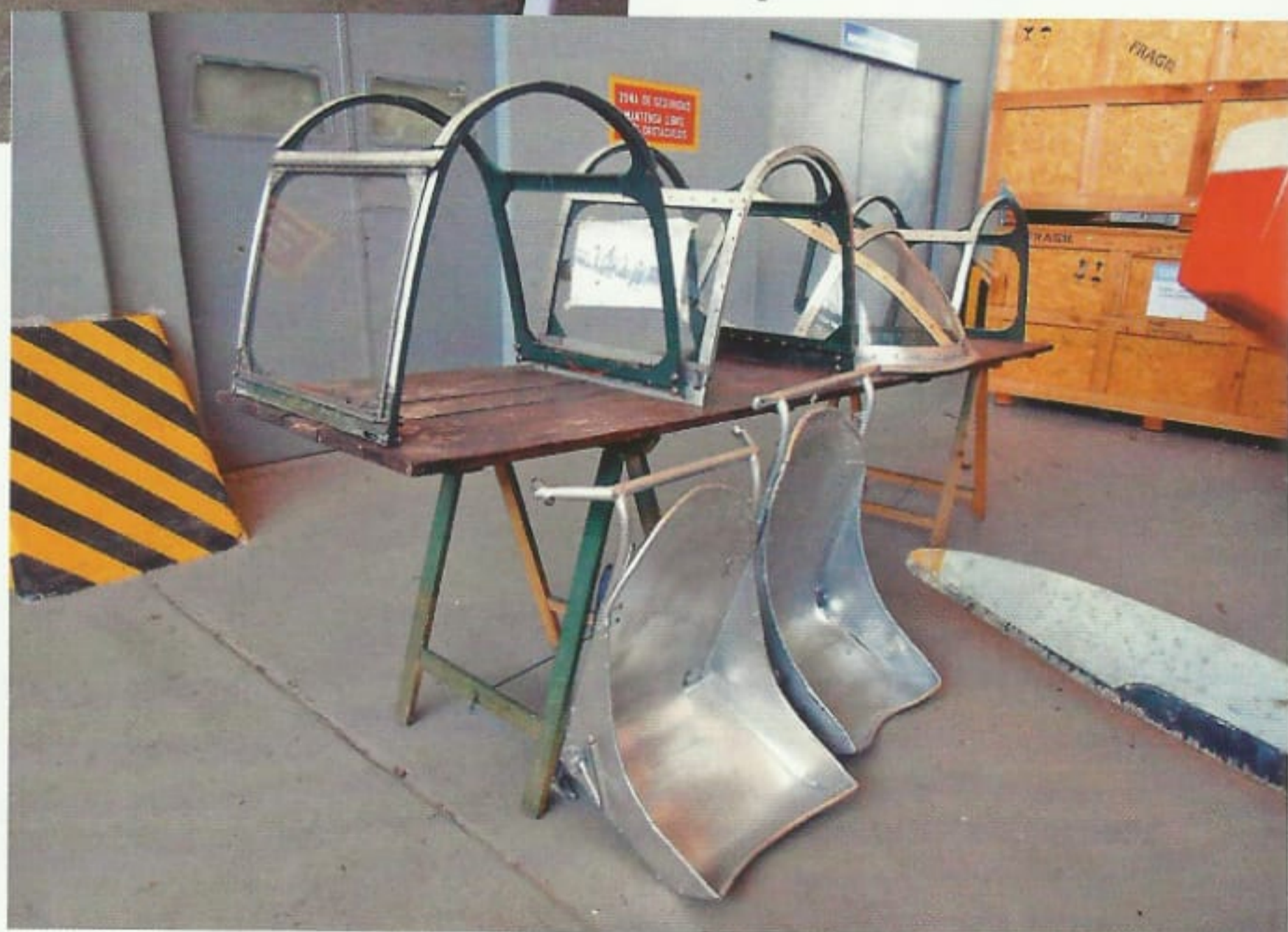
The canopy frames and seats had to be built from scratch.
