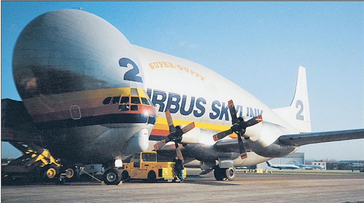
With its vast forward fuselage hinged to port, a Guppy 201 takes on a load of Airbus components.
