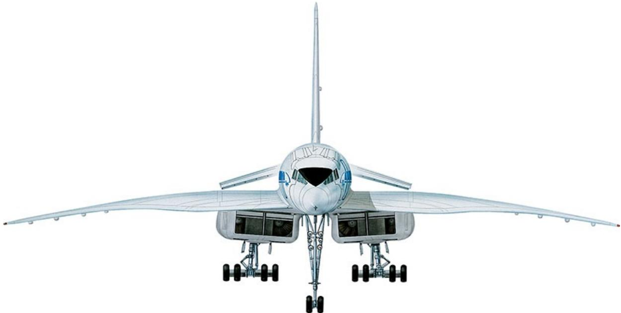
The Tu-144 prototype resembled Concorde, but was quite different in detail, while the production aircraft were far closer to the Western aircraft in design.
