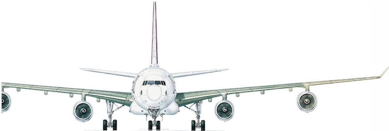
The wings of the A330 and A340 are remarkably similar, the A330 retaining the hardpoint for the outer engine's pylon.
