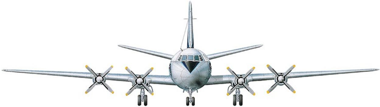
The Viscount's sharply dihedralled tailplanes and sloping nose profile were particularly evident from the front.
