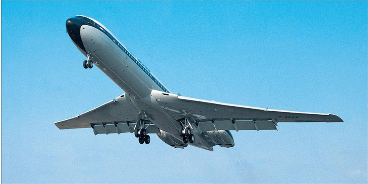
**The VC10's extensive high-lift devices were particularly evident on take-off.**
