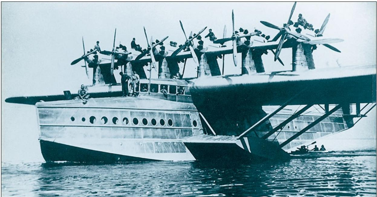
The Do X in its original form, with Jupiter radial engines. Although it flew successfully with this powerplant, it was underpowered for regular operations.
