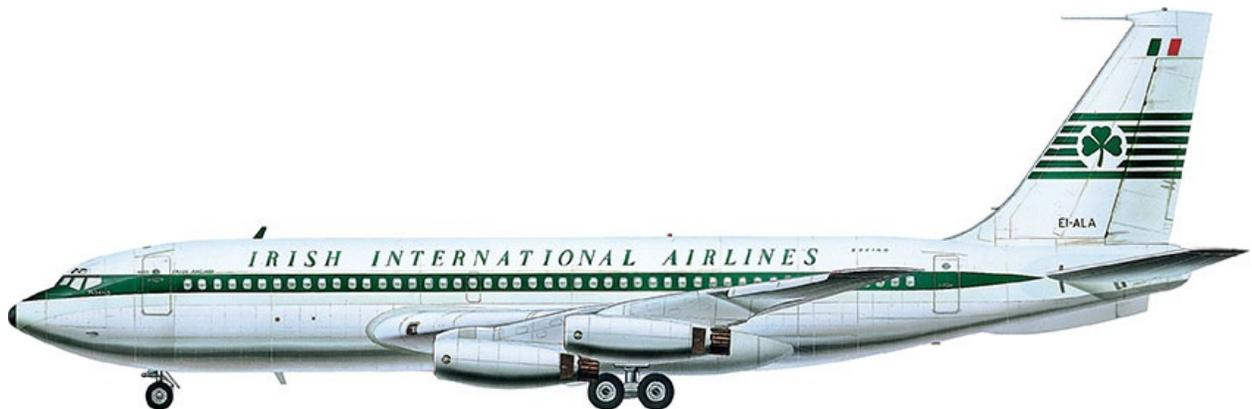
**Aer Lingus was among many airlines that operated the 720 from new. This is an early machine, with JT3C turbojet engines.**
