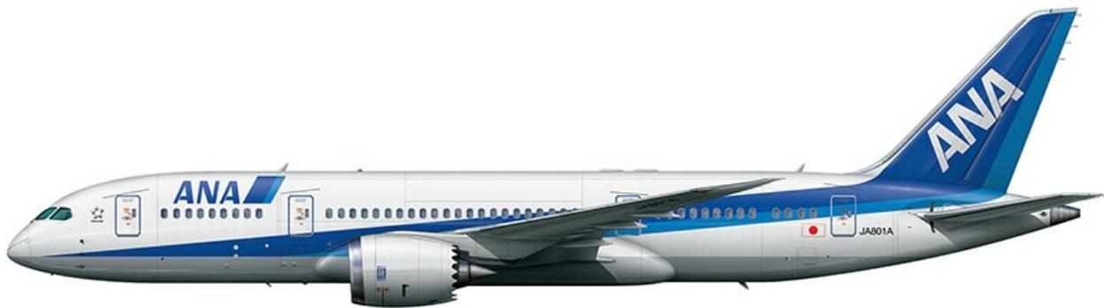
**All Nippon Airways were the first airliner to operate the Boeing 787-8, which first flew commercially in October 2011. The 787-8 is the base model of the 787 family, with a length of 57m (186ft) and a wingspan of 60m (197ft).**
