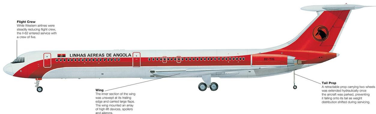
**Thanks to its more efficient engines and greater fuel capacity, the Il-62M offered a considerable**
