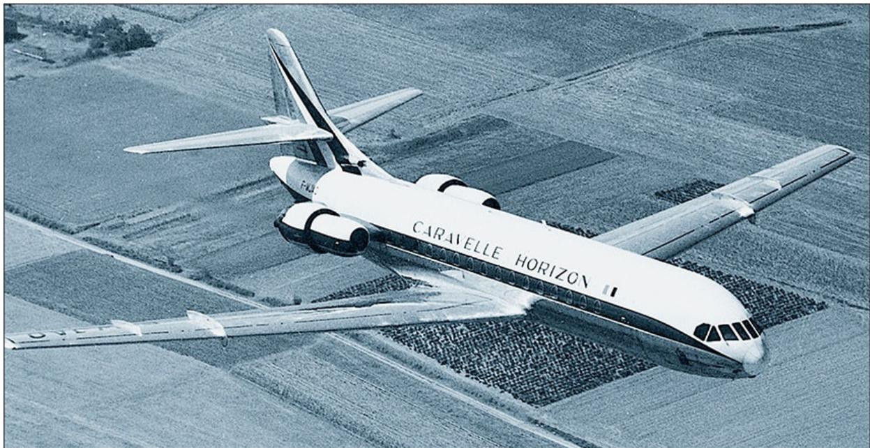
As well as CJ805 engines, the Caravelle Horizon featured wing and tailplane changes. Its cabin windows were raised to a higher position.
