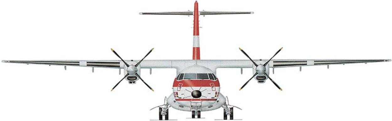
From the forward elevation the ATR's bulbous main undercarriage fairings are obvious. The four-bladed propellers are also evident.
