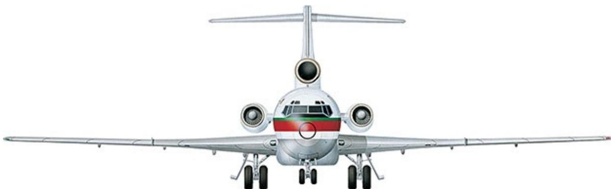
In another masterstroke Boeing used the upper fuselage of the 707, speeding design, standardizing flight decks and saving money on production tooling. The relatively wide cabin also allowed the 727 to seat passengers six abreast in
