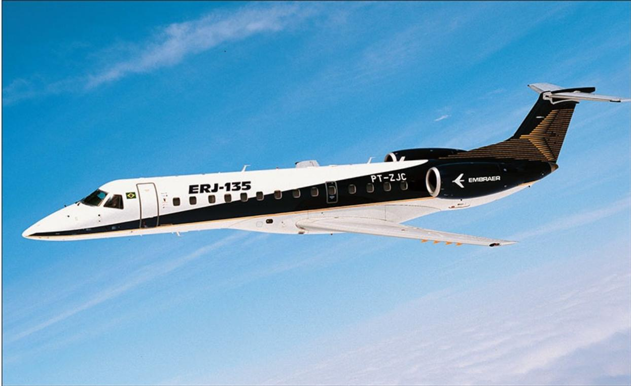
**PT-ZJC was the second ERJ-135 prototype. The model's forward fuselage was shortened compared to that of the ERJ145.**
