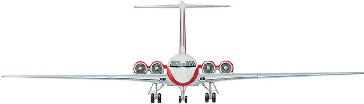
The VC10's engine nacelles were mounted in a 'spectacle' arrangement, but a short joining section separated those of the Il-62.
