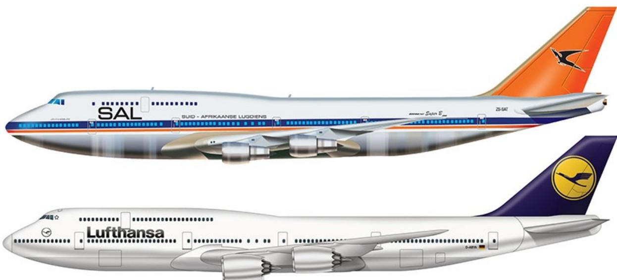
A stretched upper deck was the primary difference between the 747-300, here shown in South African Airways livery, and the 747-200, here shown in Lufthansa livery.
