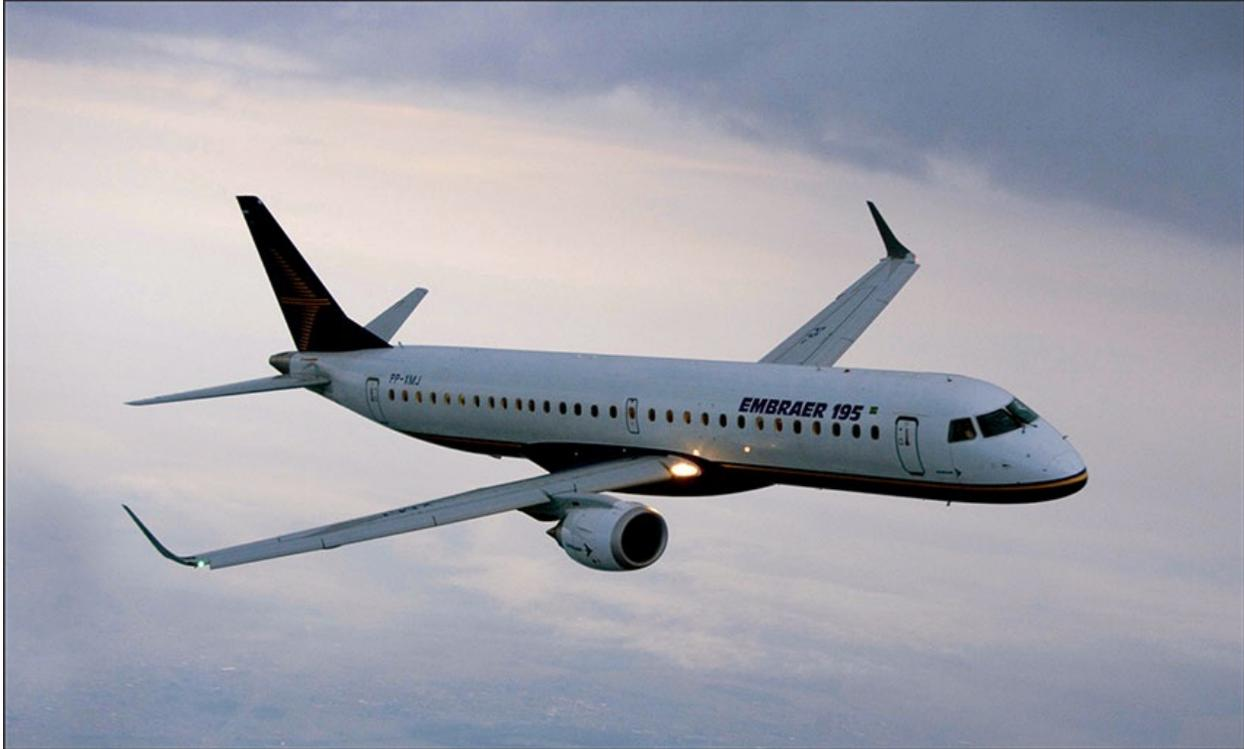
**The E195 is the longest member of the E-Jet family, featuring a new wing and revised tail section. This aircraft was the prototype.**
