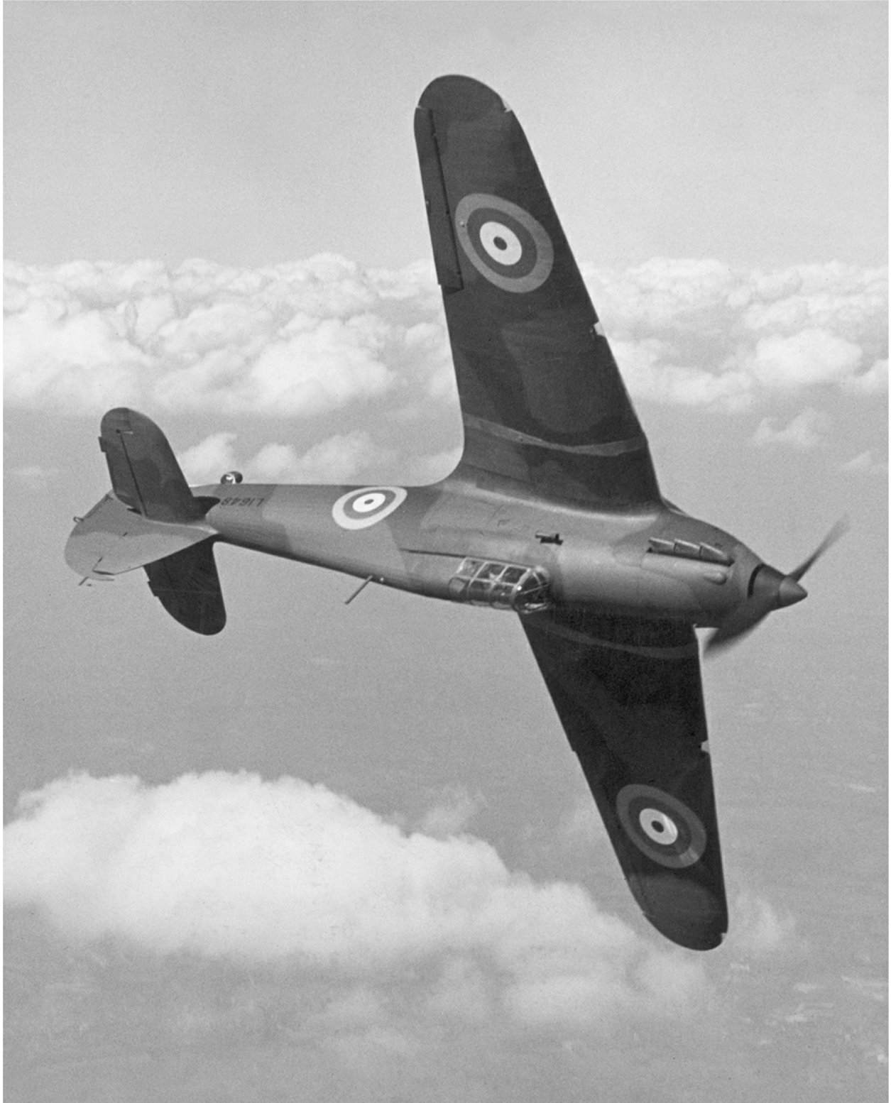
In 1940, the Hawker Hurricane Mk I formed the backbone of Fighter Command. The first monoplane fighter to enter service with the RAF, the type was powered by a 1,030hp Rolls-Royce Merlin engine and armed with eight Browning 0.303in machine guns. The type was involved in heavy fighting over France and Norway and 34 Hurricane-equipped squadrons were deployed during the Battle of Britain.
