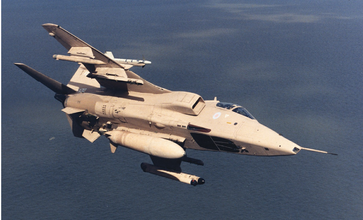
A SEPECAT Jaguar GR1A fitted with the self-defence suite carried during the Gulf War: over-wing mounted AIM-9L Sidewinder air-to-air missiles (AAM), a 1,200lt centre-line fuel tank, with an AN/ALQ 101-10 electronic countermeasures (ECM) pod and a Phimat chaff and flare dispenser pod on the outboard pylons. This configuration leaves the inboard under-wing pylons free for weapons. (BAe Heritage)
