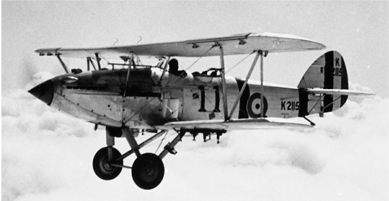
The early 1930s saw streamlined and more powerful aircraft entering service. The Hawker Hart, powered by a Rolls-Royce Kestrel engine, could outperform most fighters of the day. Apart from being the standard day-bomber used by the RAF home squadrons, the type also equipped overseas units, including 11 Squadron (here), based at Risalpur in northwest India. (Flintham)
