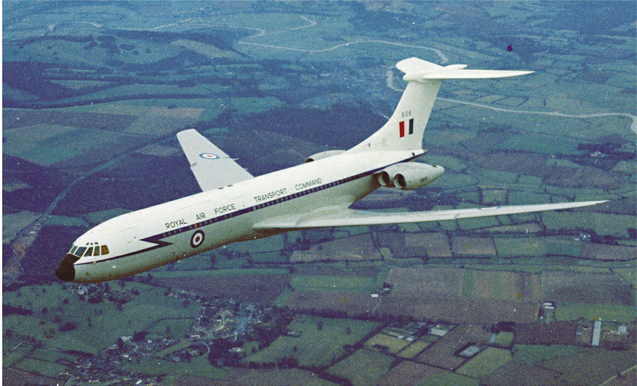
The Vickers VC10 C1 entered service with 10 Squadron at RAF Fairford in 1966. The military version of the aircraft was based on the fuselage of the civilian airliner, but was fitted with the more powerful Rolls-Royce Conway 301 engines and the improved fuel capacity of the Super VC10. (RAFM)
