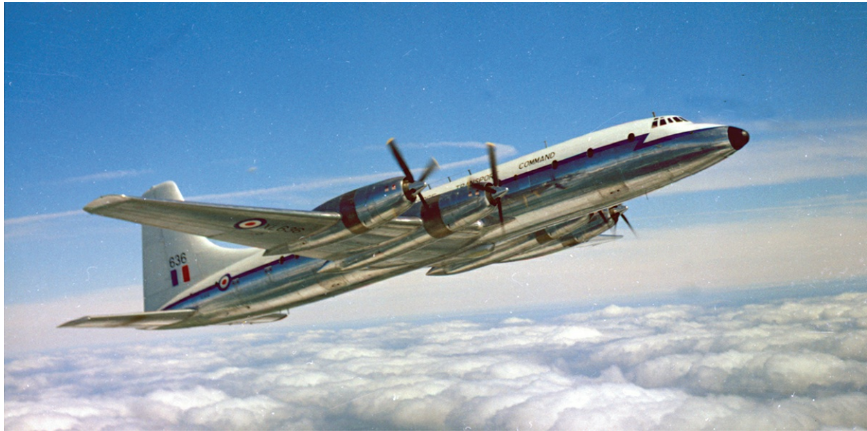
The Bristol Britannia entered service with 99 and 511 Squadrons at RAF Lyneham in 1959. Capable of carrying 113 passengers or 37,400lb of freight, the type served as the strategic transport aircraft supplying British military interests across the globe. (RAFM)
