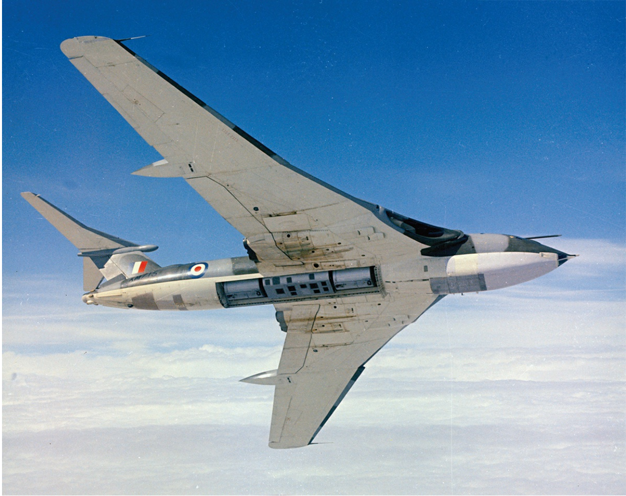
A Victor B(SR)2 strategic reconnaissance aircraft of 543 Squadron banks away to display the reconnaissance equipment. Fitted inside the bomb bay in three sections, the equipment could be varied to suit the task and could include a F49 vertical, F96 oblique or night-capable F89 camera, photo-flash flares, air sampling equipment and/or extra fuel tanks. (RAFM)
