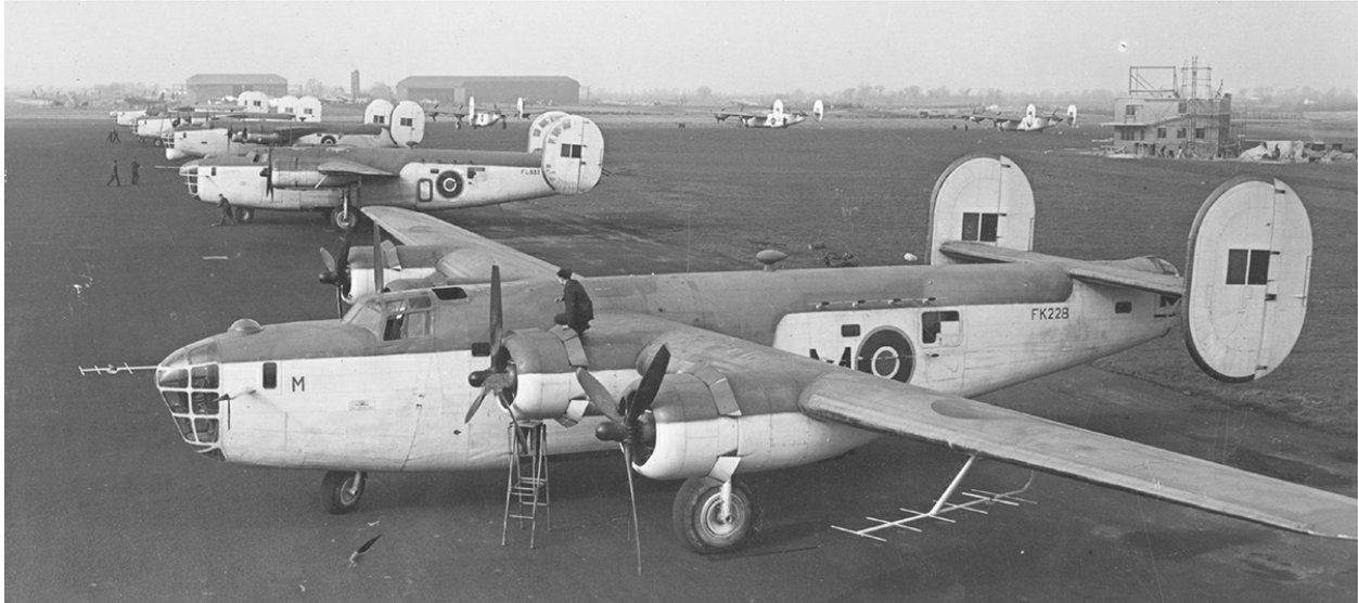
Consolidated B-24D Liberator IIIs of 120 Squadron. The Yagi aerals for the forward-looking ASV radar are clearly visible under the wing. With an operational range of some 2,400 miles (as compared to 1,300 miles for a Sunderland), the Liberator gave Coastal Command a quantum leap in its anti-submarine capability. (RAFM)
