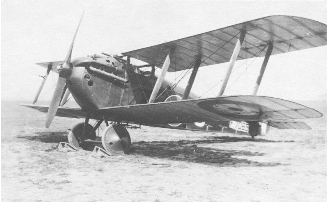
The distinctive 'backward stagger' of the wings of the Sopwith 5F1 Dolphin is clearly visible in this view. The type saw service in France with 19, 23, 79, 87 and 90 Squadrons.
