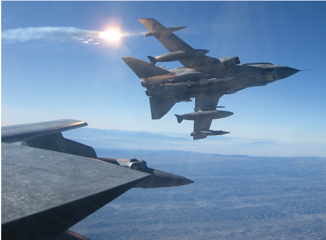
An infra-red decoy flare is ejected from the BOZ-107 pod on a Tornado GR4 over Afghanistan. The aircraft is also armed with 500lb Paveway IV Laser-Guided Bombs (LGB) and MBDA Brimstone Dual-Mode Seeker (DMS) missiles. (Stradling)
