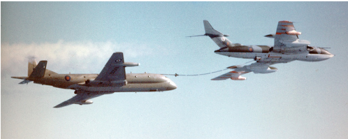
When the Falklands Campaign was launched an air-to-air (AAR) capability had to be hastily introduced for the Nimrod MR2 fleet, to enable the aircraft to fly long-range patrols from Ascension Island. Here a Nimrod MR2P refuels over the South Atlantic from a Victor K2 of 57 Squadron. (120 Squadron Archive)
