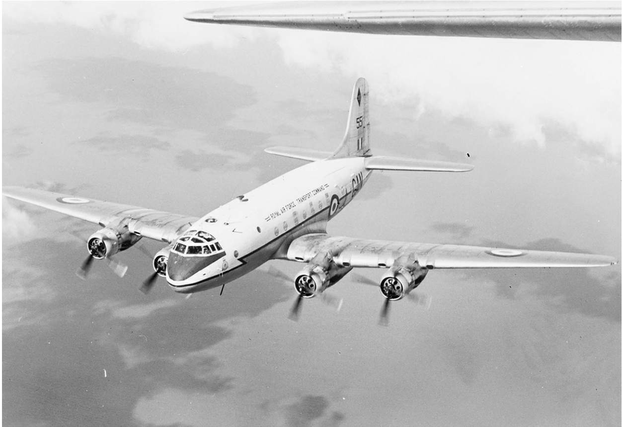
A Handley Page Hastings C1 of 70 Squadron. The type formed the backbone of RAF Transport Command equipping eleven squadrons in the UK and Europe, and a further two overseas. A small number of aircraft designated Hastings Met1 were operated by 202 Squadron for meteorological reconnaissance flights. (© IWM 27470)
