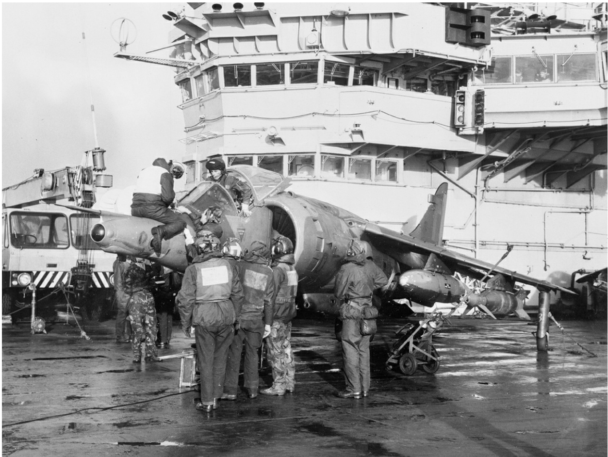
A Harrier GR3 from 1 Squadron prepares for a sortie aboard HMS Hermes . The aircraft is loaded with a 1,000lb Paveway II Laser Guided Bomb (LGB). These weapons were used briefly at the end of the campaign: for the majority of ground-attack missions the Harriers were armed with 1,000lb high-explosive (HE) bombs or BL755 Cluster Bomb Units (CBUs). (RN Official Photographer/IWM/Getty)
