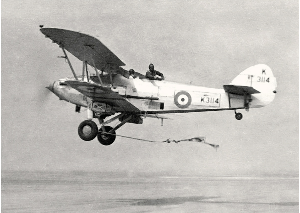
In the days before reliable Radio/Telecommunication (R/T) equipment could be carried in aircraft, the main method of communication between ground forces and aircraft was by written message. Here a Hawker Audax of 208 Squadron picks up a message in 1936. (Pitchfork)
