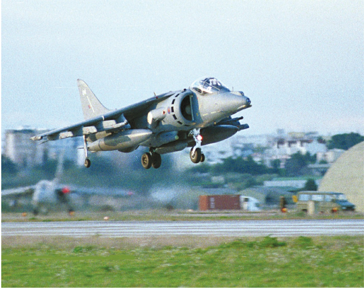
A BAe Harrier GR7 returns to Gioia del Colle after a mission over the Balkans in the late 1990s. Equipped with forward looking infra-red (FLIR) sensors and a cockpit compatible with night vision goggles (NVG), this version of the aircraft introduced a night combat capability to the RAF Harrier force. (Crown Copyright)
