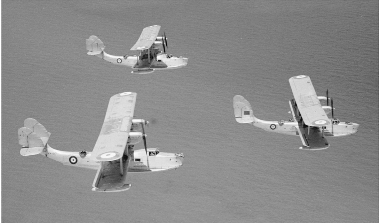
A formation of Supermarine Scapa flying boats of 204 Squadron, based at Alexandria in 1936. The aircraft was originally known as the Southampton IV and was powered by two Rolls-Royce Kestrel engines. (Charles E. Brown/RAF Museum/Getty)
