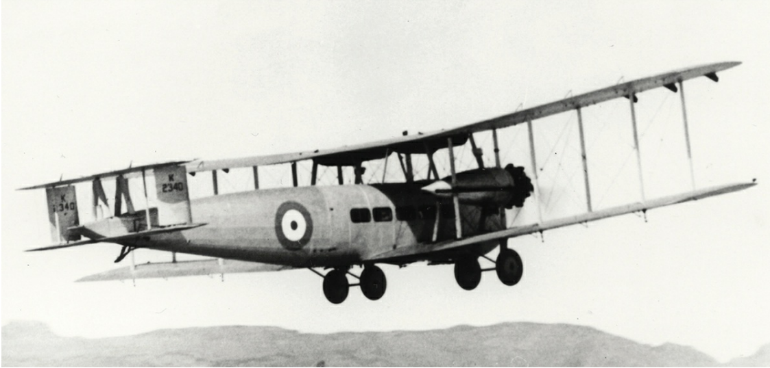
A Vickers Victoria V over northern India. Eight of these aircraft, from 70 and 216 Squadrons, carried out the evacuation of nearly 600 British and other nationals from Kabul during the winter of 1928/29. Powered by two Napier Lion XI engines, the aircraft could carry 22 passengers. It was superseded in service by the Vickers Valentia, although many were, in fact, re-engined Victorias. (Flintham)
