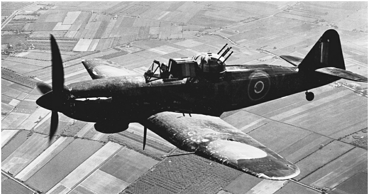
A Boulton Paul Defiant of 264 Squadron. During the early days of World War II, the type proved to be a failure as a day fighter, but was used successfully as a night fighter, eventually equipping 13 squadrons. (Corbis/Getty)
