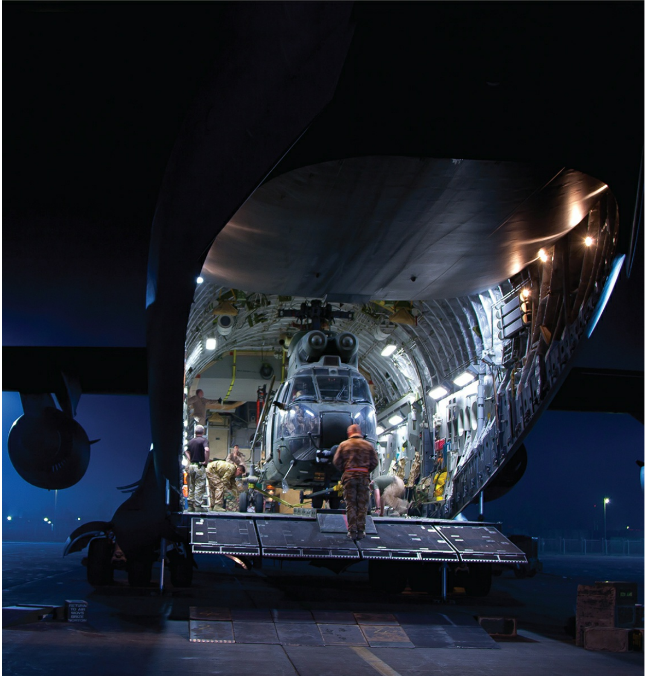
A Westland-Aerospatiale Puma HC1 loaded in the hold of a Boeing Globemaster III, ready to be transported to Iraq. The aircraft can carry two Pumas and once delivered, the helicopters could be readied for flight within four hours. (Knight)
