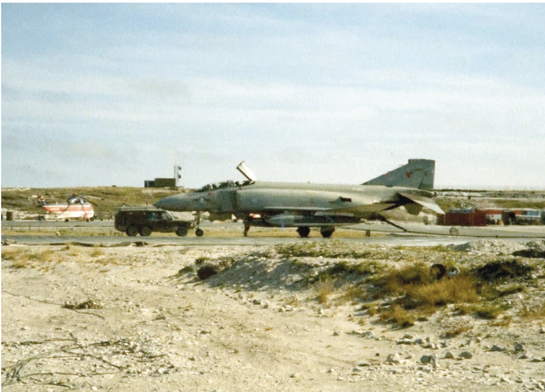
A Phantom FGR2 of 23 Squadron at Stanley airstrip in the Falklands. The runway had to be extended with AM2 aluminium matting to allow Phantom operations, but even so the type needed to use the Rotary Hydraulic Arrestor Gear (RHAG) to stop after landing. The lowered arrestor hook is clearly visible. (Peter Butt/Wikimedia/Public Domain)
