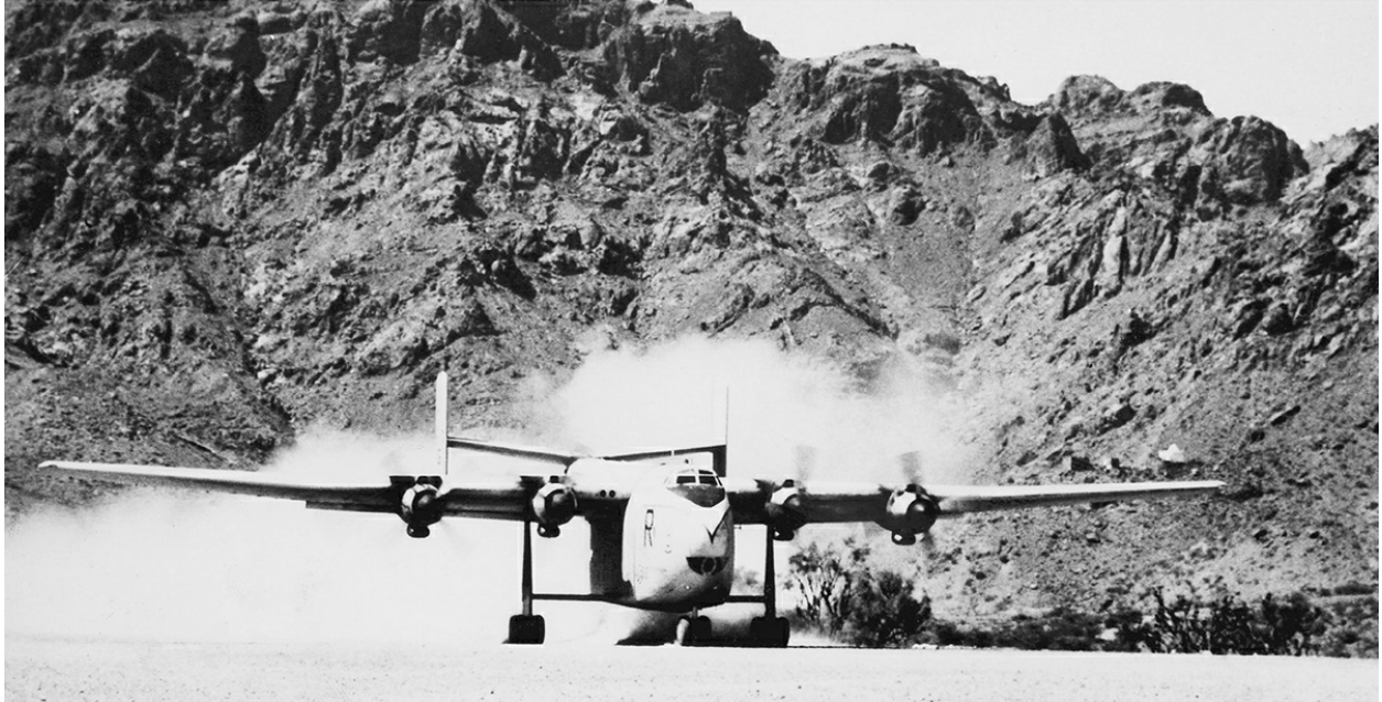
A Blackburn Beverley of 84 Squadron lands on a desert strip 'up country' in Aden. The fuselage had a capacity of some 22 tons and a compartment in the tail boom could accommodate up to 94 passengers. The Beverley could also operate from rough airstrips as short as 2,550ft. (Flintham)
