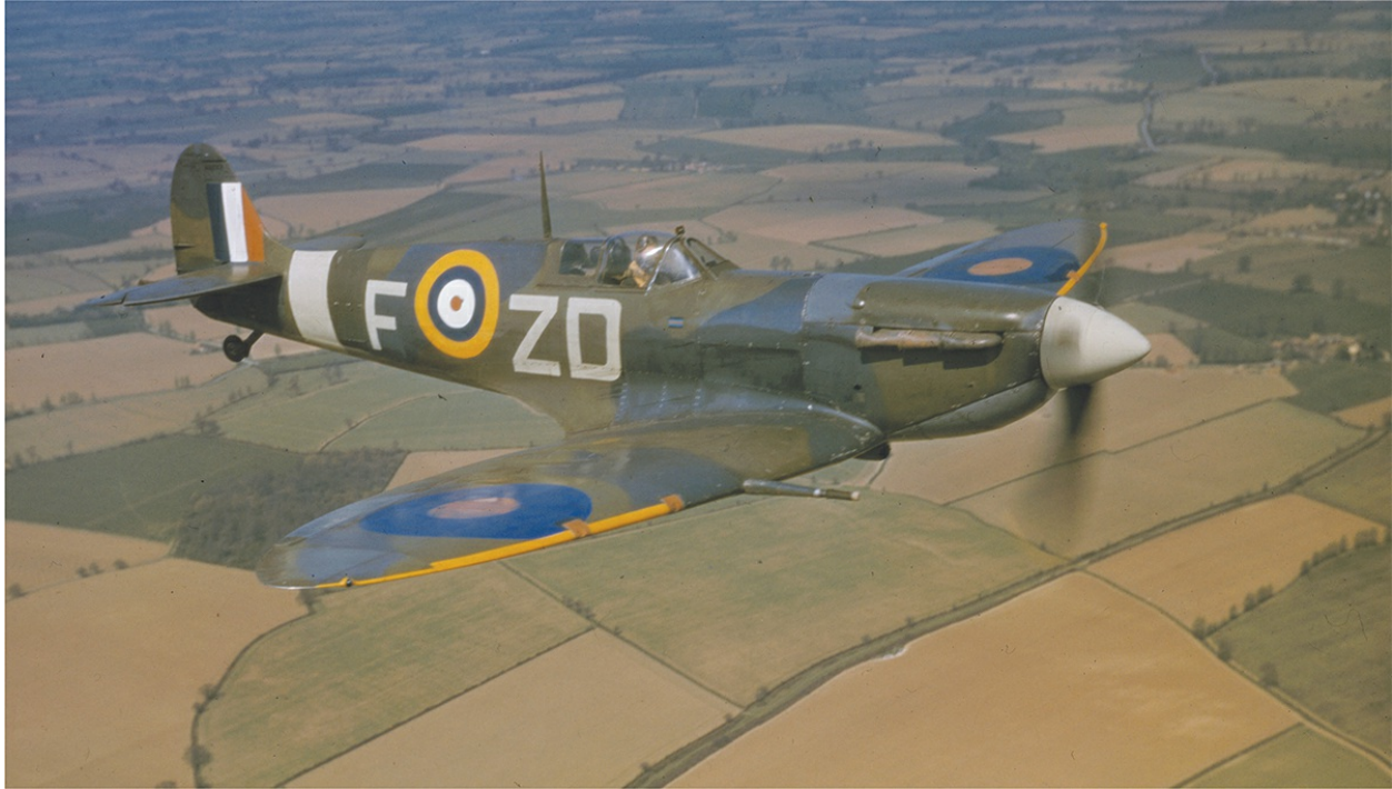
A Spitfire Mk VB of 222 Squadron based at North Weald. Deliveries of this version began in early 1941 and the improvements introduced included a 1,440hp Rolls-Royce Merlin 45 series engine and improved armament comprising two 20mm cannon and four .303in Browning machine guns.
