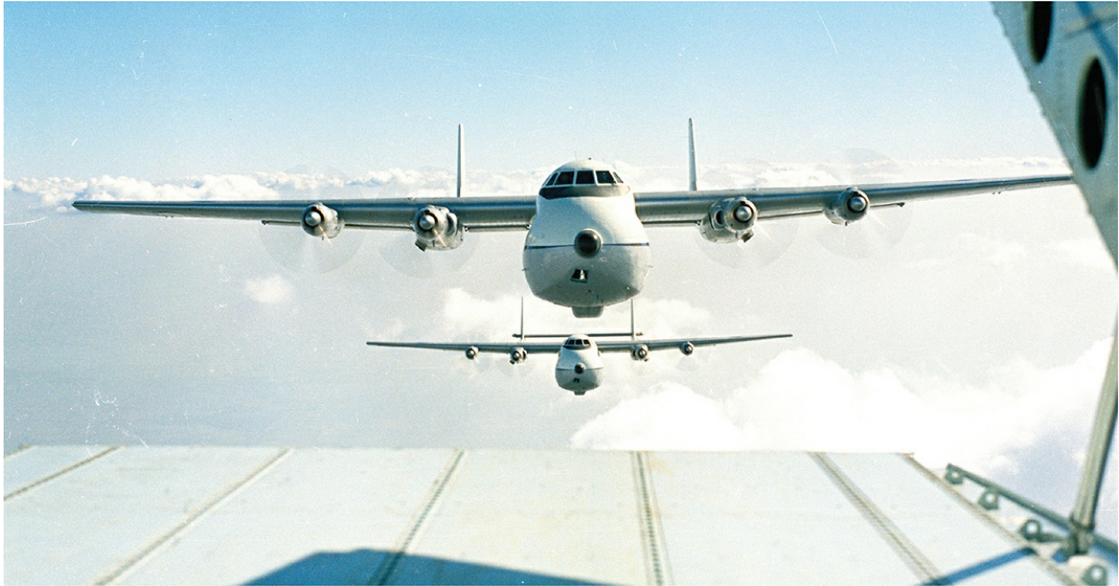
The Armstrong Whitworth Argosy saw service in the UK, Cyprus, Aden and the Far East. The cockpit was above the spacious cargo hold and loads could be air-dropped through the 'crocodile jaw' doors at the rear of the aircraft. (RAFM)
