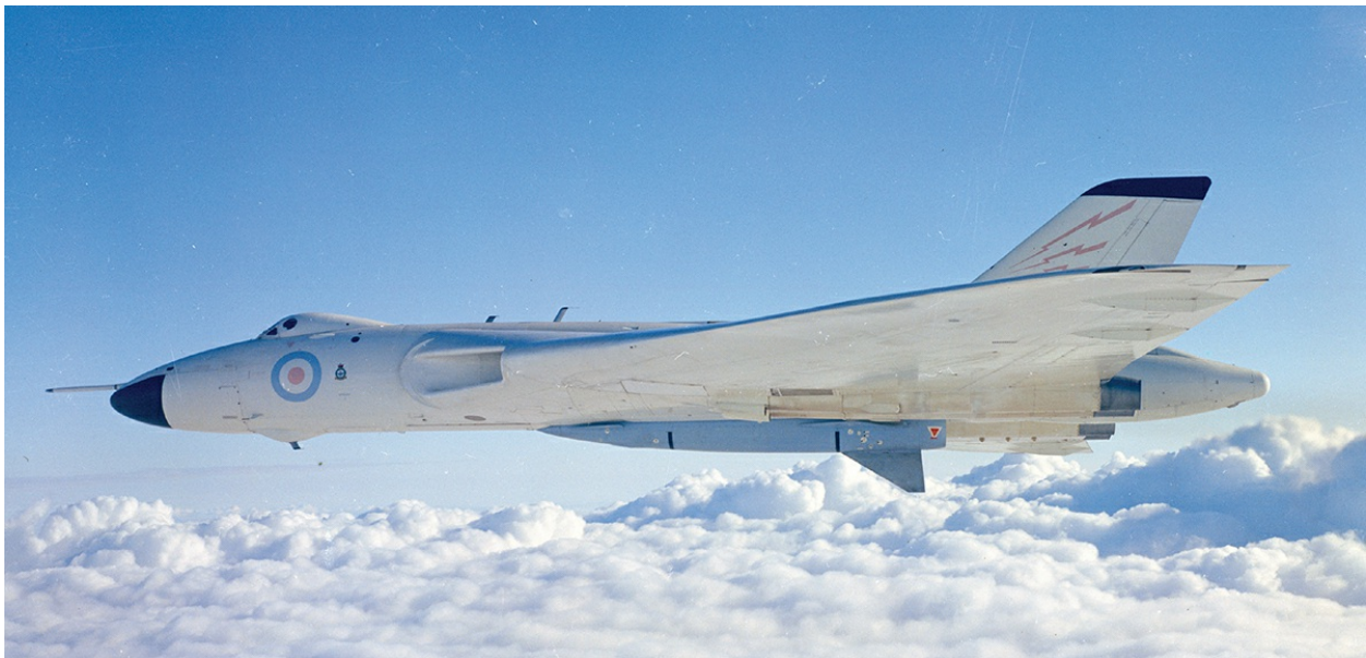
An Avro Vulcan B2A of 617 Squadron armed with an Avro Blue Steel stand-off missile. Between 1962 and 1966 the Vulcan and Victor aircraft of Bomber Command were equipped with the Blue Steel missile to provide Britain's independent nuclear deterrent. (RAFM)
