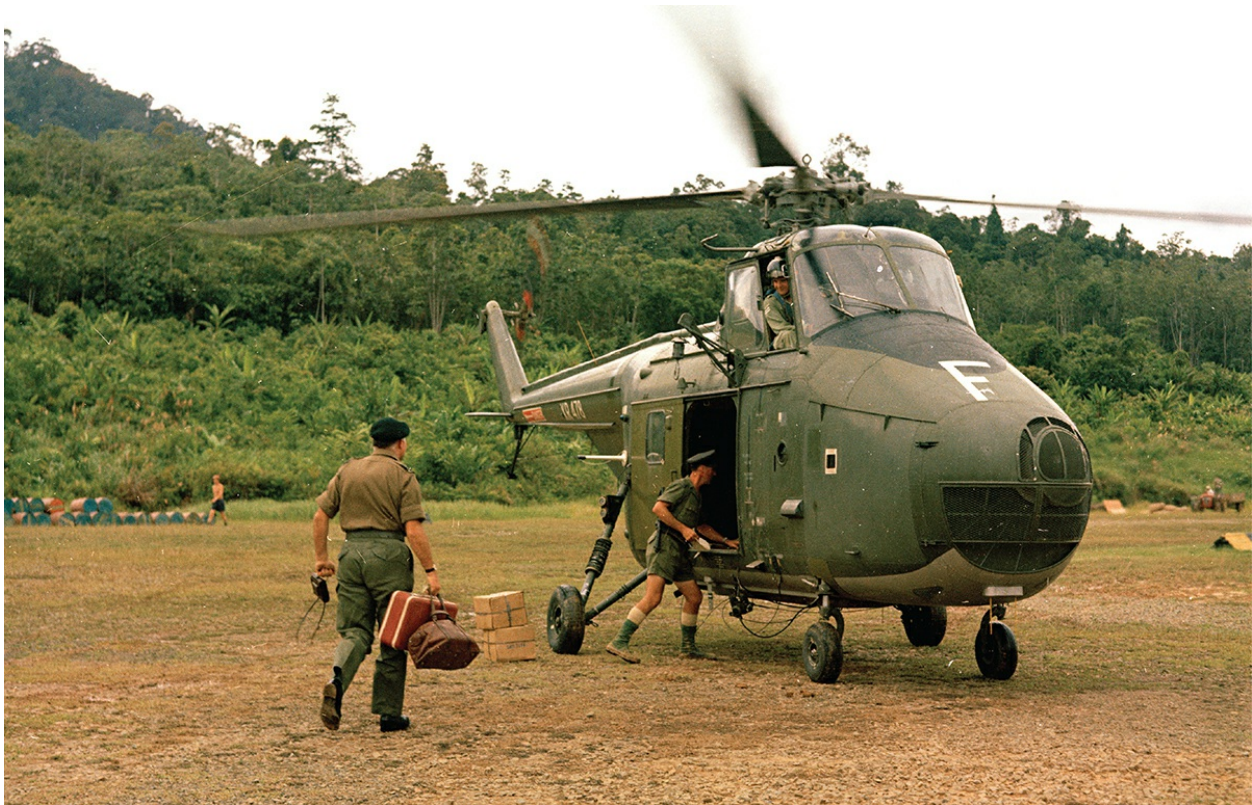
A Westland Whirlwind HAR10 of 110 Squadron in Borneo, where the campaign proved the true value of the helicopter in RAF service. Unlike earlier piston-engined types, the HAR10 was powered by a Bristol Siddeley (Rolls-Royce) Gnome gas turbine engine. (RAFM)
