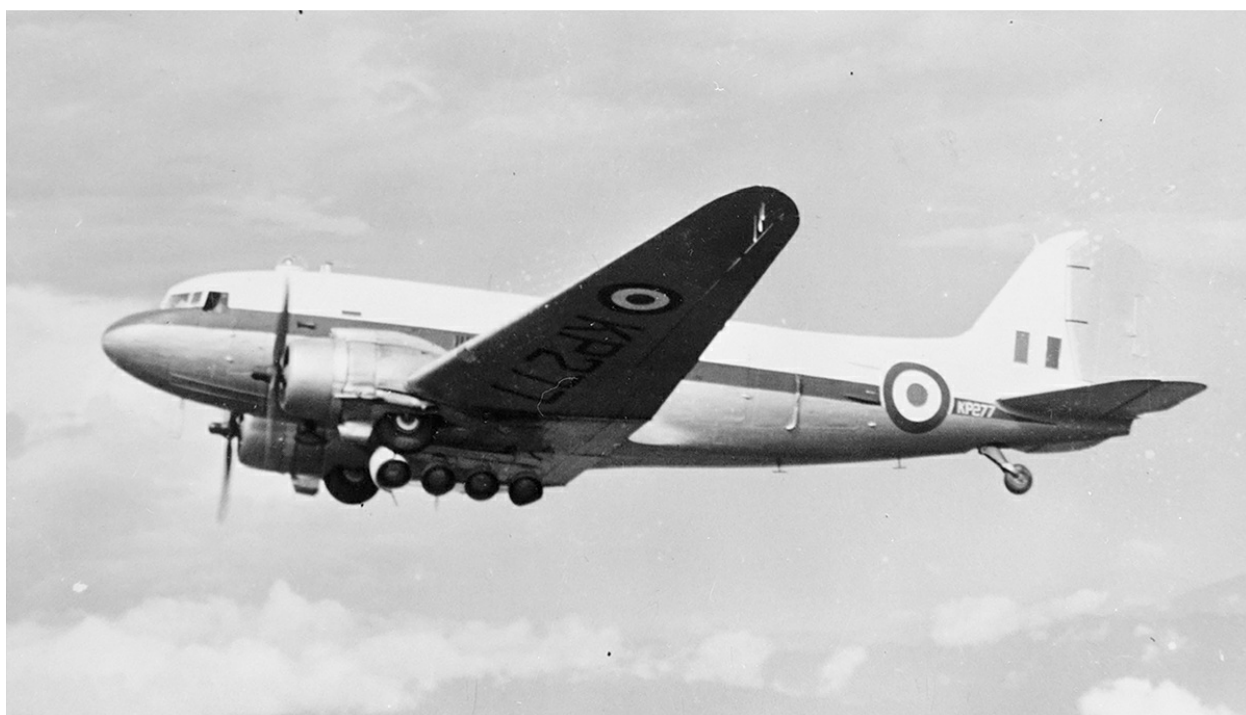
An RAF Douglas C-47 (DC-3) Dakota equipped with loudspeakers fitted to the underside of the fuselage. 'Sky shouter' aircraft, including the Auster AOP and the Hunting Percival Pembroke, were used over rebel areas in Malaya, Kenya and Oman to broadcast messages encouraging insurgents to surrender. (© IWM MAL 80)
