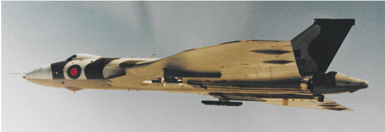
An Avro Vulcan armed with an AGM-45 Shrike Anti-Radiation Missile (ARM) mounted under the left wing and a Westinghouse AN-ALQ101 Electronic Countermeasures (ECM) pod under the right wing.
