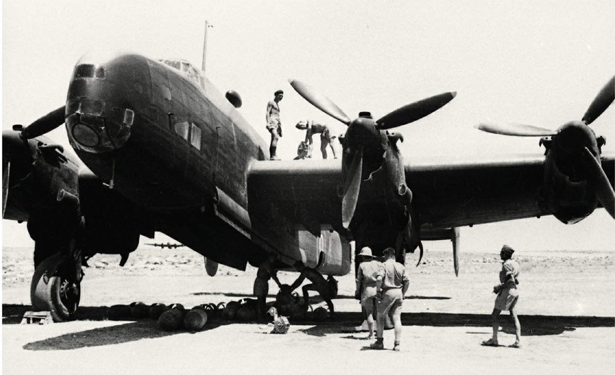
A Handley Page Halifax II Series I Special in the Middle East. This version of the aircraft had the original high-drag nose turret replaced with a fairing. The type was used in the Mediterranean and Balkans both as a heavy bomber (shown) and also as a special duties aircraft; in the latter role the type was used in support of the Special Operations Executive (SOE). (Flintham)
