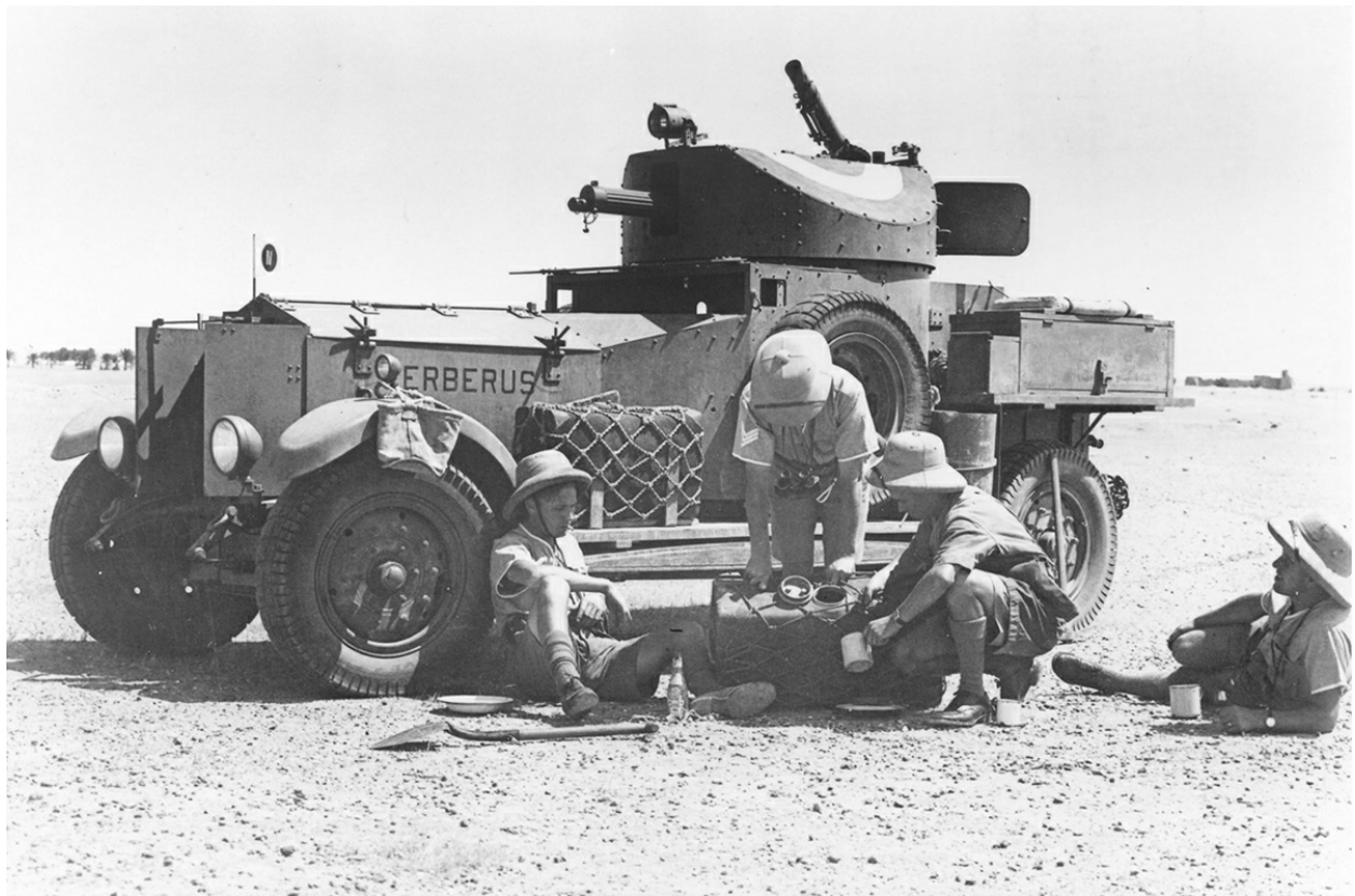
The crew of a Rolls-Royce 1920 Pattern Mk1 armoured car relaxing in the Iraq desert. The armoured car companies were an integral part of the system of Air Control in Palestine, Transjordan and Iraq. The vehicle was built using a Silver Ghost chassis, and was armed with a water-cooled Vickers .303in machine gun. The type remained in service long into World War II. (Pitchfork)
