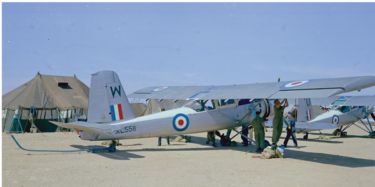
A Scottish Aviation Pioneer CC1 required a run of only 225ft for take-off, making it ideal for counter-insurgency work in Malaya where it was flown by 267 Squadron (re-numbered 209 Squadron) and later by 78 Squadron in Aden. (© IWM RAF-T1710)
