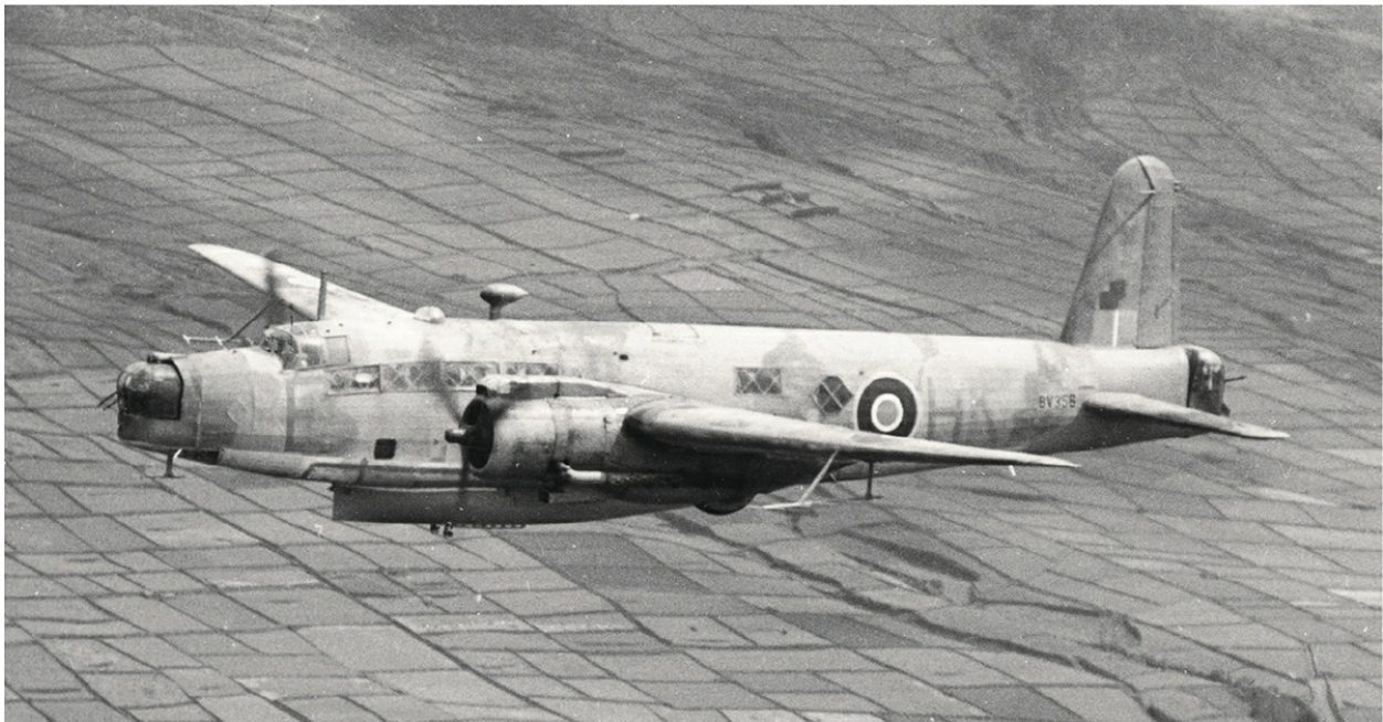
A Vickers Warwick I of 269 Squadron carrying a lifeboat under the fuselage. Some 350 of these aircraft, which was originally designed as a replacement for the Wellington, were used instead for Air
