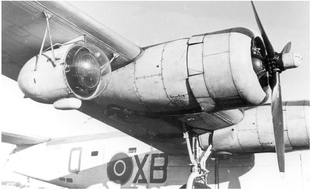
A Leigh Light mounted under the wing of a Liberator GR VI of 224 Squadron. In early 1944, the unit was based at Milltown, on the Moray Firth, Scotland to counter U-boats operating from bases in Denmark and Norway. (Pitchfork)
