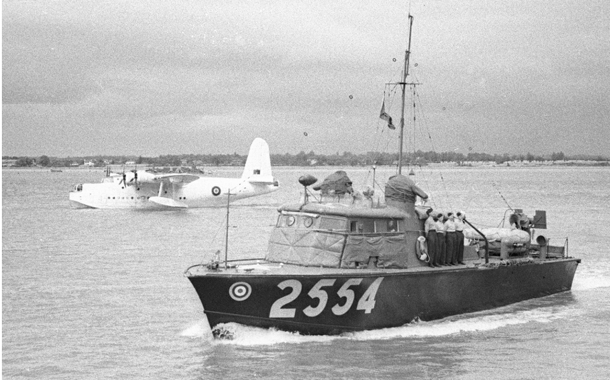
A High Speed Launch (HSL) Type 3; a total of 69 were built and used by the Air Sea Rescue service from late 1942. Powered by three 500hp Napier Sea Lion petrol engines, the 68ft vessel was capable of up to 28kt. (Charles E. Brown/RAF Museum/Getty)
