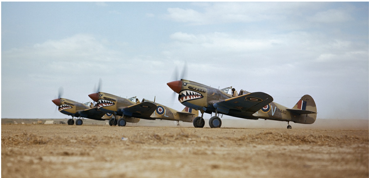
Curtiss P-40K Kittyhawk IIIs of 112 Squadron in North Africa. This version of the aircraft was fitted with the 1,600hp Allison V-1710 engine rather than the 1,040hp engine used for the Tomahawk. Eventually, the Kittyhawk equipped five RAF squadrons in the Middle East, as well as one RAAF and five SAAF units in the theatre. (© IWM TR 975)
