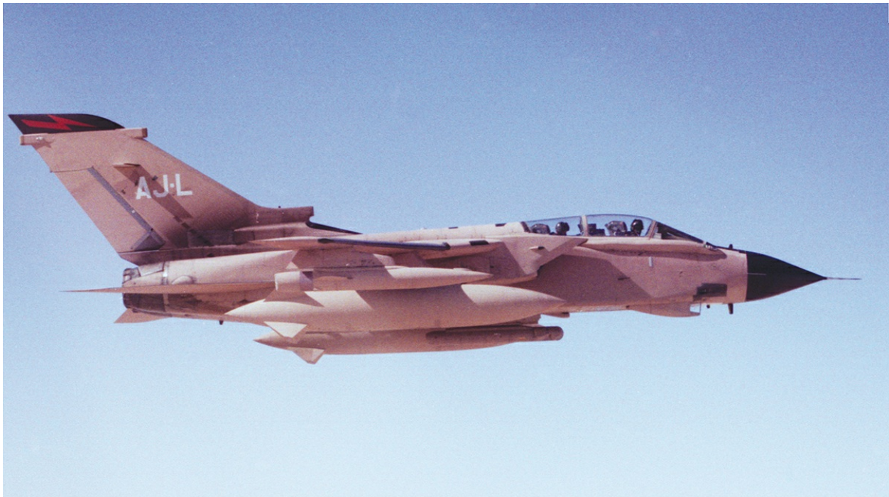
A Dhahran-based Tornado GR1, equipped with a Ferranti-manufactured Thermal Imaging Airborne Laser Designator (TIALD) pod, on patrol in the No Fly Zone (NFZ) over Southern Iraq in late 1992. The aircraft also carries 2,250-litre under-wing fuel tanks and the BOZ-107 chaff and flare dispenser.
