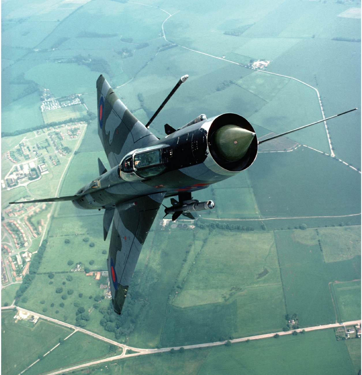
A Lightning F6 of 5 Squadron armed with two BAe Red Top infra-red seeking air-to-air-missiles (AAM). The last units equipped with this British-built fighter were 5 and 11 Squadrons based at RAF Binbrook. In 1988, both were re-equipped with the Panavia Tornado F3. (Crown Copyright)
