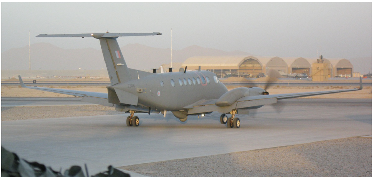
A Raytheon (Beechcraft) Shadow R1 of 14 Squadron at Kandahar. Equipped with a Hughes Wescam MX-15 electro-optical/infra-red sensor and an electronic surveillance suite, the Shadow provided ISTAR for army units.
