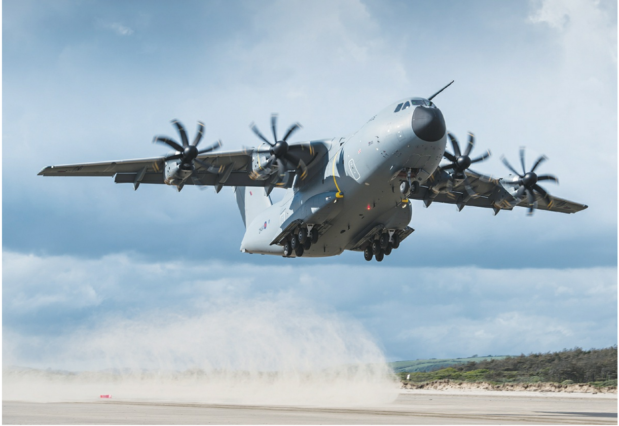
The Airbus A-400M Atlas which will replace the Lockheed C-130 Hercules in RAF service. The aircraft can carry a larger load than a Hercules, and is also capable of operating into a smaller airstrip than the Boeing C-17 Globemaster. (Crown Copyright)
