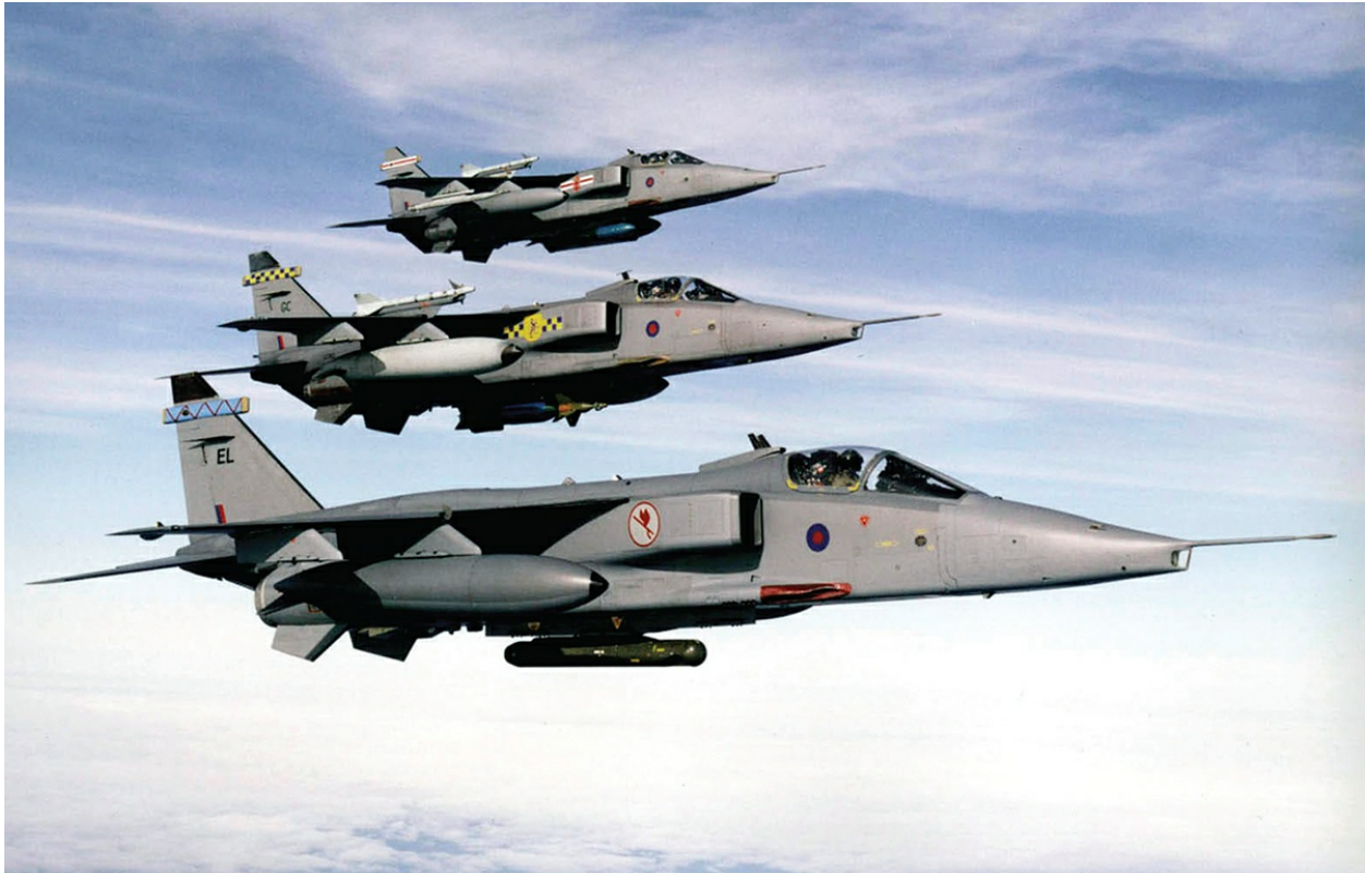
Jaguars of 6, 54 and 41 Squadrons of the Coltishall Wing. The aircraft in the foreground is a GR1B carrying a Ferranti TIALD pod. During operations over Bosnia in the autumn of 1995, TIALD-equipped Jaguars designated targets for Harrier GR7s to attack with LGBs. (Crown Copyright)
