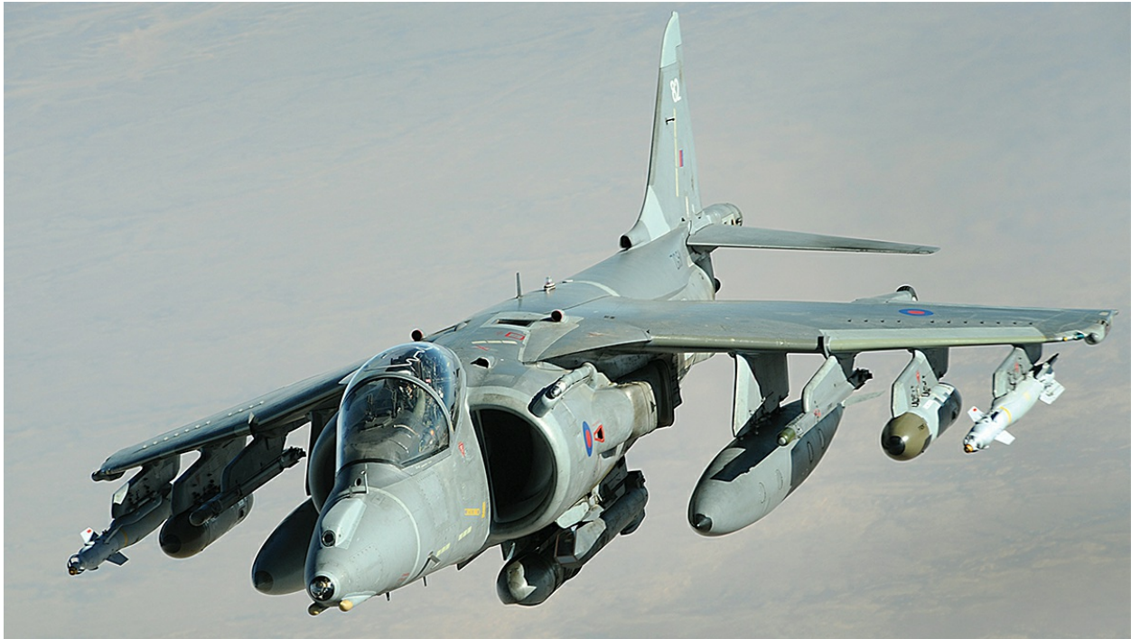
The BAe Harrier GR9, which superseded the GR7A in 2007, had many improvements over its predecessor including the capability to use the Hughes/Raytheon AGM-65 Maverick air-to-ground missile and the Lockheed Martin Sniper targeting pod. (USMC)
