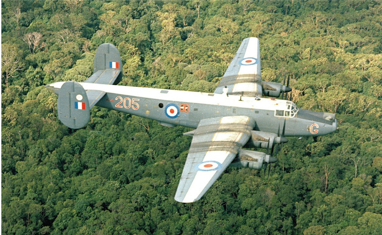
A Shackleton MR2C of 205 Squadron at low level over the Borneo jungle. Unique to 205 Squadron, the aircraft were MR2 airframes updated with the navigation and attack systems of the Shackleton MR3. (RAFM)
