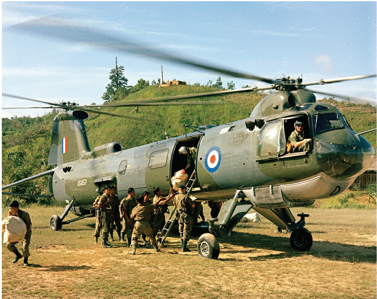
A Bristol/Westland Belvedere HC1 of 66 Squadron delivers supplies to a Gurkha detachment in Borneo. The Belvedere was powered by two Napier Gazelle NGa2 gas turbines and could carry 18 fully armed troops or an underslung load of up to 5,250lbs. (RAFM)
