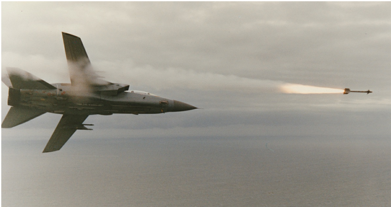
An AIM-9 Sidewinder AAM is fired from a Panavia Tornado F3 during a training sortie. Like the Phantom which it replaced, the Tornado F3 was armed with four Sidewinder and four Skyflash missiles. By 1989, six front-line air-defence squadrons had been equipped with the type. (Crown Copyright)
