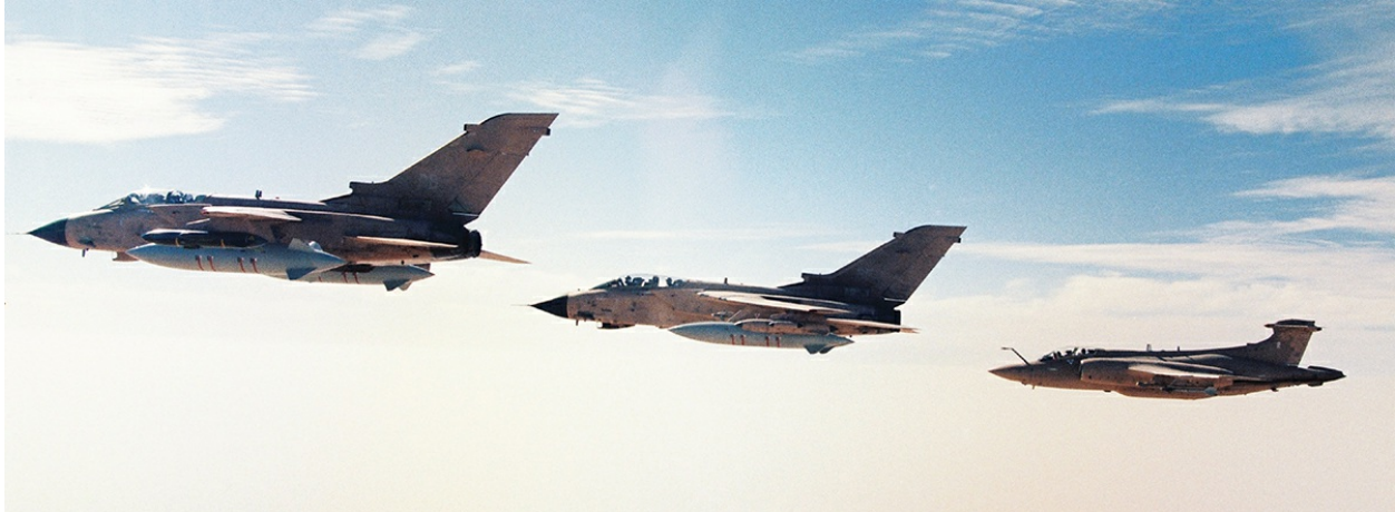
A typical interdiction formation as used in the latter half of the Gulf War: two Tornado GR1s armed with laser-guided bombs (LGBs) are accompanied by a BAe Buccaneer S2B equipped with an AN/AVQ-23E Pave Spike, electro-optical laser designator targeting pod. (Glover)
