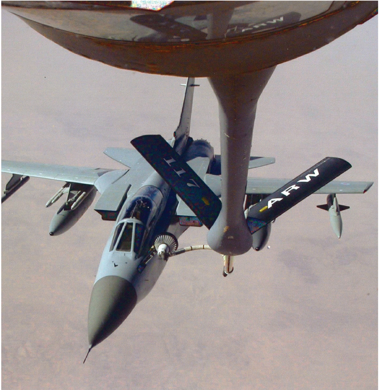
A Tornado F3 in its operational weapons fit refuels from a USAF Boeing KC-135 Stratotanker during Operation Telic . The aircraft is equipped with a Towed Radar Decoy (TRD) on the port outer wing pylon and a Phimat chaff dispenser on the right wing. Four MBDA AIM-132 Advanced Short Range AAMs (ASRAAMs) are carried on the inner stub pylons. (43 Squadron Archive)
