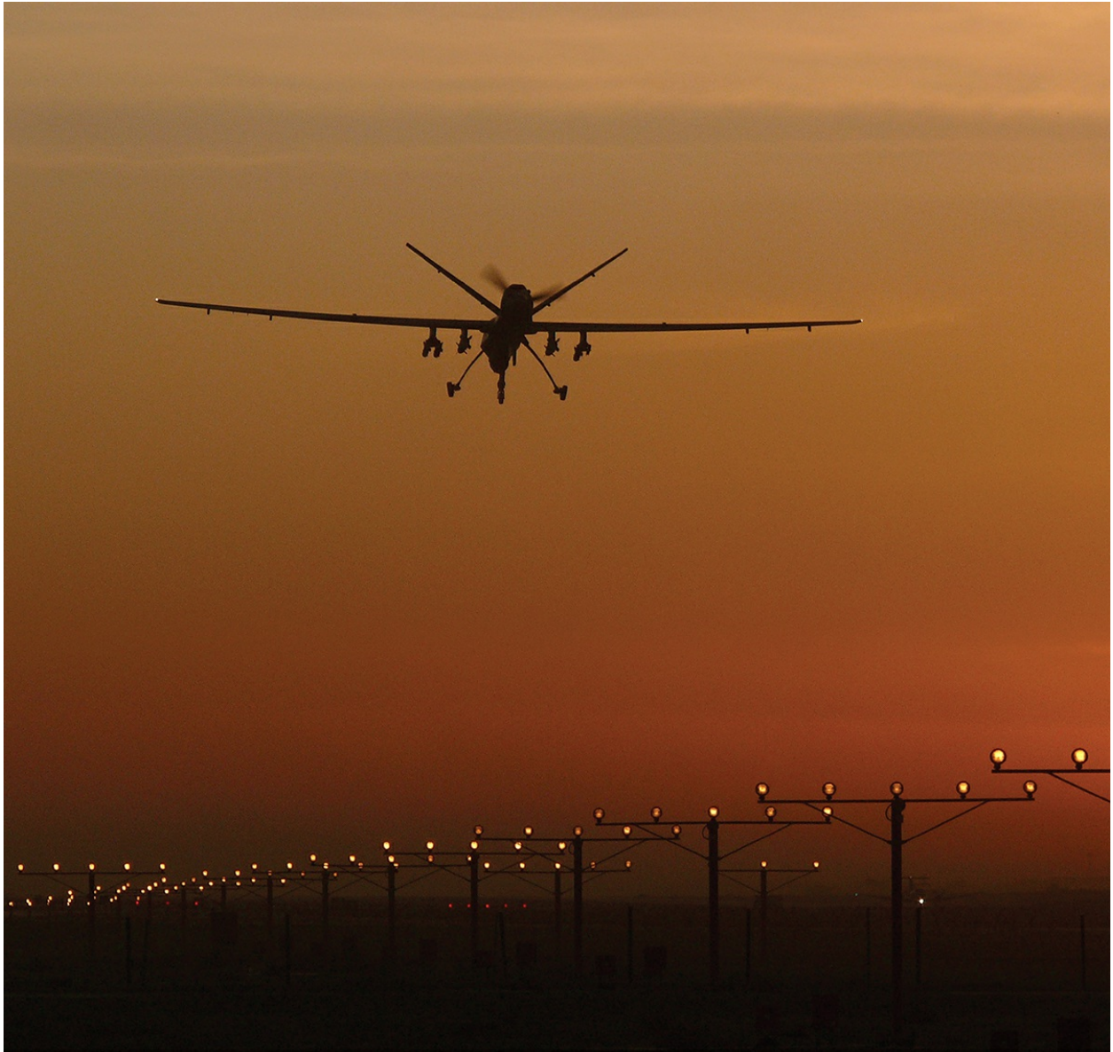
A General Atomics MQ-9A Reaper Remotely Piloted Air System (RPAS) of 39 Squadron on the final approach to Kandahar. It is armed with two GBU-12 500lb LGBs and four Lockheed Martin AGM-114 Hellfire missiles. During a mission the aircraft would be 'flown' remotely by a crew at Creech Air Force Base, Nevada, but the take-off and landing would be performed by a crew at Kandahar. (Stradling)
