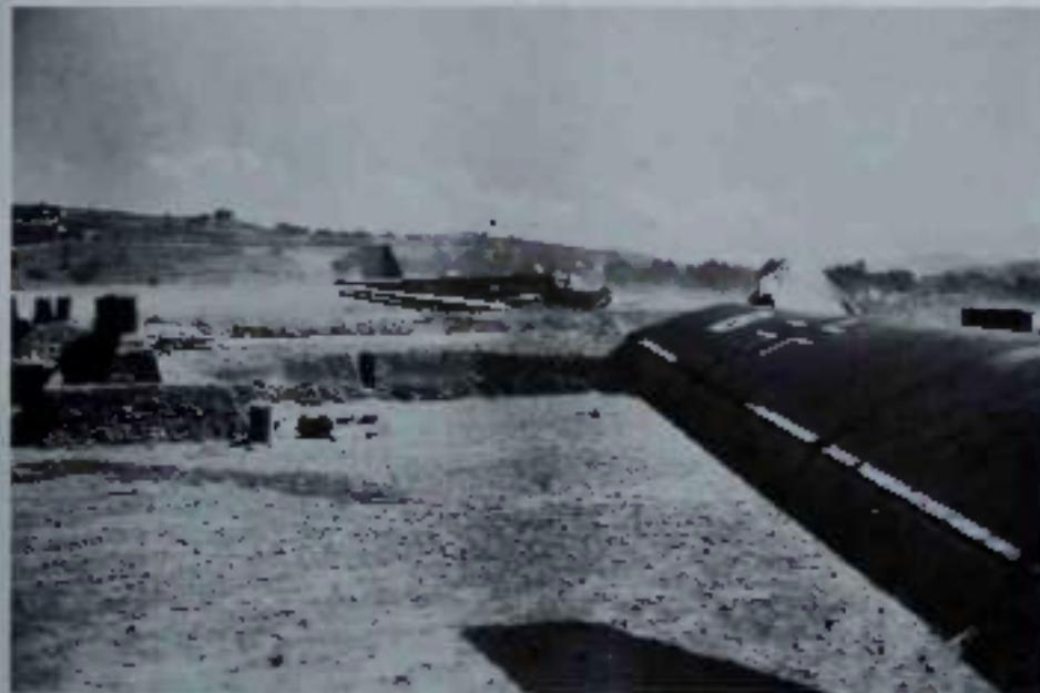
*Bottom: The approaching aircraft overfly some DFS 230 gliders that had landed earlier leaving skid marks from their plough-type brakes. The DFS 230A on the left has lost most of its port wing.*
