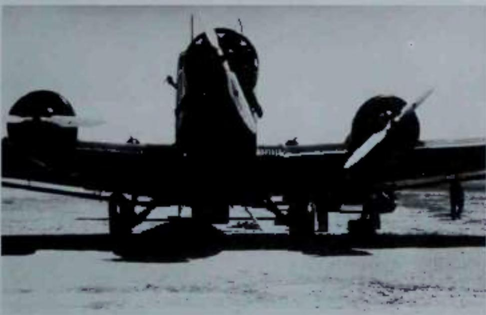
Centre: The squadron commander of 3.K/88, Hptm. Krafft von Dellmensingen had mounted two fixed MG 17 machine guns upon the inner mainplane of his Ju 52/3m to protect it against fighter attacks from dead ahead. These 'scare weapons' fully justified themselves in action.
