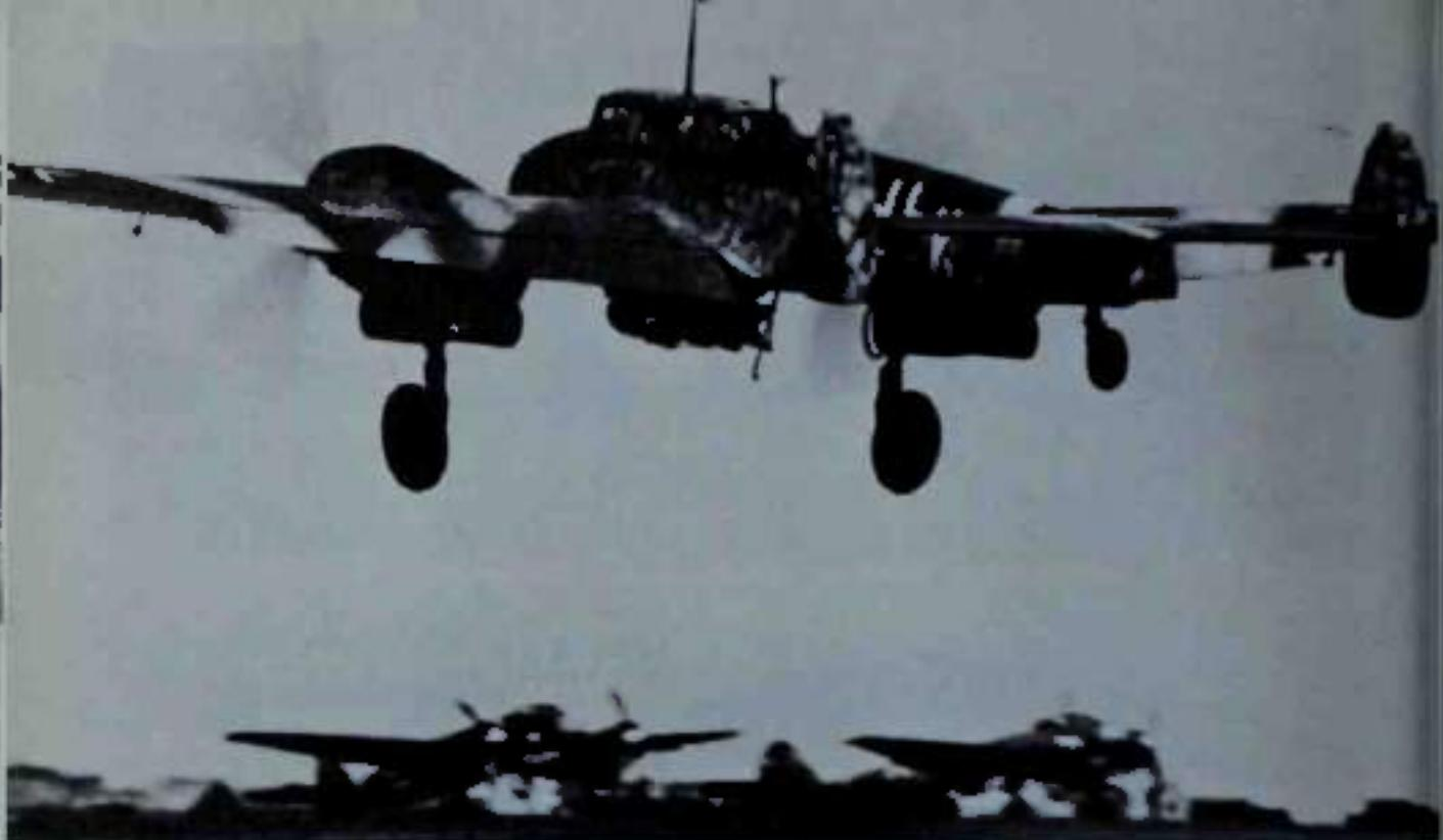
Top: Carrying two SD 250 (55lb) splinter bombs on its fuselage bomb racks, a Bf 110F-1 of II/ZG 1 takes off from Kharkov in June 1942. The Bf 110F-1 was the bomber version of the Bf 110 Zerstörer.
