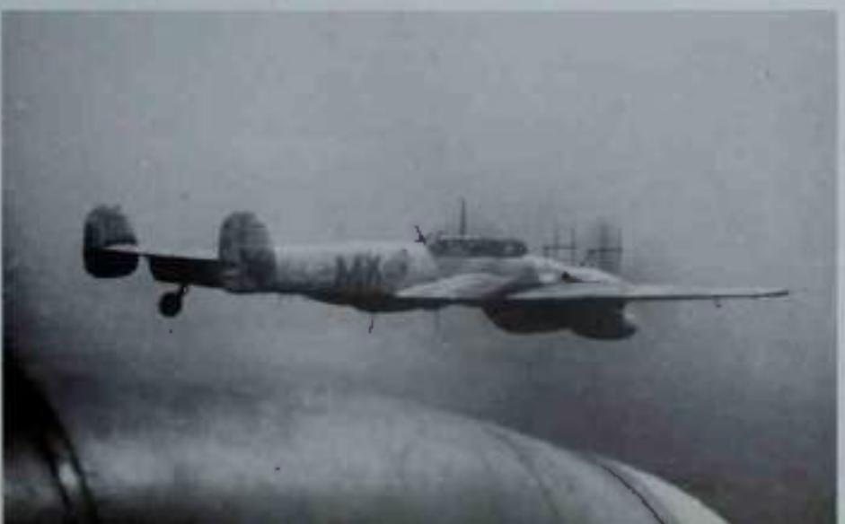
Bottom: The Bf 110G-6 piloted by Oblt. Becker during a twilight flight in summer 1944. The aircraft is equipped with the FuG 220 (Lichtenstein SN-2) air interception radar and carries additional underwing fuel tanks. The two small protuberances on the rear cockpit cover hide the gun muzzles of the 'Schrage Musik' ('Slanted music'), two obliquely-fitted 20mm MG FF cannon. Hptm Martin Becker (as he became) ended the war with 35 confirmed eight victories.
