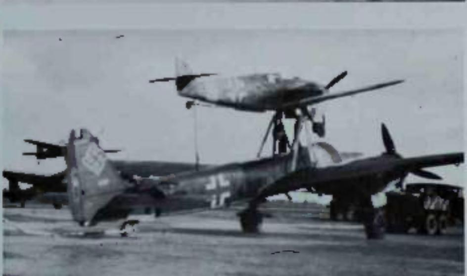
Centre: The 'Father and Son' aircraft too became a talking point during the last months of hostilities. A manned fighter coupled to the uncrewed component controlled the combination in flight towards the target and released itself after switching on the automatic flight controls of the powered 'flying bomb'. Shown here is a 'Mistel 1' (Mistletoe 1, nickname for this novel weapon) combination, a Ju 88 'bomber' with its Bf 109G control aircraft on its crudely at Burg near Magdeburg in April 1945.
