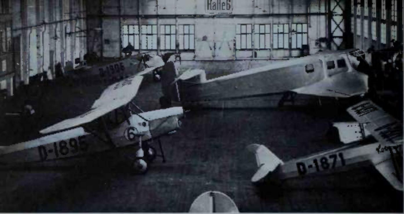
Top. During the crisis years the Albatros works kept its head above water with a varied construction programme. Four different types of aircraft are seen in this hangar, the L. 101 (D-1895), L. 109 (D-1906), L. 79 (D-1871) and (without markings) L. 82 transport. In 1932 the Albatros works were taken over by Focke-Wulf Flugzeugbau.
