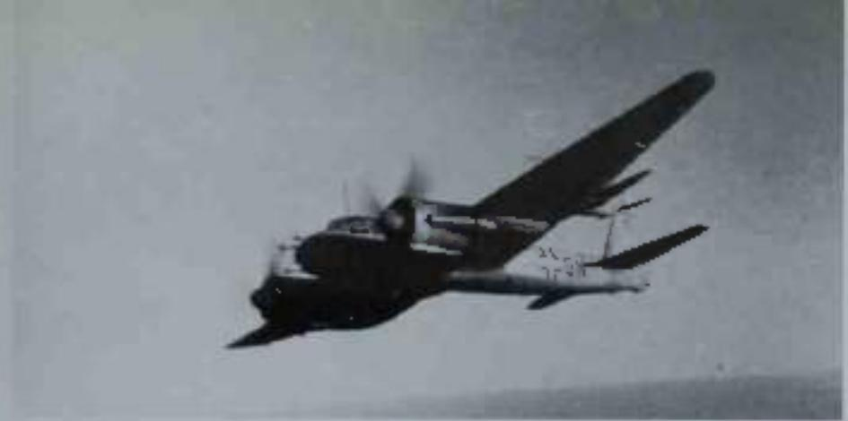
Top: A Ju 88C-6 of 3/NJG 2 over Holland. This night fighter is equipped with the FuG 212 Lichtenstein C-1 air interception radar in the nose and fitted with flame dampers over the engine exhaust stacks.
