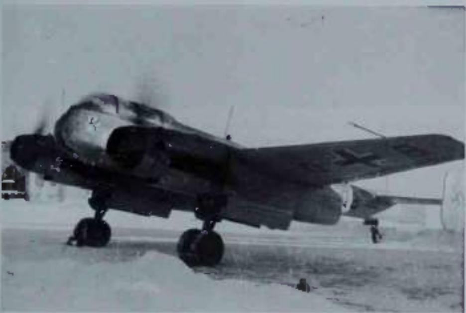
*Centre: Only a few examples of the Arado Ar 240A were built, one of which, the GL-108, was being temporarily used by 3(F)196 long-range reconnaissance Staffel. However, the pilots could not get used to the flight behaviour of this odd aircraft. The machine is depicted at Kharkov in February 1943.*
