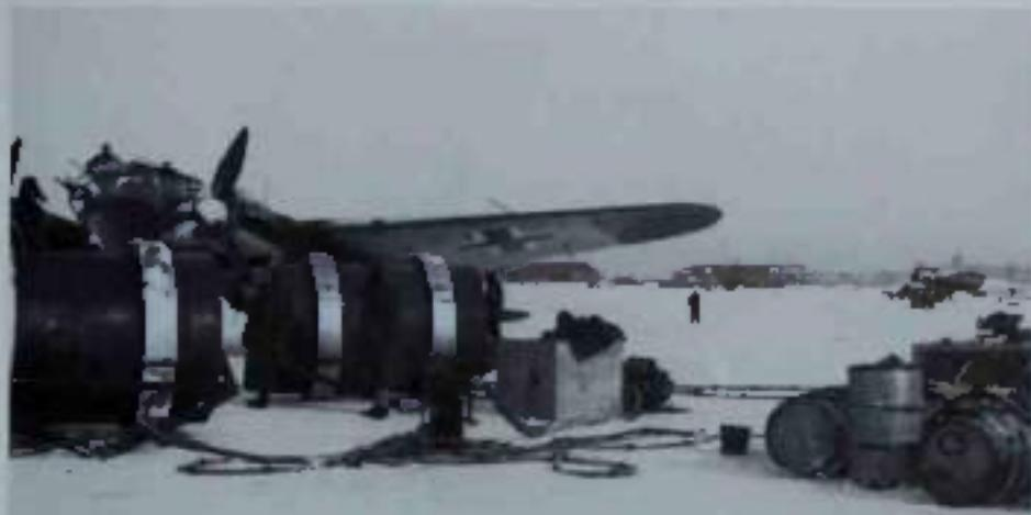
*Center: Rolling petrol tanks. Steel cylinders, 1.60 ft in diameter, strengthened by wire strips, could be rolled directly to the aircraft to speed up refuelling in Rosebud winter conditions. Some He 111 bombers were also impelled to fly in supplies to the Demyansk 'cauldron', Pskov, February 1942.*
