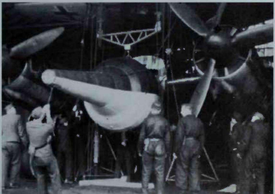
Bottom: Attaching the 3.8-ton (8377lb) warhead to the airframe of the specially prepared Ju 88. These 'Mistel' combinations were first used against the Allied supply ports in Normandy in June, 1944, and then against the Neisse and Oder bridges in the East and the Rhine bridges in the West during the final months of the war.
