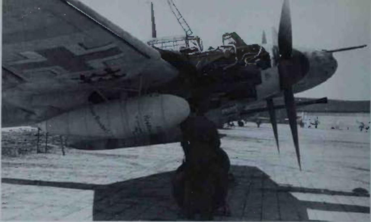
*Top:* To hold their own against the four-engined Allied bombers, the calibres and number of weapons carried by German fighters had to be increased. The depicted Bf 110G-2 'Vulkanauswärter' (formation destroyer) is armed with 1 × 30mm BK 3.7 cannon under the fuselage and 2 × 20mm MG 151/20 cannon in the nose.
