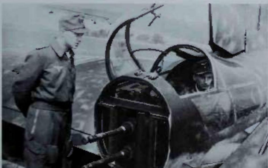
*Bottom:* A 'field modification' of the He 177A tail gun position. The normal tail armament of one 20mm MG 151/20 cannon has been replaced by two 13mm MG 131 heavy machine guns for greater volume of fire.
