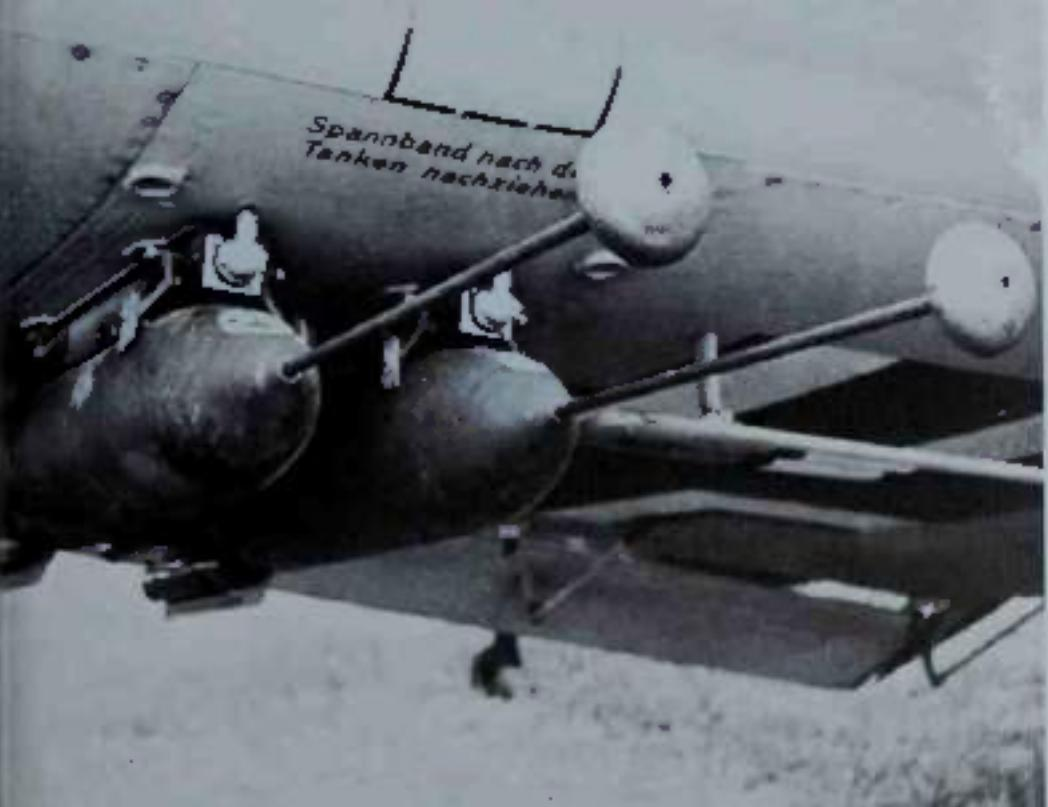
Bottom: To achieve the optimum fragmentation effect (by 50kg (110lb) SD 50 splinter bombs were fitted with special stand-off pipes), the so-called 'Dienst-Sparpfeil' (Dienst asparagus). These bombs exploded just above the ground and were especially effective against groups of vehicles and troop assembly areas. They were named after their inventor, Oberst Dienst, a noted Stuka pilot and commander.
