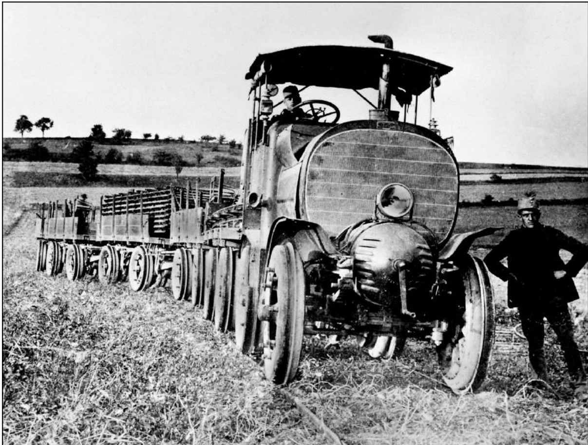
Based on trials with the earlier A-Train Porsche and Austro Daimler developed the multi-trailer B-Train, ten of which went into service during the war to deliver supplies to the army's huge mortars and howitzers.
