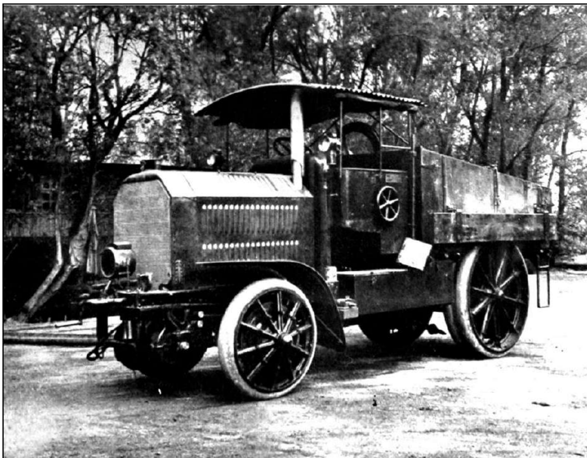
Enlarged and paired rear wheels were hallmarks of Austro Daimler's M 12, which was ready for action in 1913. Known as the 'Hundred' for the power of its 20.3-litre six-cylinder engine, the M 12 saw major service in the First World War.
