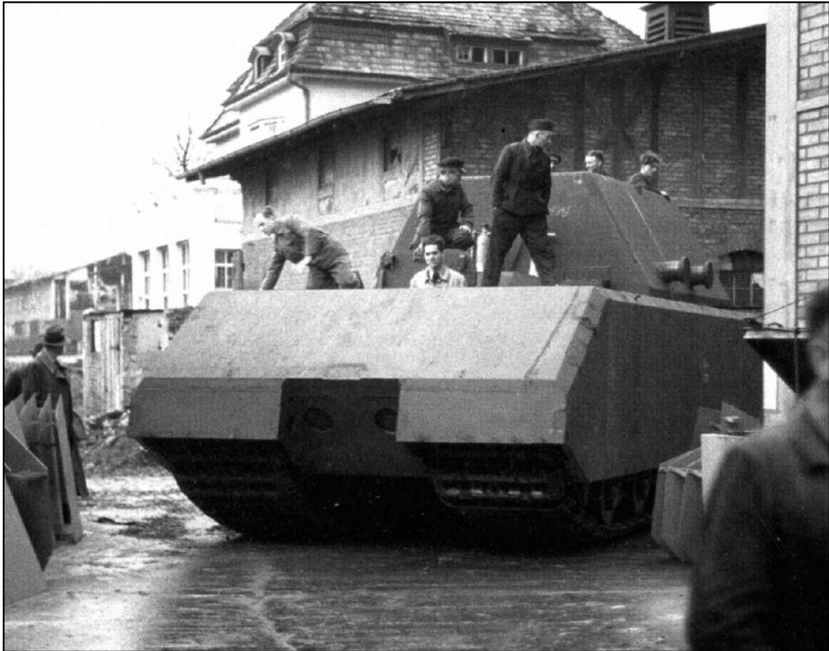
Karl Gensberger was at the controls of the first Maus as it inched out of Alkett's Berlin works at Christmastime 1943, carrying its mass-substitute turret. It manoeuvred perfectly in response to its controls.
