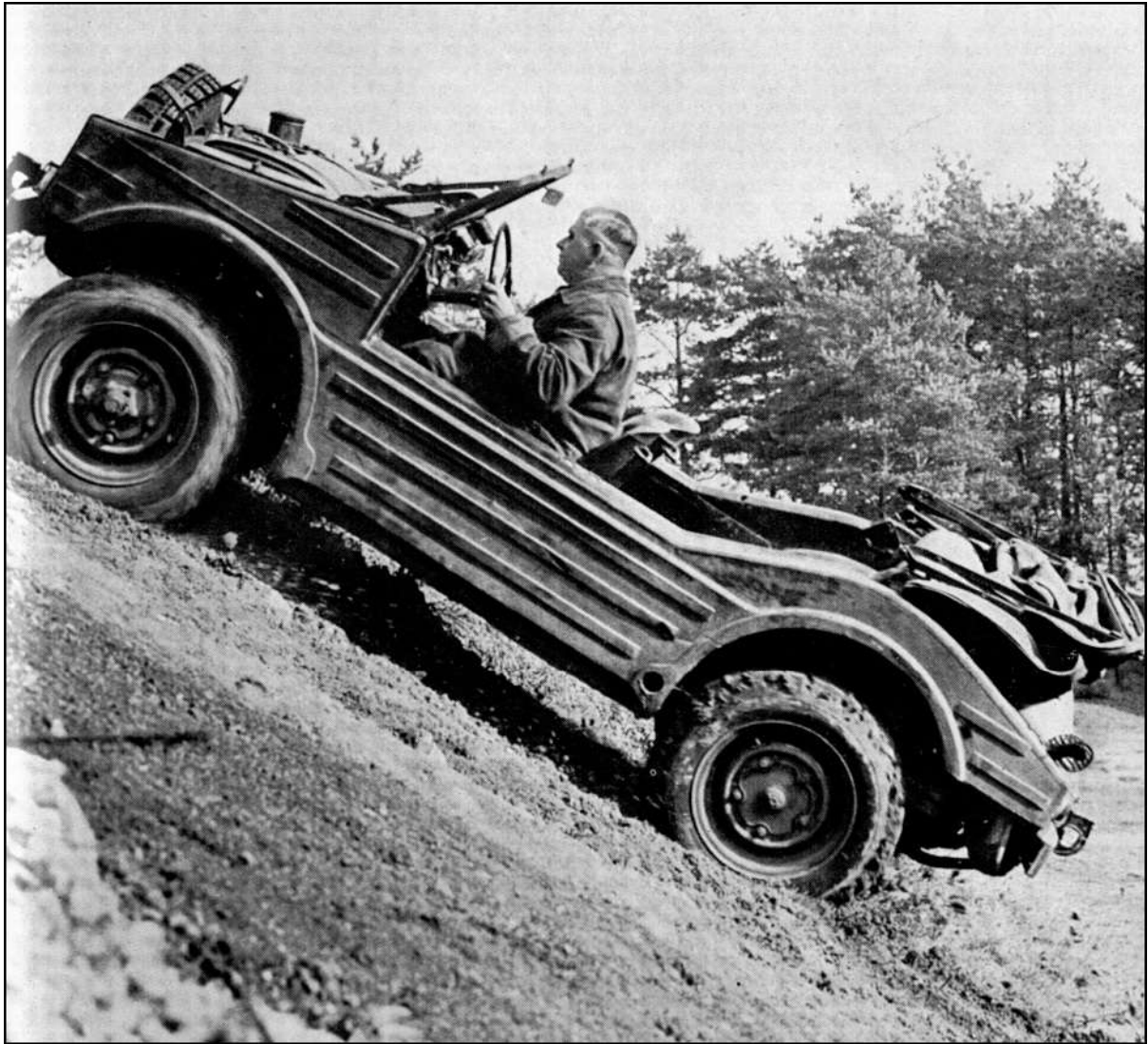
As completed with its ribbed bodywork the T597 was both more 'military-looking' and agile with its five-speed gearbox. Porsche spent some DM1.8 million on its development and body shells sourced from Karmann.
