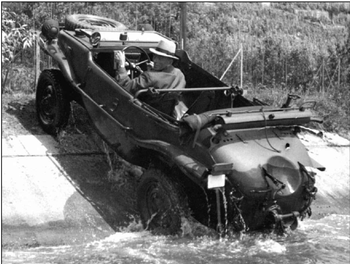
Instead of the prototype's abbreviated windscreen the final Schwimmwagen had a full-width screen. Its silencer was well clear of the water from which it emerged with its propeller still in seagoing position.
