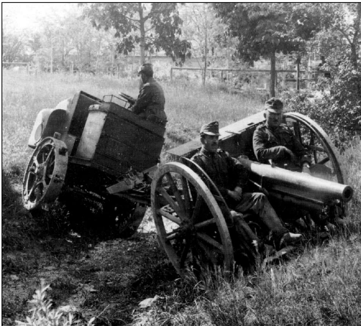
Seen in a 1915 test on the Austro-Daimler grounds, this was the initial experimental version of Porsche's Pferd or 'Horse', a two-wheeled tractor that could tow an artillery piece or other field equipment.
