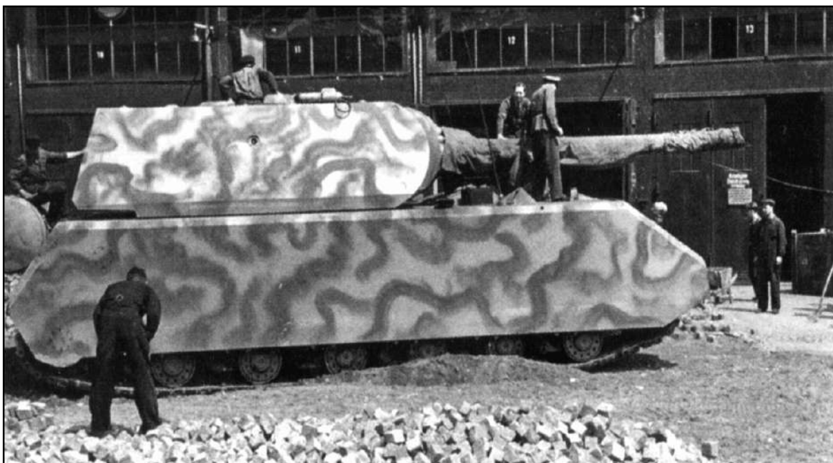
The Maus had a devastating effect on the stone-block paving of the Panzerkaserne yards. This resulted from a combination of its sheer weight and the wiping effect during manoeuvres of its unusually wide tracks.
