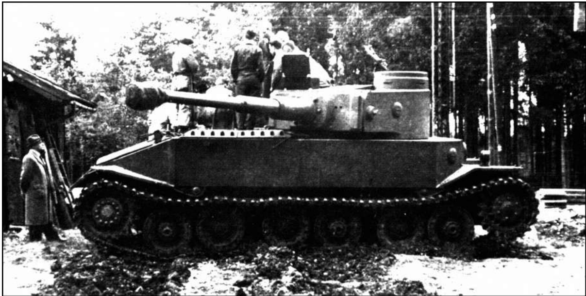
Shown with its barrel aimed rearwards, the Type 101 Tiger (P) underwent trials. Porsche strongly preferred drive through the rear sprockets, which left unstressed the upper return half of the caterpillar track.
