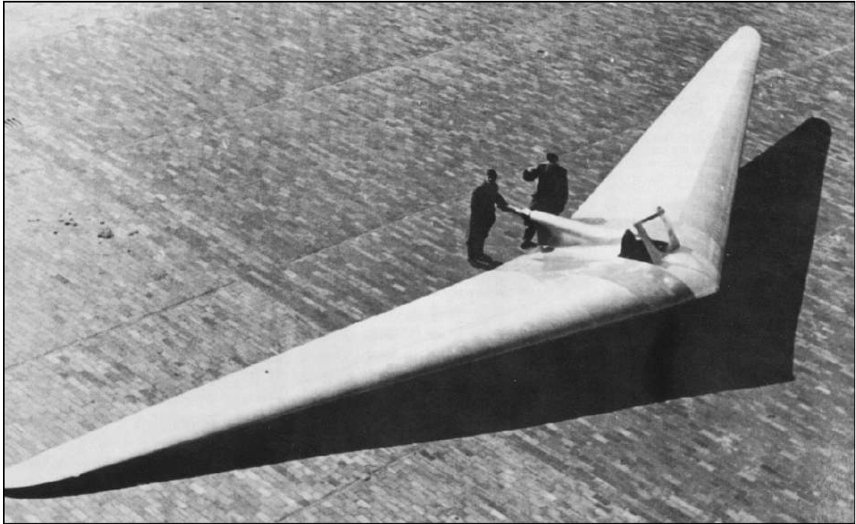
Easily as futuristic as any aircraft of 1944, the H IIIe flying wing of the Horten brothers was one of many prototypes they built and tested. Its Porsche-modified VW engine provided a smooth 32bhp.
