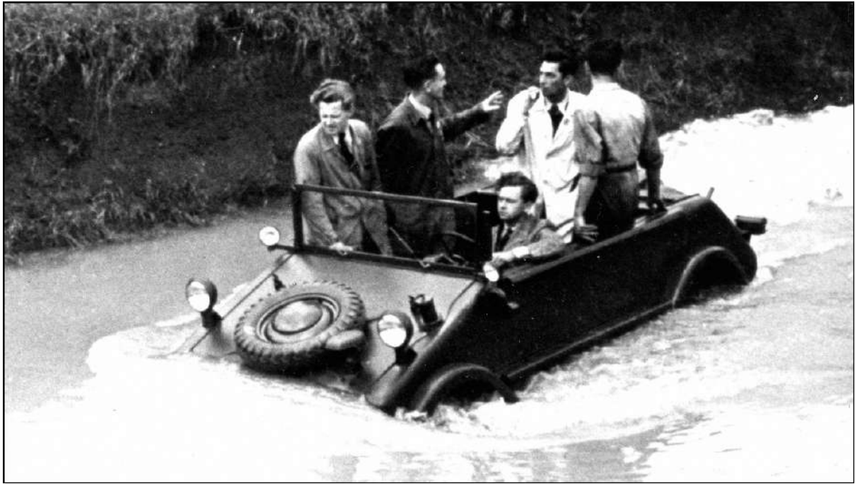
The end of September 1940 found Ferry Porsche at the wheel of the first Type 128 prototype as it surfed the Max Eyth Reservoir with a full complement aboard. Its Drauz-built body was doorless.
