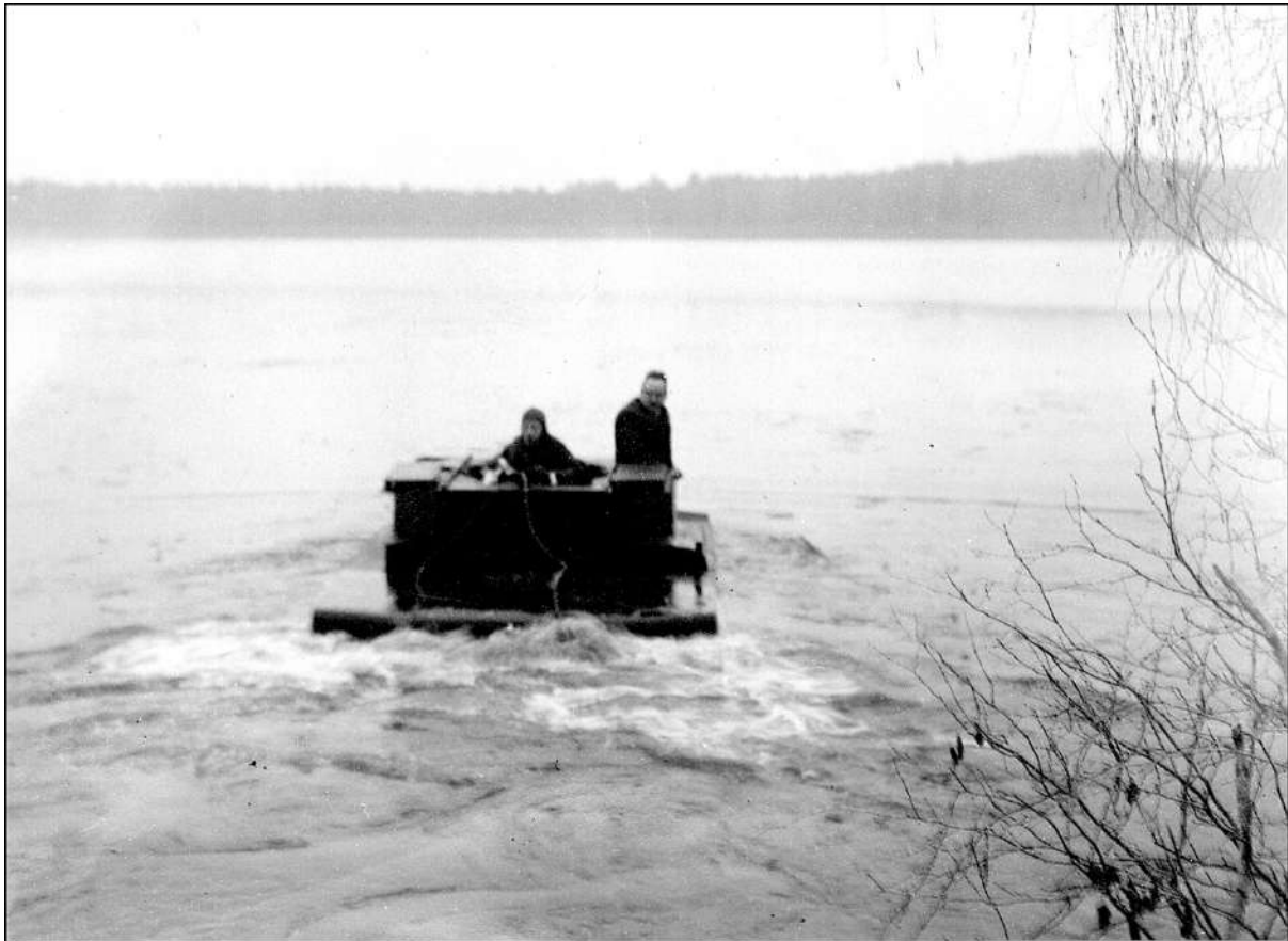
Although with a minimum of freeboard, the MTW 1 was a good swimmer in both directions. Plans for further trials in Russia in 1932 were dropped although the underlying concept had acknowledged potential.
