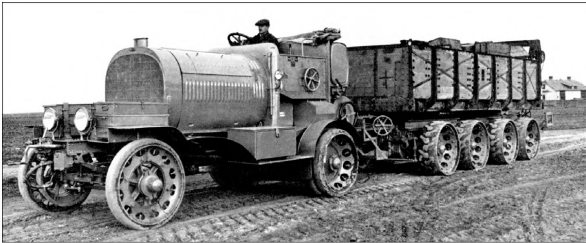
Towing a mixed load in its powered trailer, an Austro Daimler C-Train gave a hint of its colossal dimensions. Not without reason mountain troops saw the guns and their electrified deliverers as their 'Panzer-smashing big brothers'.
