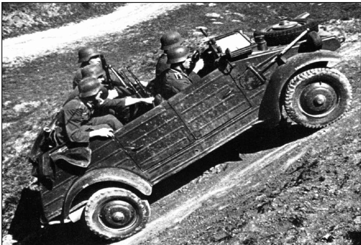
This striking image of the Type 82 Kübelwagen with its complement of five soldiers showed the benefit of adopting bench rear seating. The use of doors was considered a radical departure for this class of vehicle.
