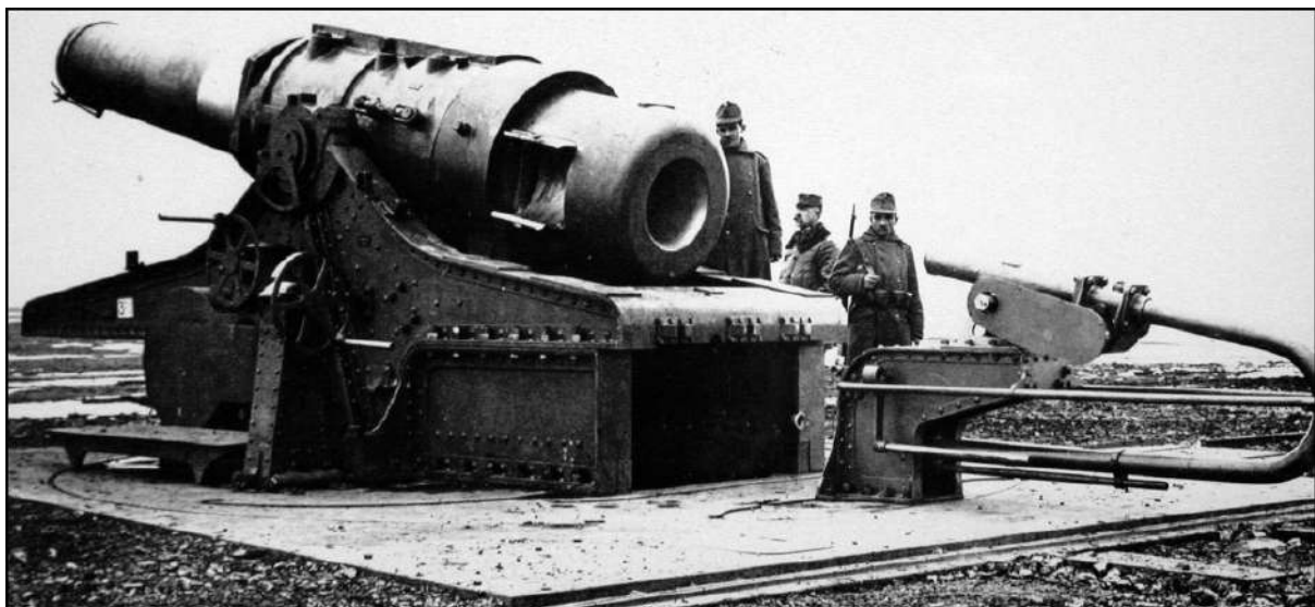
Gudrun was the second Skoda M 16 howitzer to be completed. The total produced during the war came to ten of these 380mm guns. They could only be transported by dismantling them into their constituent parts.
