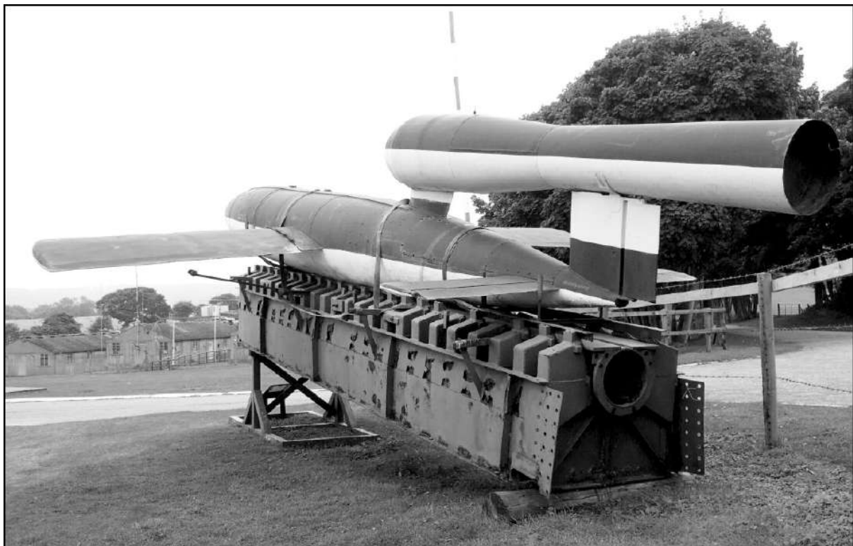
A fragment of launching ramp showed the circular passage through which the piston travelled to launch
