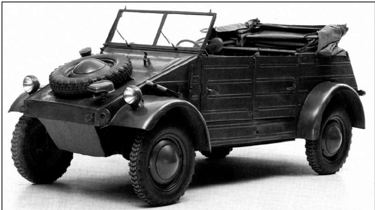
As finally realised in 1939 and redesignated the Type 82, Porsche's military version of the VW looked tough enough. Ingenious engineering gave it parade-speed pace plus the added ground clearance that the Wehrmacht required.
