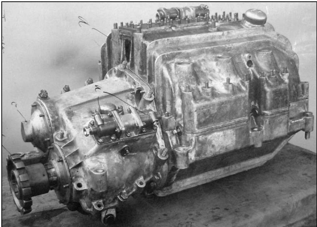
The aluminium housings of the GT I's transmission were loosely assembled for trial purposes. Hydraulic cylinders on the smaller case in the foreground shifted the two-speed gearbox giving the tank a choice of overall ratios.
