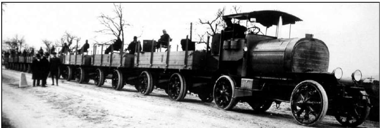
From the B-Train's generator car, with its 120bhp six-cylinder engine, electrical power for propulsion was delivered by cable to alternate trailers among the ten allocated to each train.
