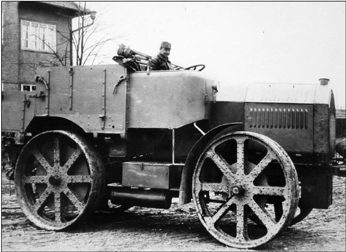
Porsche created a new 13.5-litre four-cylinder engine for his M 17 tug, using vee-inclined overhead valves to produce 80bhp at 800rpm. Appropriately dubbed 'Goliath', it entered service during the First World War.
