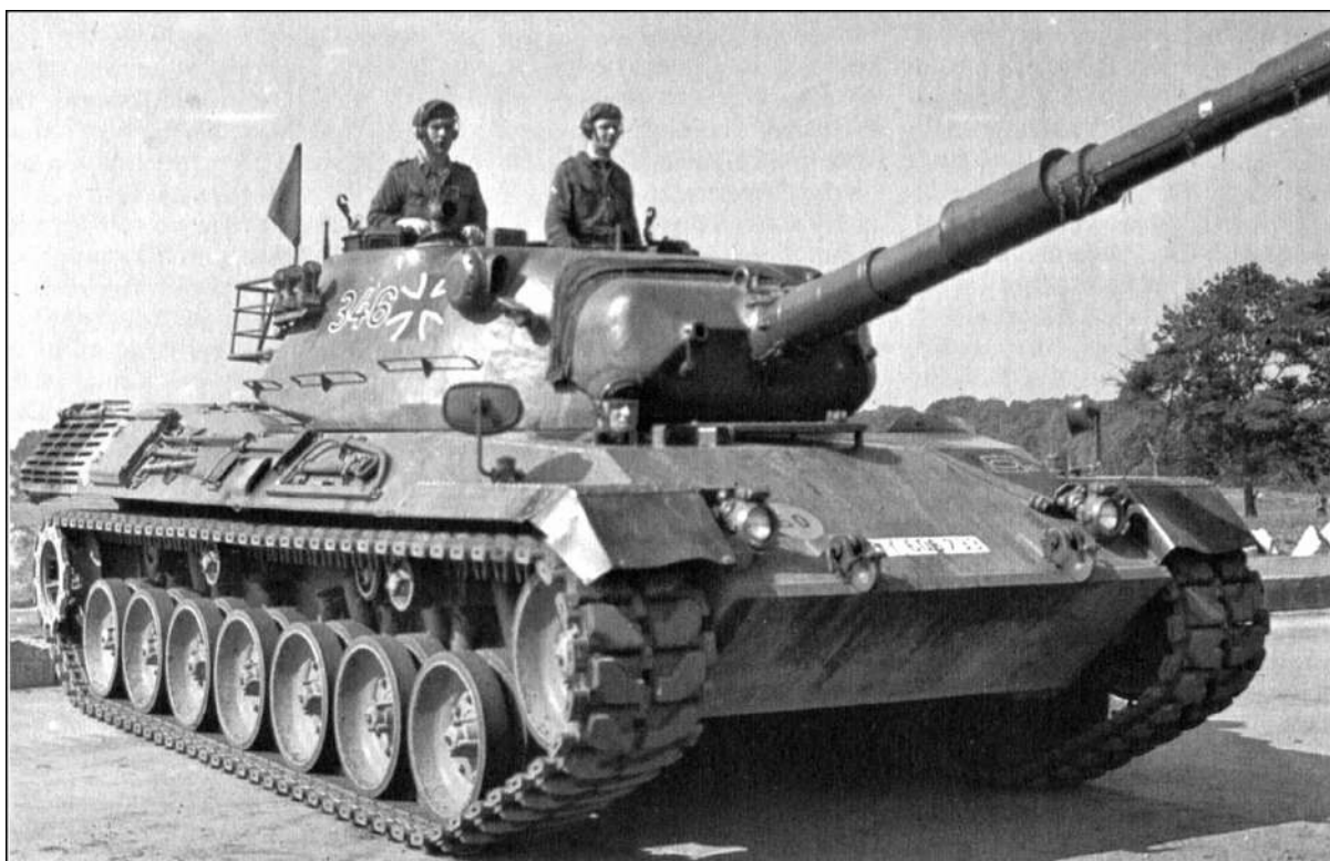
The Porsche-designed Type 714 Leopard was acquired and fielded by numerous nations. Although able to reach 40mph, in spite of its torsion-bar suspension 30mph was the maximum its crew could tolerate on uneven terrain.
