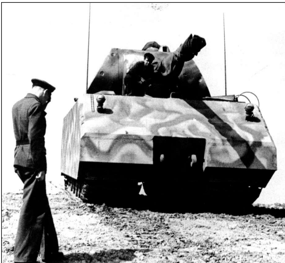
Arriving at Böblingen on 10 March 1944, the second Maus prototype was fitted with its correct turret during May. Both its curved turret face and frontal glacis were sloped to deflect incoming munitions.
