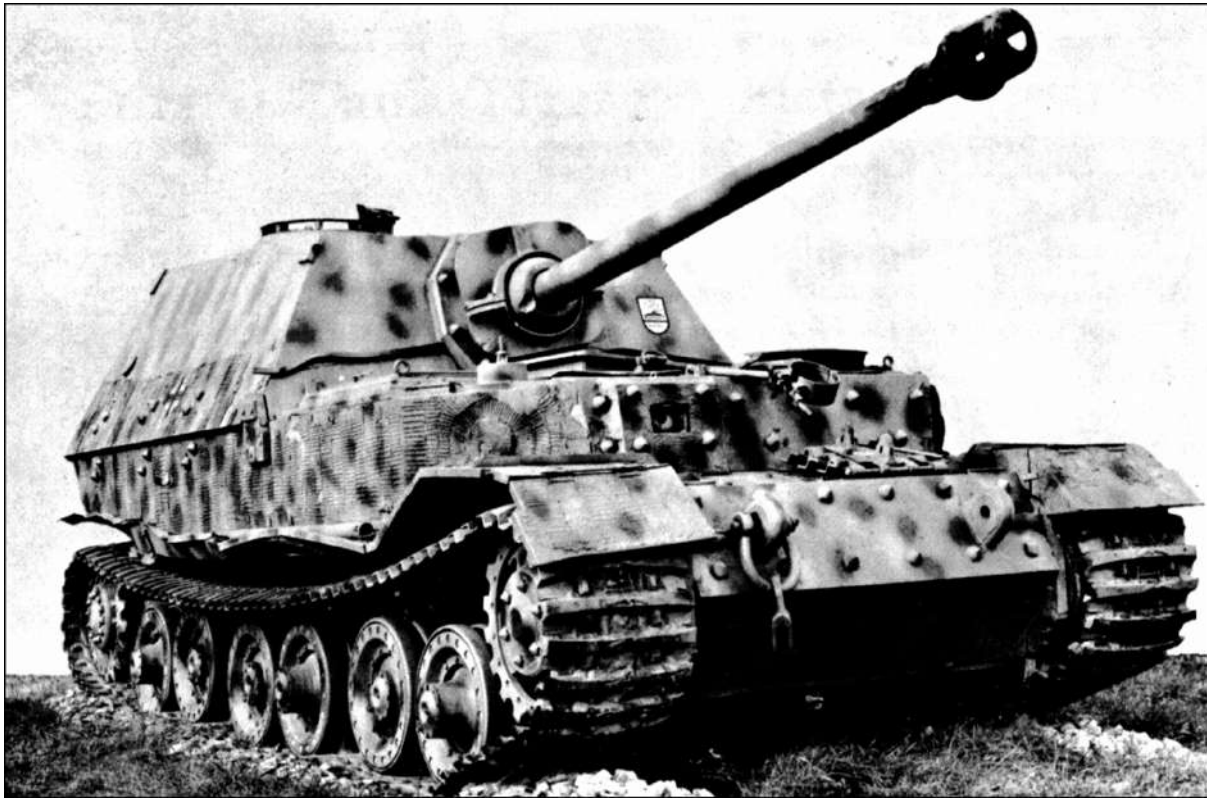
Forty-eight serviceable Ferdinands were recalled to St Valentin for refitting over the 1944/45 winter. They received a machine-gun aperture, commander cupola and rough-finished Zimmerit coating to shrug off magnetic limpet mines.
