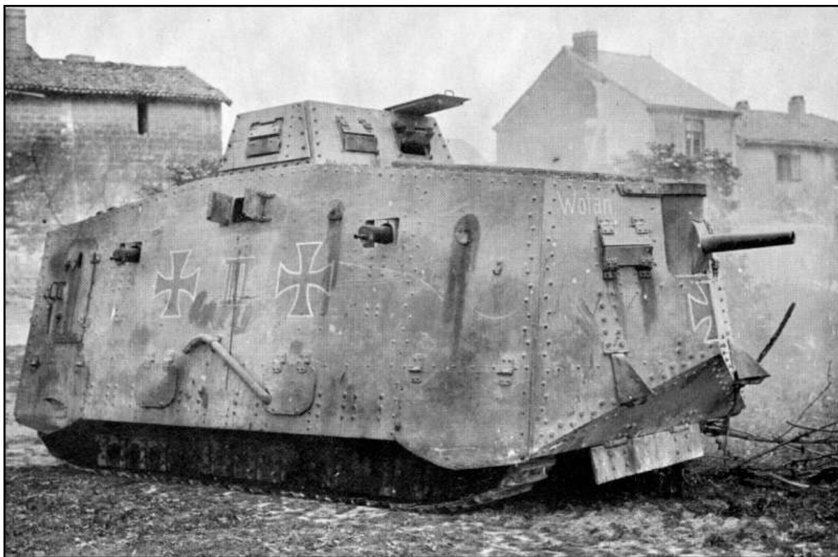
Stuttgart's DMG cut its teeth on tanks with the A7V of 1917, a design by Joseph Vollmer powered by two 100hp fours. With 18-strong crews, several took part in history's first tank-to-tank battle in April 1918.
