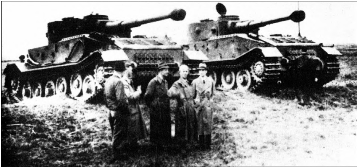
Two Type 101 Tiger (P)s rested between trials with their guns slung to the rear. Ultracompressed production timing gave little opportunity for perfection of its engines, which continued to be troublesome in spite of modifications.
