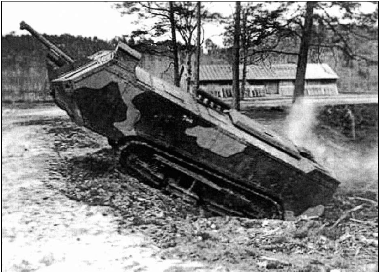
Riding on American Holt caterpillar tracks, the French Saint-Chamond tank of the First World War was a respectable performer with its Crochat-Colardeau electric drive from a Panhard-Levassor engine.
