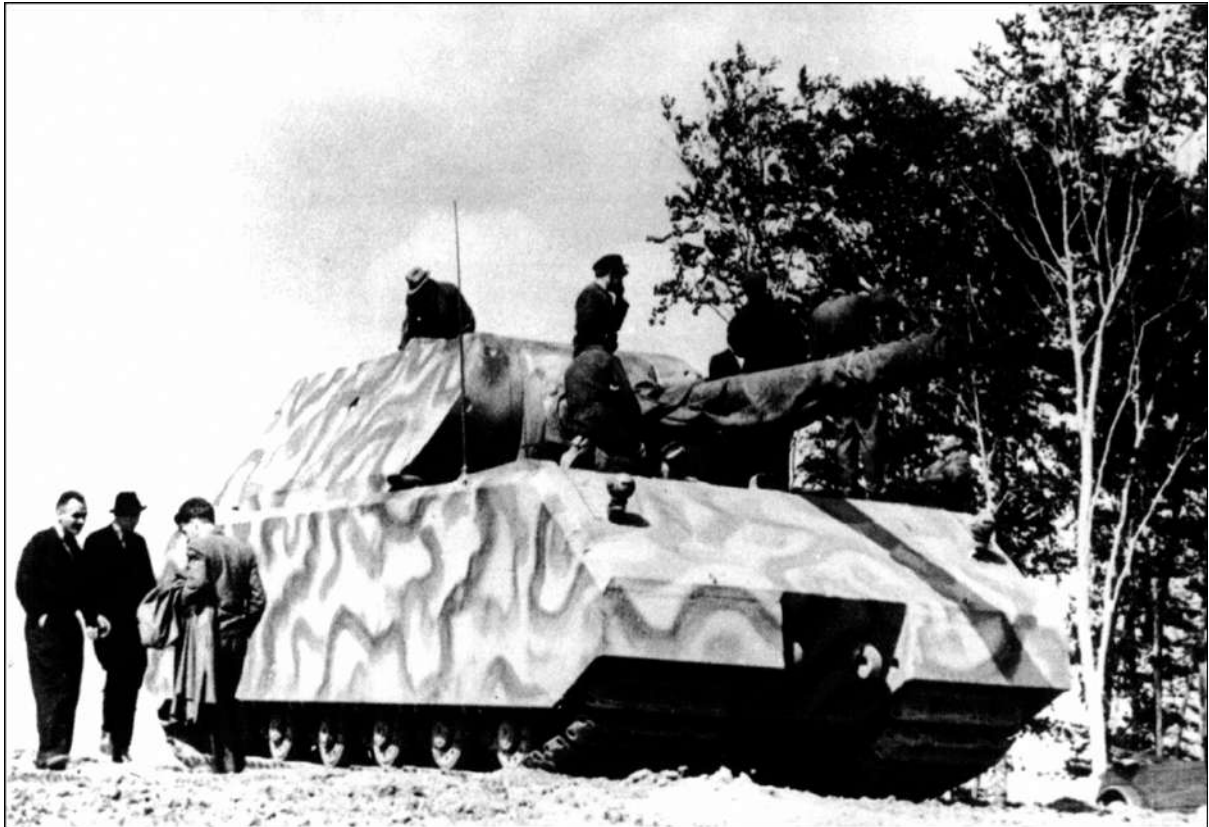
Developed by Daimler-Benz from its aero V-12s, an MB 517 diesel engine was fitted to the second Maus, giving improved fuel economy. Both Type 205 prototypes were shipped to the Kummersdorf test grounds in October 1944.
