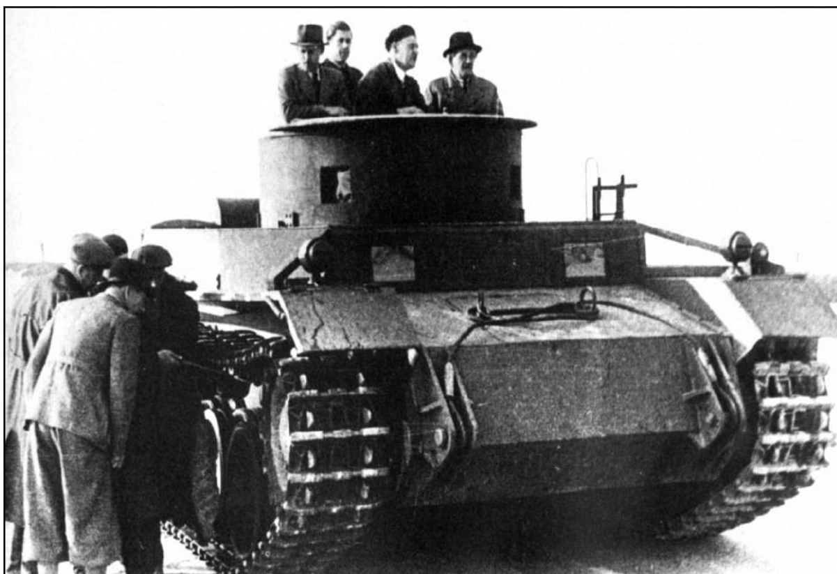
Porsche, at right in its conning tower, oversaw trials of his Type 100 tank. Built in the Nibelung Works where Franz Xaver Reimspiess was chief designer, only one of its two prototypes was made fully operational.
