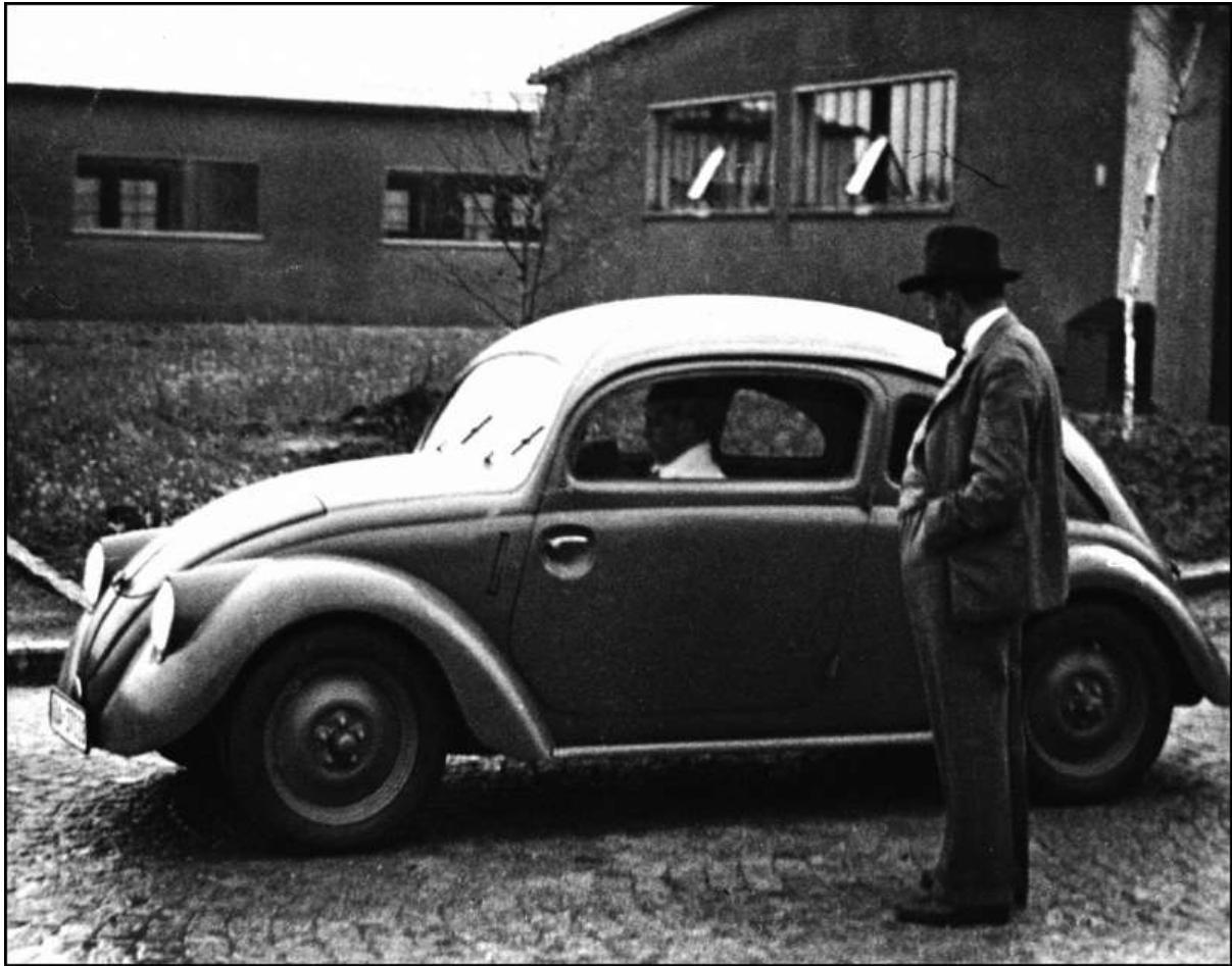
In typical stance Porsche looked on as one of the V30 prototypes of 1937 went out for its trials. One of the results of its evaluation was the decision to make the final design of 1938 larger, a full four-seated car.
