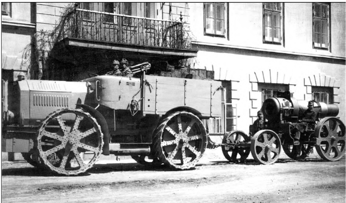
In front of one of the works billets at Austro Daimler in 1917 an M 17 'Goliath' towed a Skoda M 11 305mm mortar. Cleated wheels gave it traction to reach speeds of up to 9mph.
