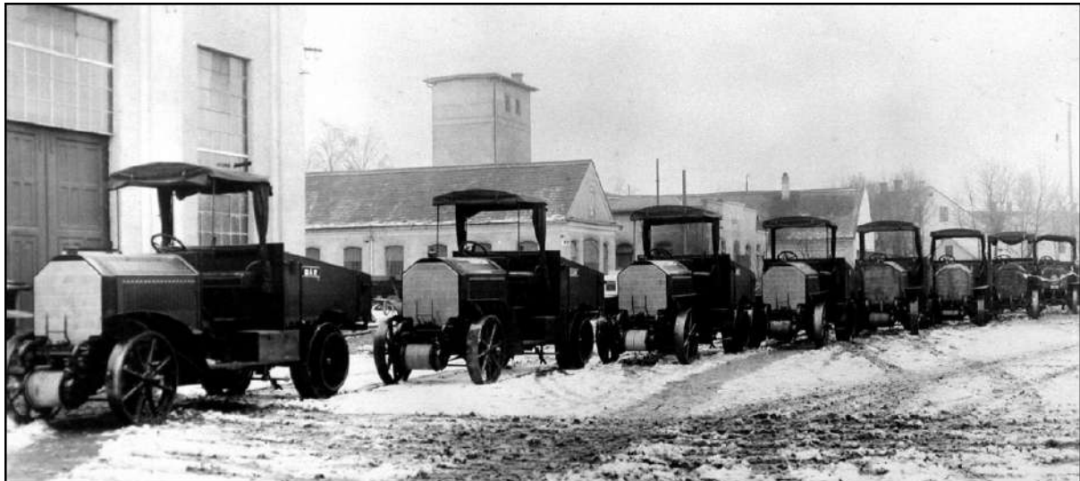
Its power increased to 80bhp, by 1911 the M 08 tug evolved into the M 09, eight of which awaited collection by the army in Austro Daimler's courtyard at Wiener Neustadt.
