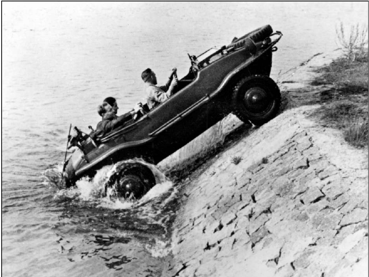
With its shortened wheelbase the Type 166 gained agility in entering and leaving the water as tests demonstrated. Its development was funded by the Waffen SS, which provided engineering draftsmen to Porsche for the project.
