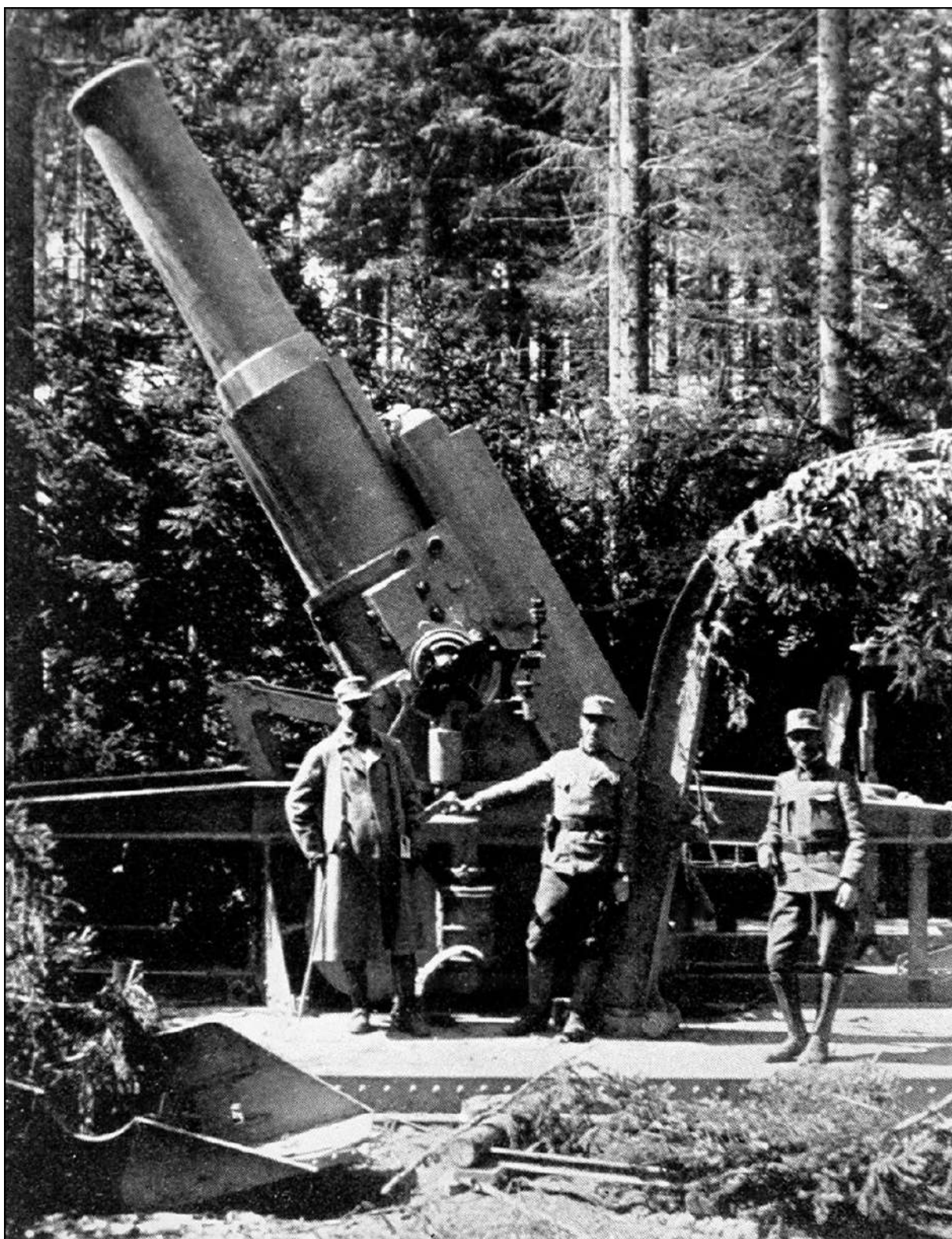
The first of two such awesome 380mm Skoda howitzers, Barbara was given her initial tests in January 1916. The complete M 16 assembly, with barrel, cradle and base plates, scaled 90 tons.
