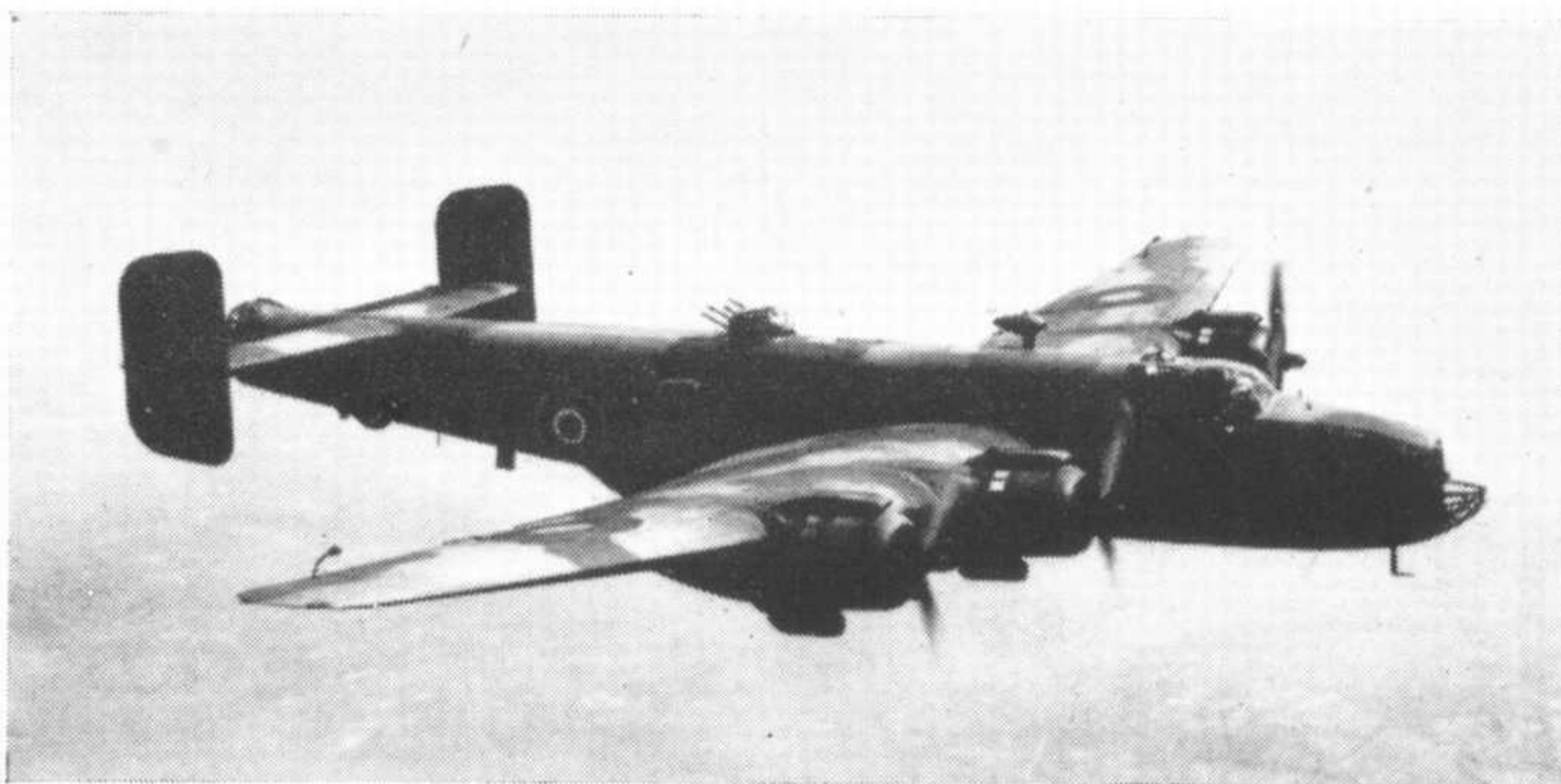
An aeroplane which developed almost out of all recognition—compare with the photograph on page 29—was the Handley Page Halifax. On this B. Mk. VI, part of the ventral H2S radar scanner can be seen below the roundel.
