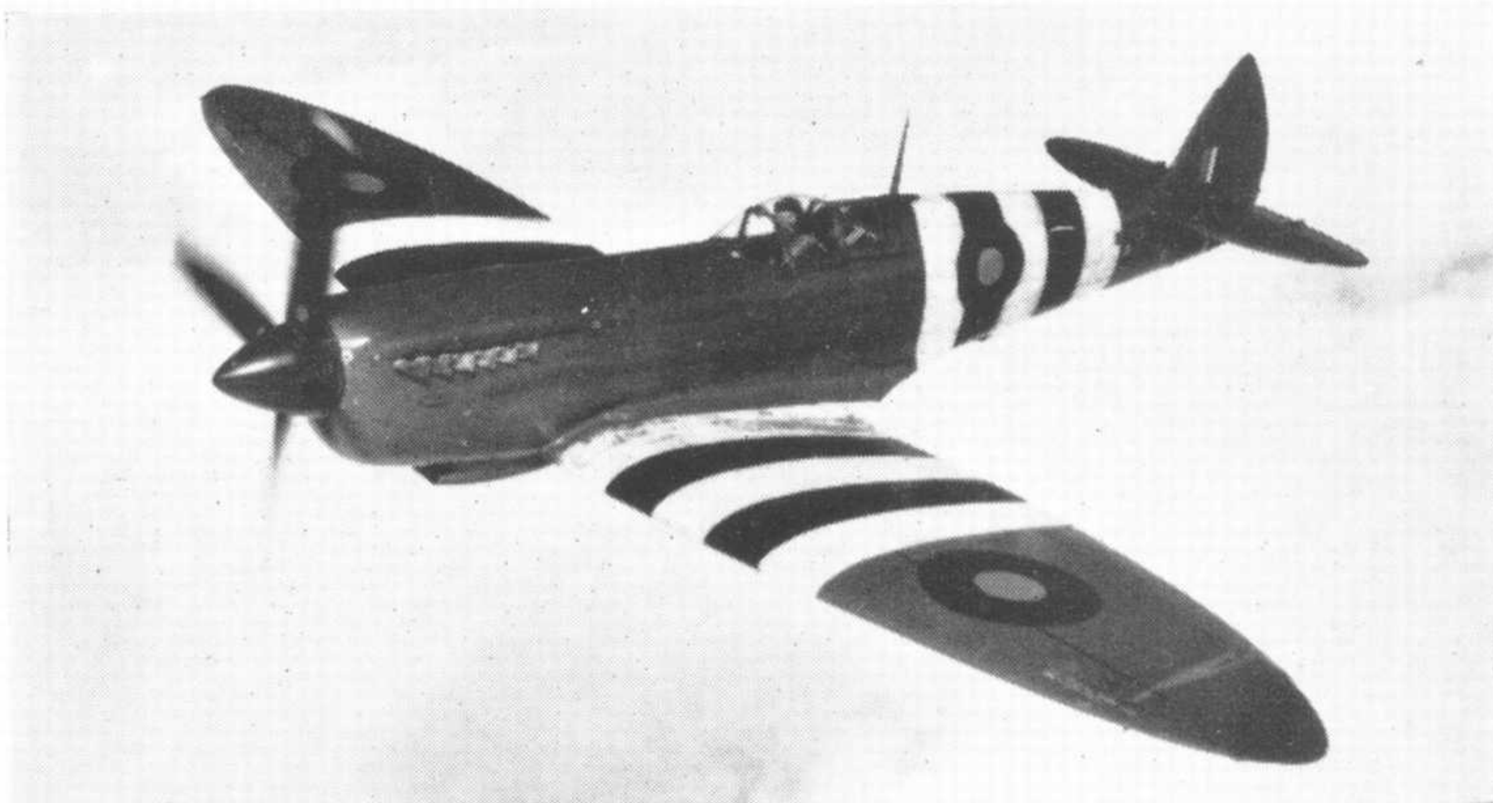
Spitfire P.R. Mk. XI. Note the pointed fin and rudder.
