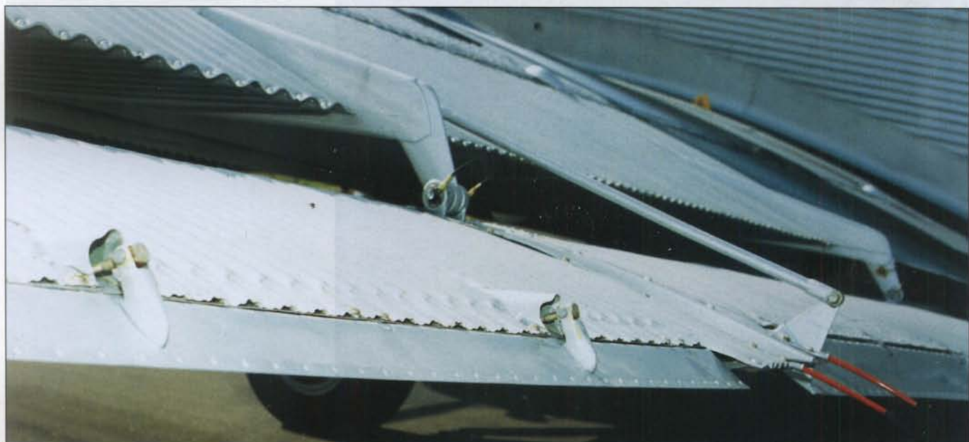
Part of the port wing aileron system.
