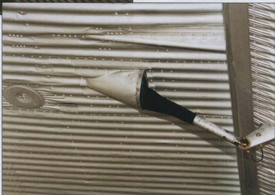
Aileron control rods on the starboard side of the wing.
