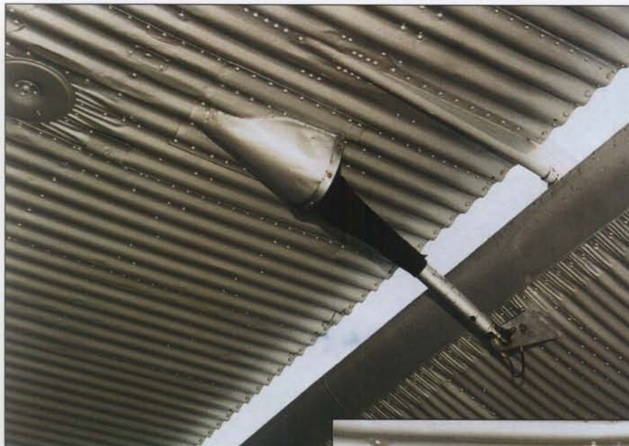
Aileron control rods on the starboard side of the wing.
