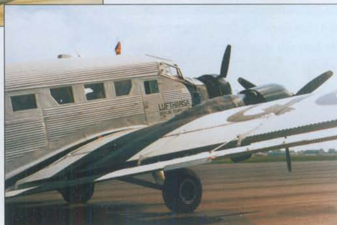
These photographs show clearly the corrugated surface on both fuselage and mainplane.
