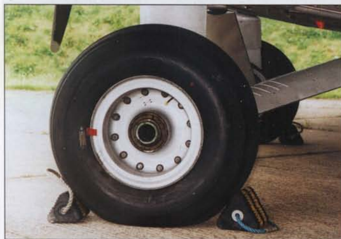
Photographs of the left wing undercarriage. Note the non-original wheels.
