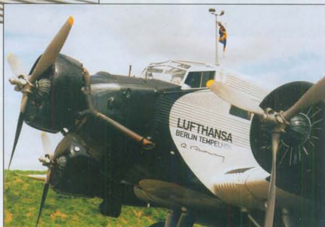
This frontal view clearly depicts the engine cowlings as well as the exhaust of the centre engine.
