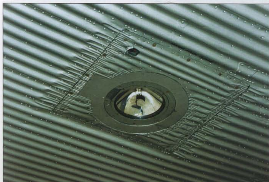
Landing light mounted on the bottom of the wing.
