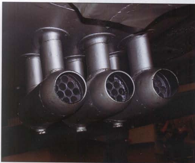
Views of the oil coolers located on the undersurface of the centre section.
