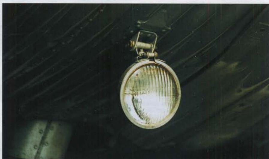
Landing light mounted on the wing, forward of the starboard undercarriage.
