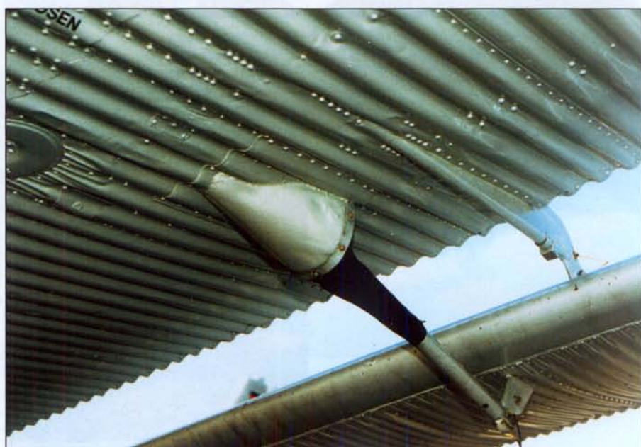
Aileron control rods on the port side of the wing.
