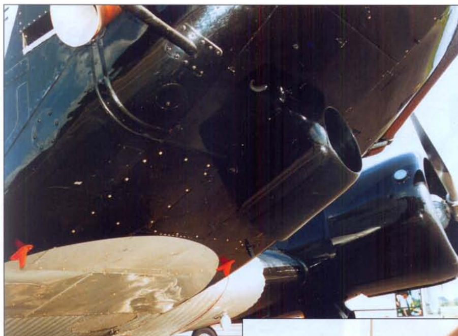
Oil radiator underneath the centre.
