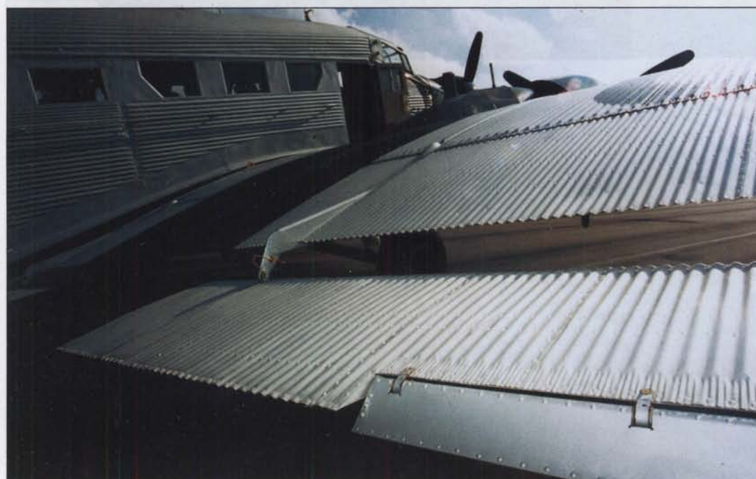
Mounting and system of flaps and ailerons of the starboard wing.
