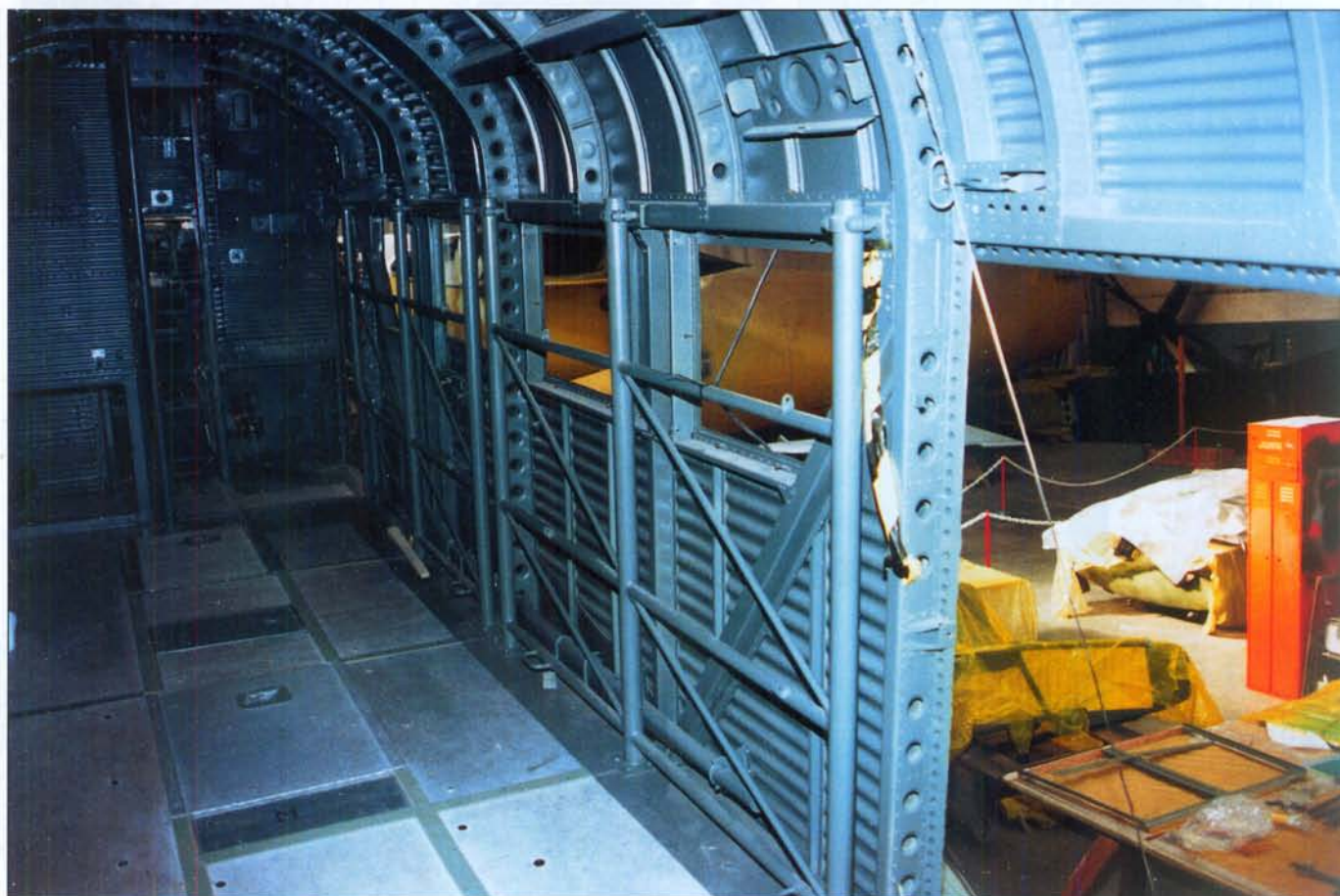
Fuselage interior facing forward clearly showing the corrugated outer skin and internal bracing.
