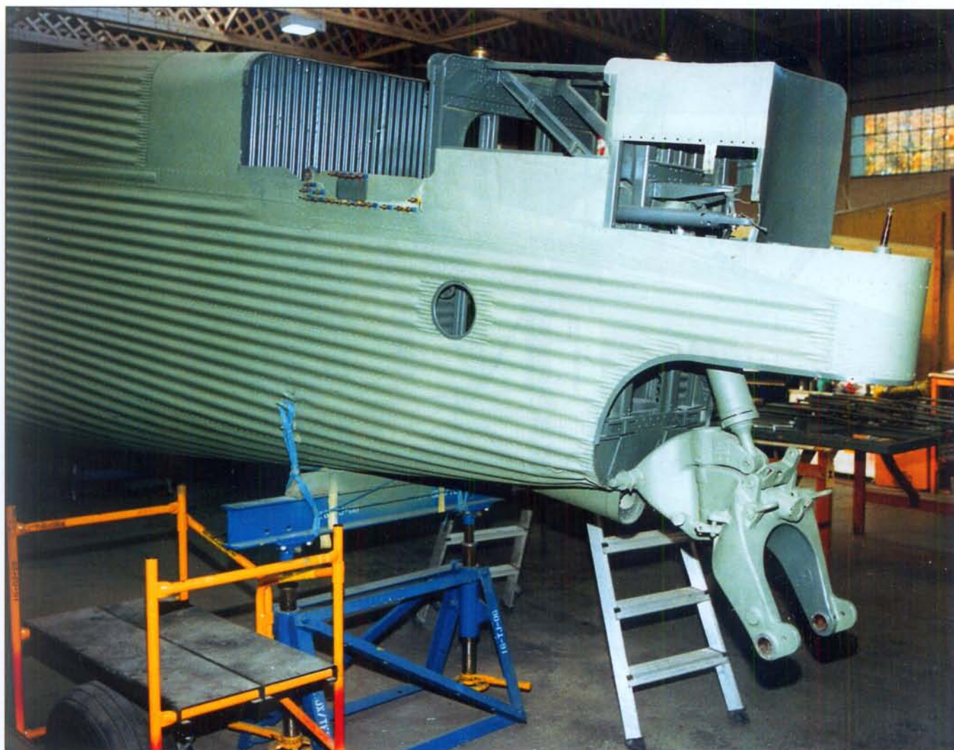
Tail wheel yoke and shock absorber.
