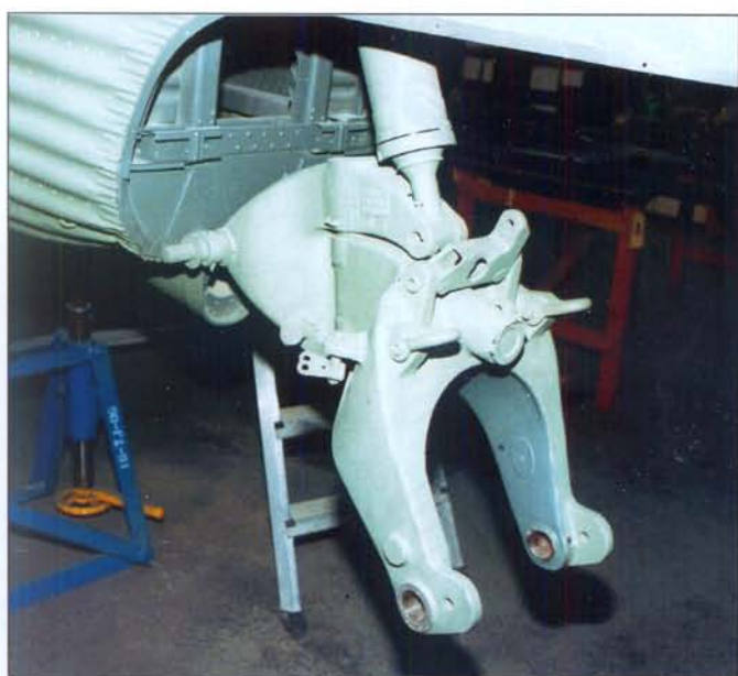
Tail wheel yoke and shock absorber.
