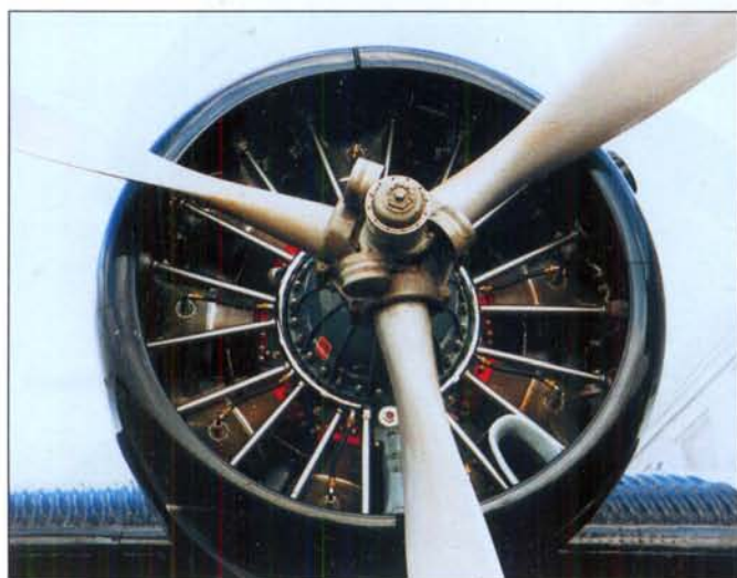
Head-on shot of the replacement Pratt and Whitney engine.
