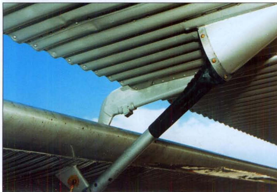
Aileron control rods on the port side of the wing.
