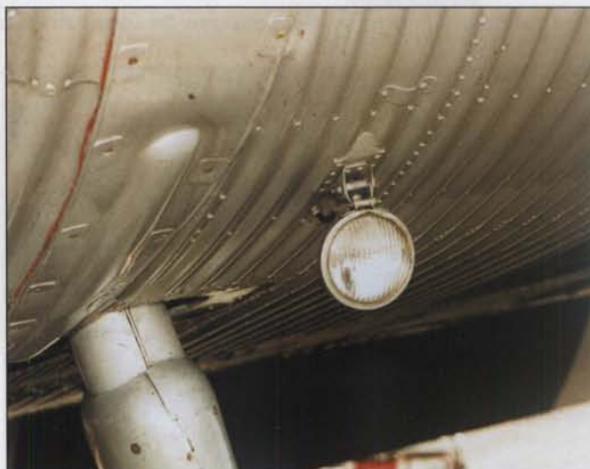
The landing-light situated on the wing forward of the left undercarriage.
