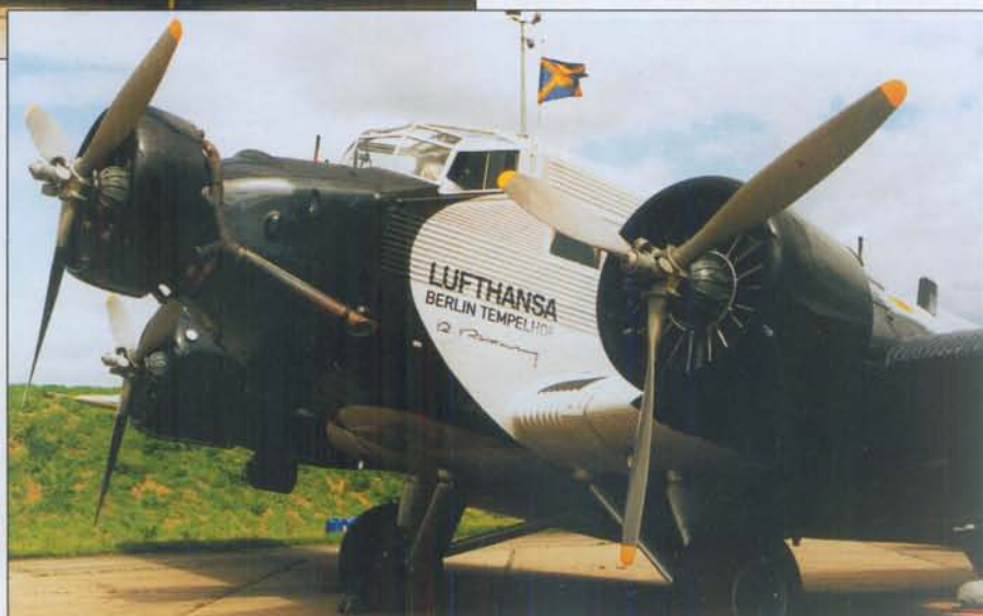
Front view of the aircraft; notice the replacement American engines, the original German BMW 132 engines being worn out due to age.
