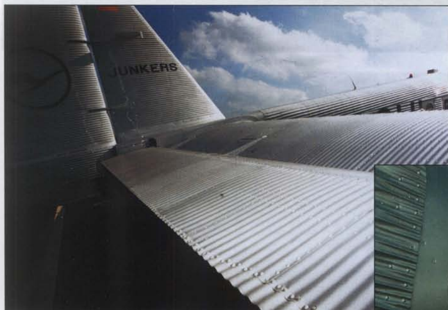
Tail surface views revealing a number of interesting design elements including the distinctive riveting patterns.
