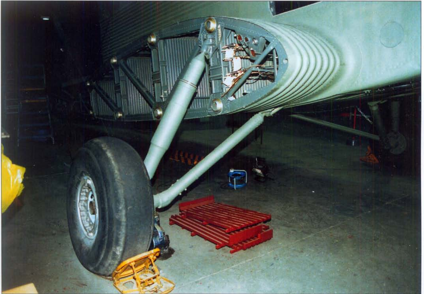
Wing rooth showing undercarriage attachment.
