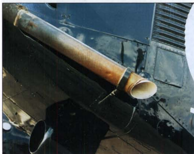
This picture perfectly shows the exhaust staining.
