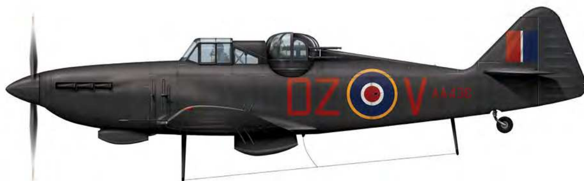
Boulton Paul Defiant NF.II AA436 DZ-V. Based at RAF Wittering, with 151 Squadron, in 1941. The NF.II was powered by a 1,280hp Rolls-Royce Merlin XX Engine and was fitted with the AI Mk.IV Airborne Interception Radar. Finished in overall Special Night RDM2A (Sooty Black). Codes and serial are in Dull Red, roundels were Type C1 on fuselage and Type B on the upper wings only, with standard fin flash
