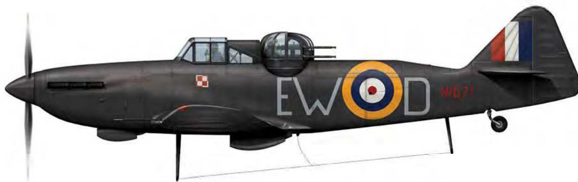
Boulton Paul Defiant NF.I N1671 EW-D. Based at RAF Kirton-in-Lindsey, Lincolnshire, with 307 (Polish) Squadron in 1940. Finished in overall Special Night RDM2A (Sooty Black). Codes are non-standard style in Medium Sea Grey. Roundels were Type A1 on fuselage and Type B on the upper wings only. Shown here with the earlier type fin flash. Currently on display at the RAF Museum, it sports a later style fin flash. Of note here is the aft fuselage fairing shown lowered
