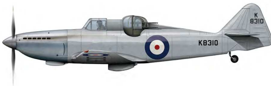
Boulton Paul Defiant (P.82) K8310, prototype. First flight August 11, 1937 from Wolverhampton in the hands of Boulton Paul's chief test pilot Cecil Feather. Powered by a 1,030hp Rolls-Royce Merlin I engine. It initially lacked a turret but is shown here when it was fitted in 1938/9. Overall Silver with Natural Metal cowling. With Type A roundels
