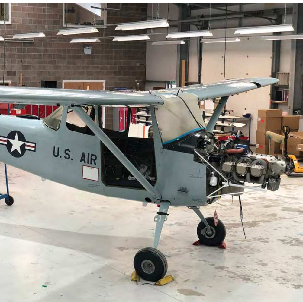
TOP: For the restoration of G-VNAM, the right wing pictured here needed some replacement skins, but the left wing required deconstruction to fix corrosion caused by operating around a coastal area for many years
