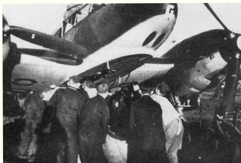
BELOW: Groundcrew installing the belly tank to a Messerschmitt Bf 110, which increased its range but severely impacted on its effectiveness in battle
