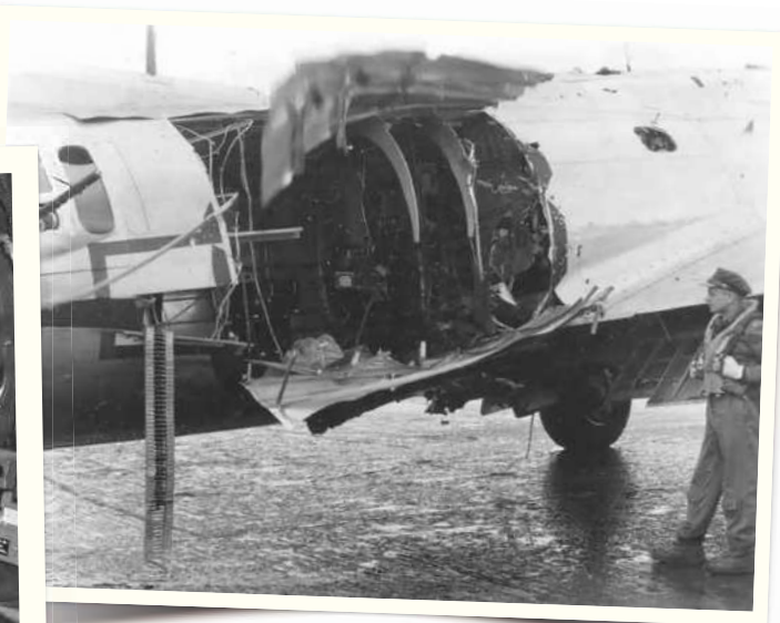
ABOVE: In a raid on Cologne on September 27, 1944, an 88mm shell entered the fuselage of B-17G 42-98004 and exploded, killing gunner Sergeant Kenneth Divil. The aircraft made it back to the 351st Bomb Group's base at Polebrook, Northamptonshire, where its pilot, Captain Jerome Geiger, was photographed surveying the damage DONALD NIJBOER
