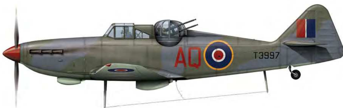
Boulton Paul Defiant ASR Mk.I T3997 AQ. Based at RAF Harrowbeer, Devon, with 276 (Air-Sea Rescue) Squadron in 1942. The ASR Mk.I was able to carry air-dropped M-type dinghies in a container under each wing (not illustrated here). Extra Dark Sea Grey and Dark Slate Grey upper surfaces with Sky undersides. Codes and spinner are Dull Red, roundels were Type C1 on fuselage and Type B on the upper wings and Type C under wings, with a standard tail flash
