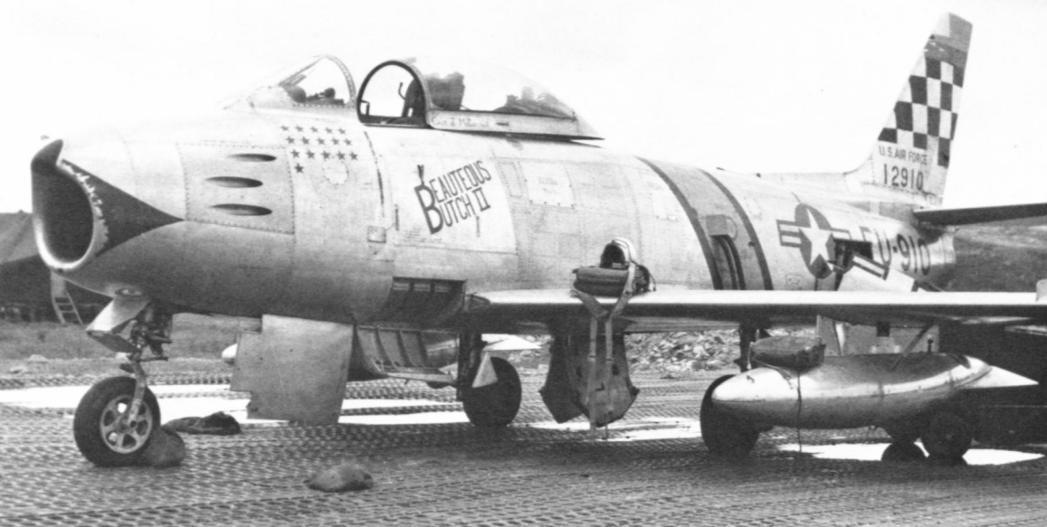
One of the last F-86s on active duty, this F was assigned to HQ USAF. Note the aluminum-painted surface, used as an anti-corrosion measure. The tail and drop tank stripes are red, white and blue. The pitot tube is red and white. (Menard)
