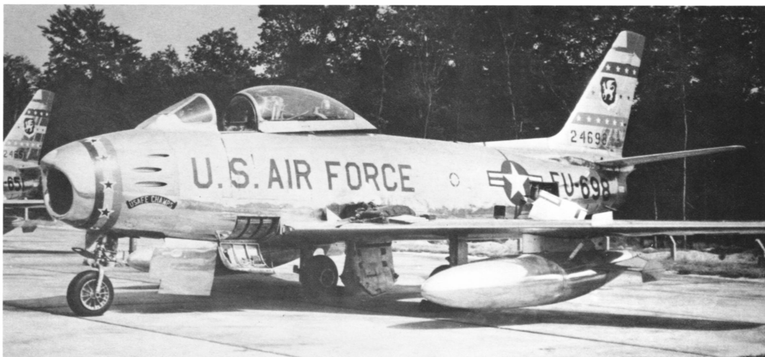
This highly polished F-86F is part of the 50th FBW gunnery team based at Landstuhl, Germany. Note the large 200 gallon underwing tanks. This is another 'bird' that shows up in the color section. (Menard)
