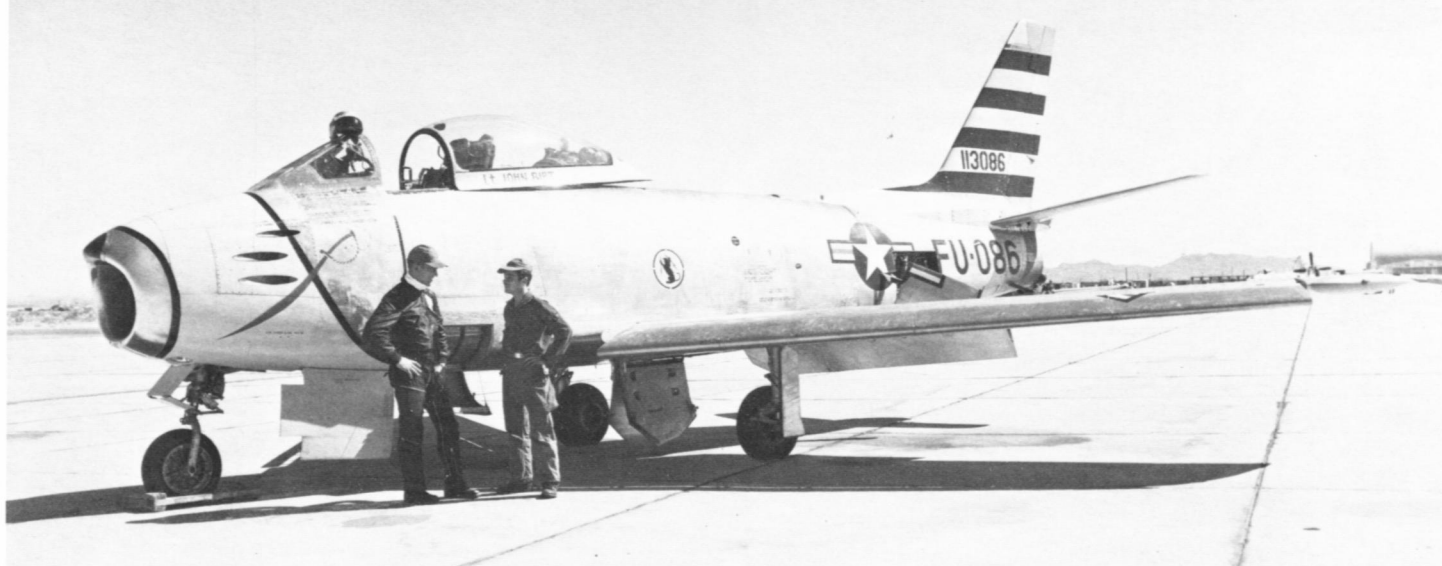
One of the F-86Fs illustrated in the color section, this Sabre was from the 84th FIS of Hamilton AFB, CA, one of the few units assigned to ADC to operate the F. Note that this aircraft retains the leading edge slats instead of the normal '6-3' wing with fences. (NAA)
