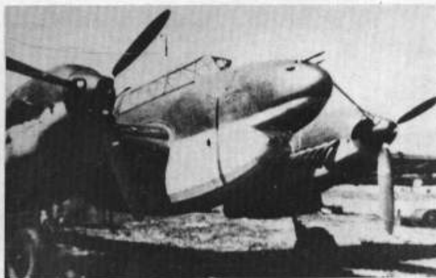
Left. Bf 110 of I/JG 52. Dragon emblem was black and white. Right. Bf 110D with "dackelbauch" (dachund belly) auxiliary fuel tank. Photos, Gerhard Ebers.
