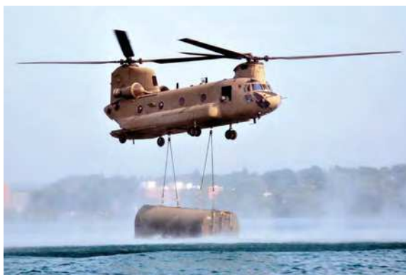
Above: A CH-47F operated by Detachment 1, Company B, 3rd Battalion, 238th Aviation Regiment, delivers a section of improved ribbon bridge bays in support of the Michigan National Guard's 1437th Multi-Role Bridge Company (MRBC) during a training evolution on August 12, 2018 Michigan National Guard
