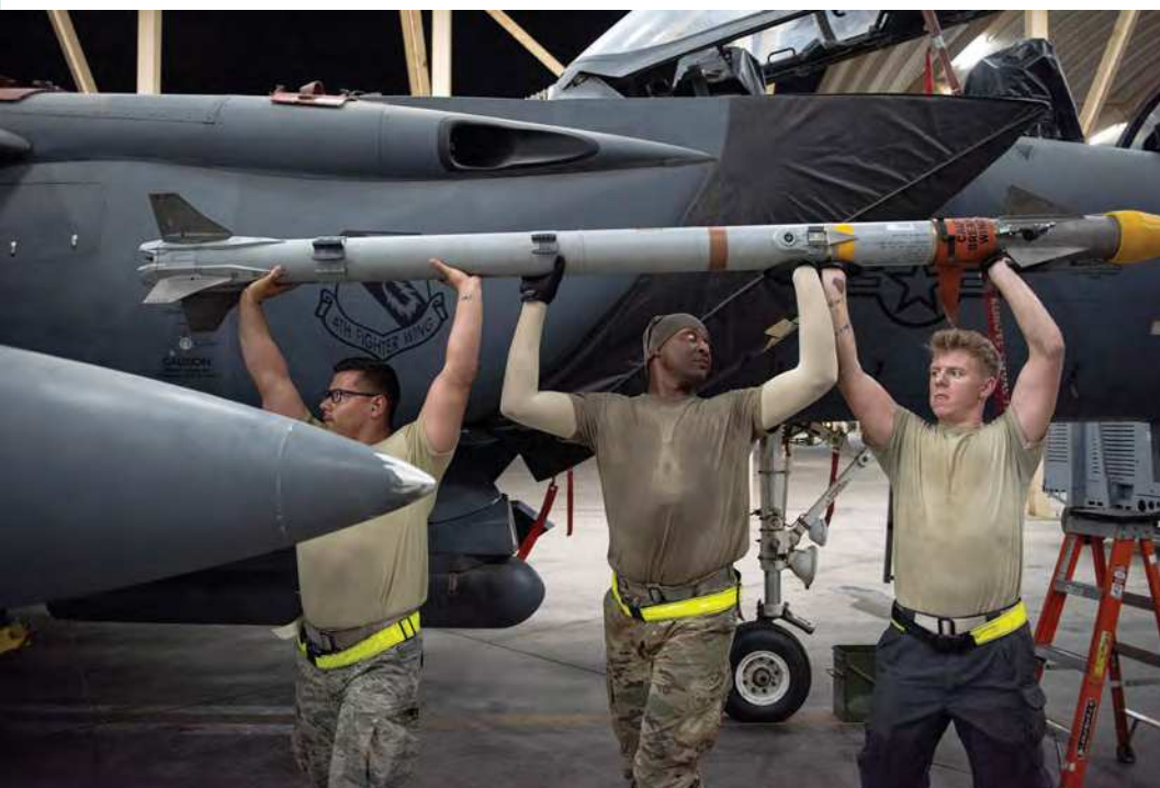
Above: An F-15E Strike Eagle weapons load crew team lifts an AIM-9X Sidewinder missile to attach to a pylon on July 15, 2019 at Al Dhafra Air Base, United Arab Emirates. The AIM-9X is an advanced infrared missile and the newest of the Sidewinder family of short-range air-to-air missiles carried on a wide range of fighter jets USAF/ Staff Sgt Chris Thornbury
