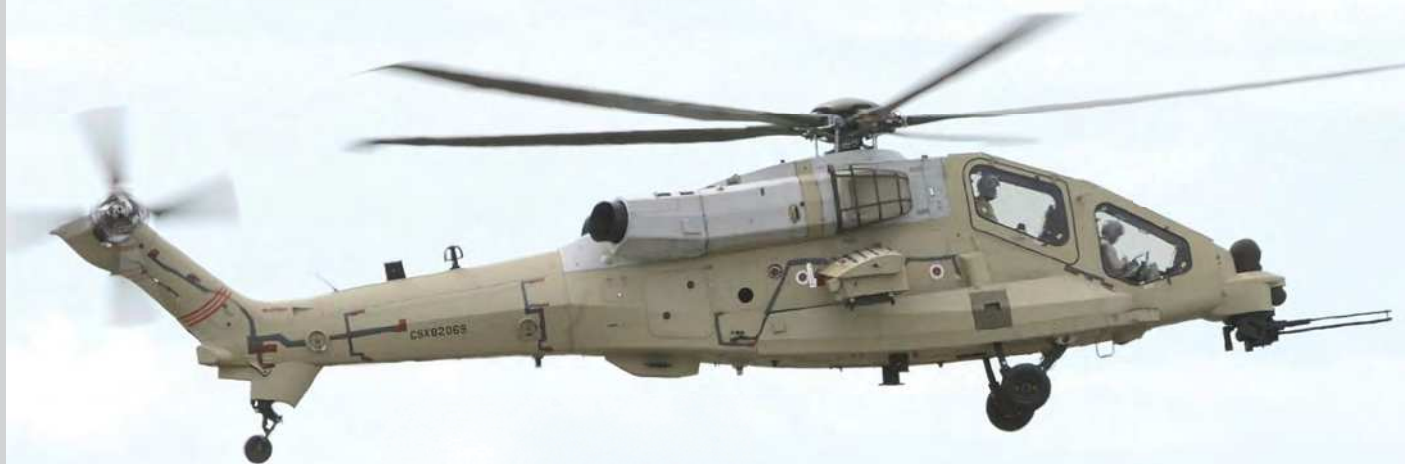
Leonardo Helicopters' AW249 attack helicopter prototype, CSX82069, completes its maiden flight on August 19. Note the TM 197B light turreted gun system under the nose Jeroen van Reijmersdal
