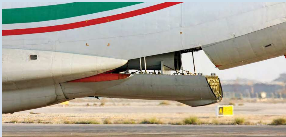
Left: The nozzles of the firefighting module installed on the Il-76TD, serialised 15-2284 Keyvan Tavakkoli
