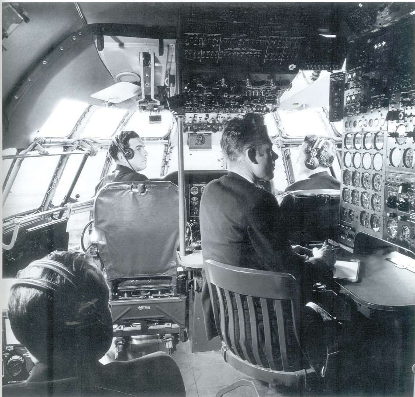
ABOVE: The Stratocruiser's flightdeck, or control cabin as it was referred to at the time, was a roomy and efficient workplace. The good visibility afforded by 2,864sq ft (266m 2 ) of window area can be clearly appreciated. The cockpit was arranged for a crew of five including the pilot, co-pilot, flight engineer, navigator and radio operator. Boeing
