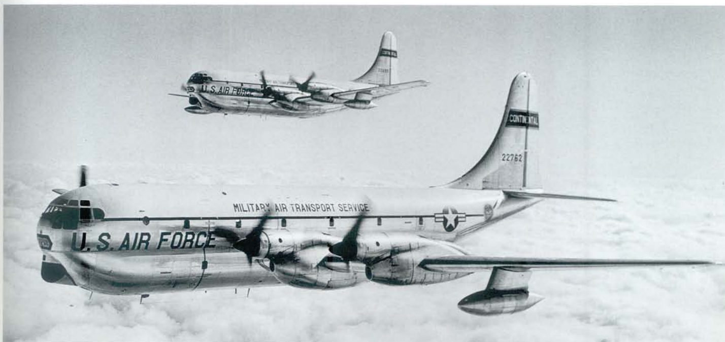
BELOW: The two turboprop powered YC-97J testbeds may be only a footnote in the C-97 story, but they hold a place of their own in the overall saga of the Stratocruiser. The YC-97Js were built to test the Pratt & Whitney T-34 turboprop engine, and a new three-bladed prop. They set many in-service performance records but the new engines were not adopted. However, both aircraft were later used to produce the B377SG Super Guppy conversion. USAF via Walter Klein
