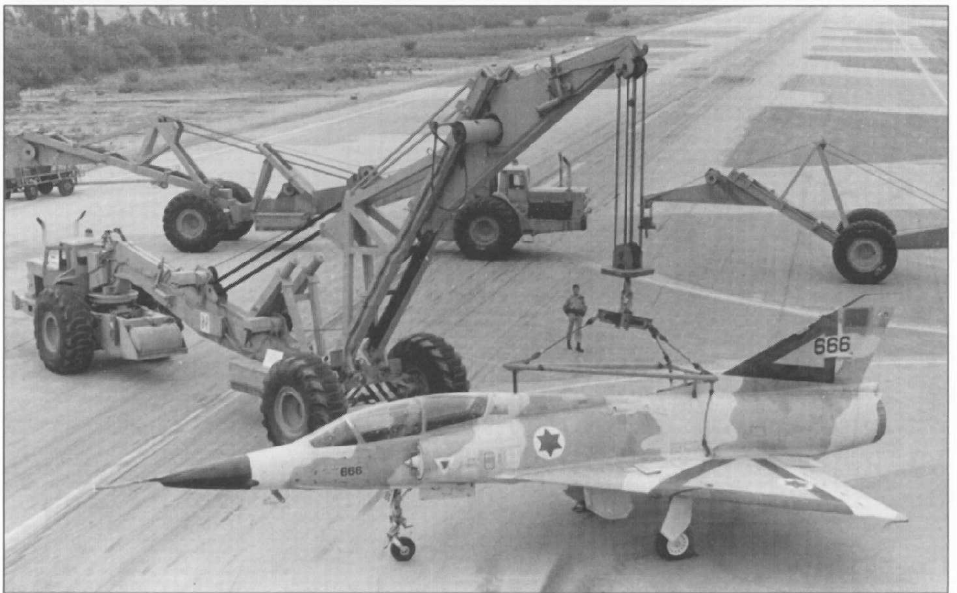
Three photos showing Nesher ground crew placing an a/c using crane, named in IAF "Gamal" (Camel in hebrew) to move it into its place for an a/c exhibition.
