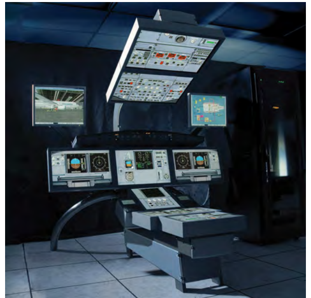
ABOVE • Fixed training devices are touch-screen based and are valuable for practising standard operating procedures (SOPs)
