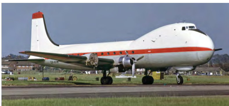
Two BAF Carvairs, including G-ASDC (c/n 7), were stripped of their paint, enabling their payloads to be increased by 1.5 tons RICHARD VANDERVORD
