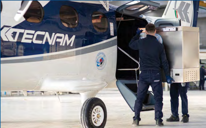
Tecnam and ultra-freezer manufacturer Desmon have modified the P2012 Traveller to leverage the aircraft's short field performance to transport up to 115,000 vaccines to less easily accessible areas TECNAM
