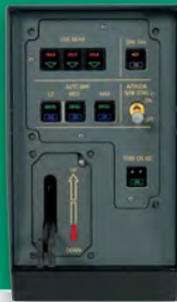
P&P ABRK Panel Real size Auto Brake with Landing Gear combo panel.
