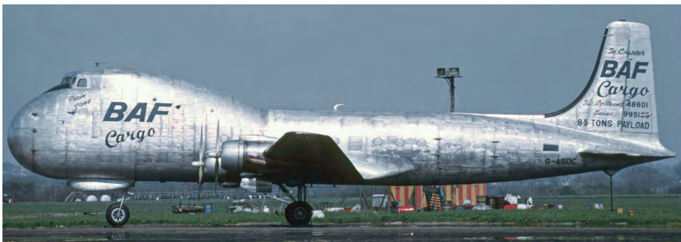
Two BAF Carvairs, including G-ASDC (c/n 7), were stripped of their paint, enabling their payloads to be increased by 1.5 tons RICHARD VANDERVORD
