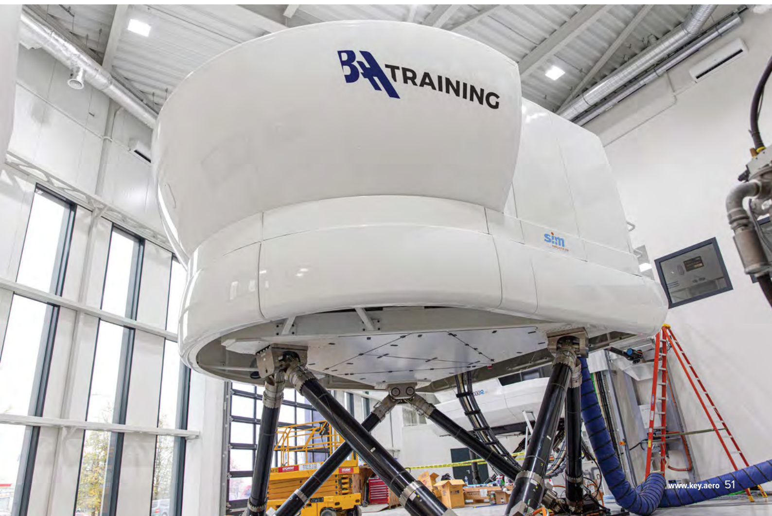
Full-flight simulators are either hydraulic or pneumatically powered and provide full motion in six degrees of axis BAA TRAINING
