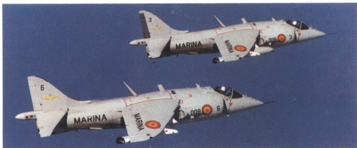
Above: Two Spanish Navy AV-8A Matadors. No 3 appears to have a replacement rudder.
