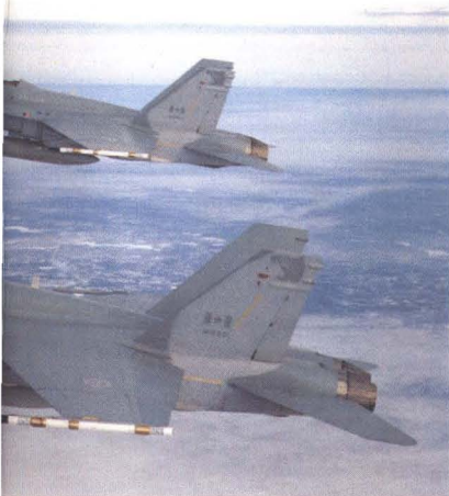
Above: Canada plans to have 138 CF-18s. These two-seaters of 410 Sqn are in standard toned-down colours (FS 35237 blue-grey on upper surface, FS 36118 dark grey for false canopy).
