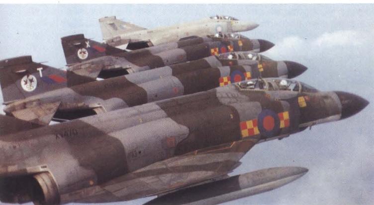
Above: Camouflaged Phantoms of 92 Sqn, RAF, formate with a lone grey example illustrating the effectiveness of the lighter colours for fighter operations.
