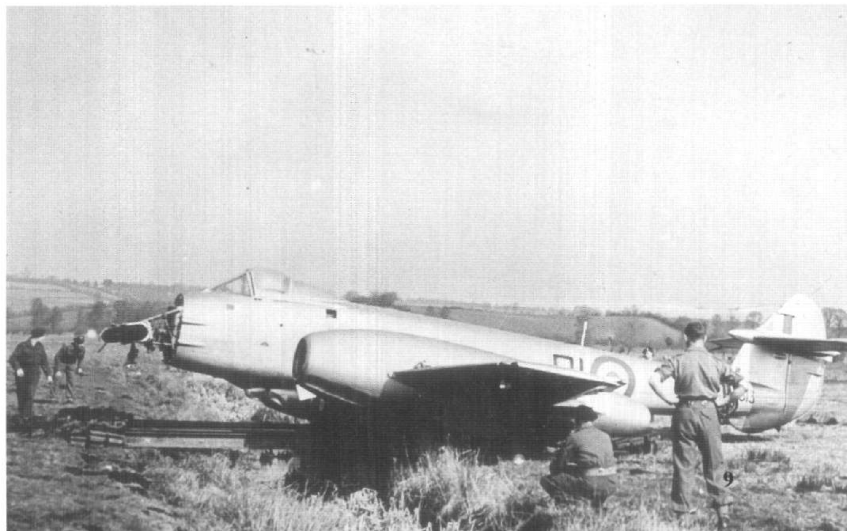
This Meteor F 4 of No 209 AFS made a crash landing on 12 February 1954. The aircraft ripped off the nose wheel and the nose cone when it hit a ditch after running off the runway. VT318 was written off because of the damage inflicted in this crash. (Westonzoyland Research Group)
