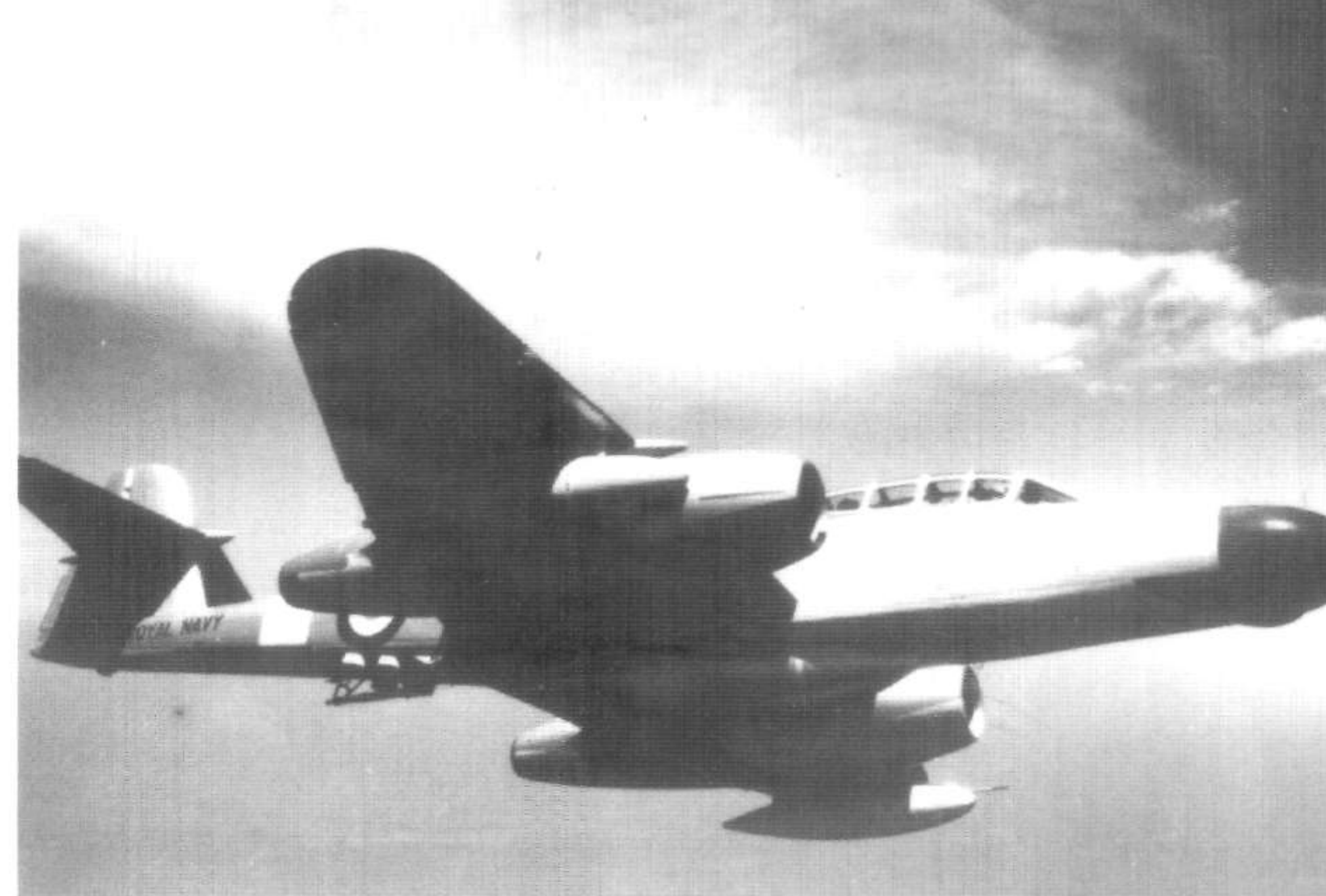
This TT 20 of the Fleet Air Arm was a rebuilt and converted NF 11 night-fighter. The wind driven wench was mounted above the wing and the target attachment point/cable guide was mounted on the fuselage underside. The TT 20s carried Black diagonal stripes painted across the underside of the aircraft to make them more visible to the gun crews during firing practice. This aircraft of No 728 Squadron, Fleet Air Arm was based at Hal Far, Malta during 1958. (Fleet Air Arm Museum)
