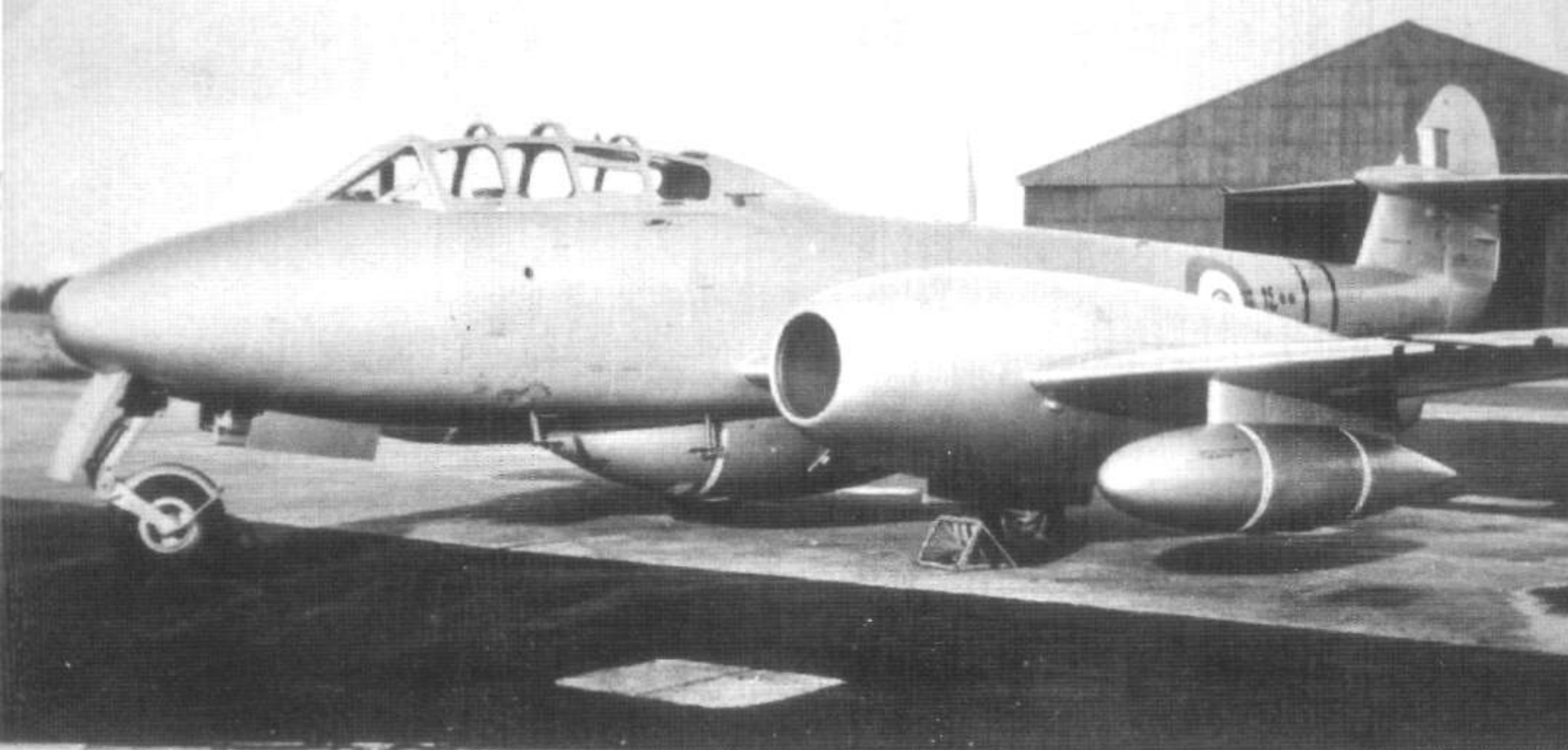
A Meteor T 7 of the Royal Egyptian Air Force probably on the Gloster ramp prior to delivery during 1949. The aircraft was finished in overall Silver lacquer with Black identification bands around the wings and rear fuselage. The aircraft's serial number was carried on the fuselage side, just behind the roundel in Black Arabic numerals. The aircraft was one of six T 7s ordered by Egypt. (Dr. David Nicolle)
