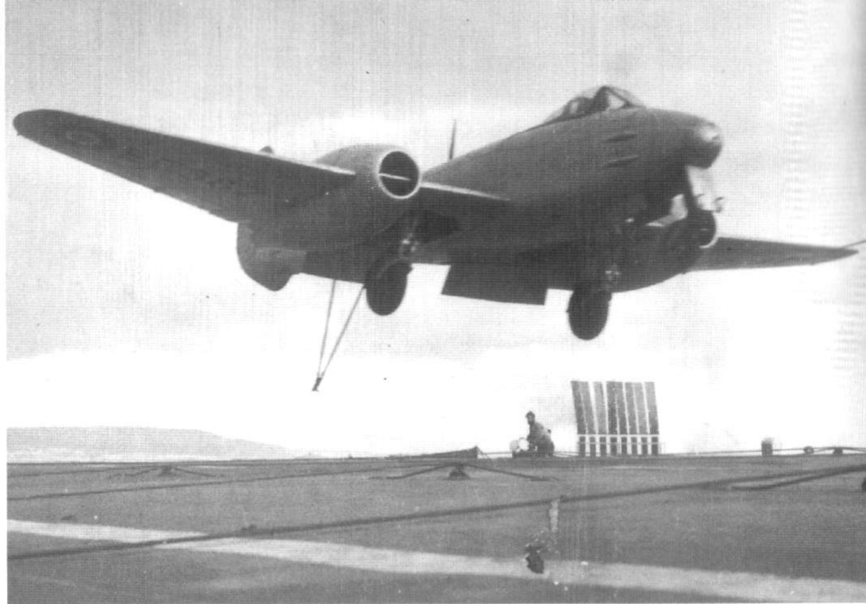
A modified Meteor F 3 (EE387) makes a successful deck landing on a Royal Navy aircraft carrier during 1948. Even though the tests were highly successful, the Navy opted for the Supermarine Attacker as its first carrier jet. (Fleet Air Arm Museum)
