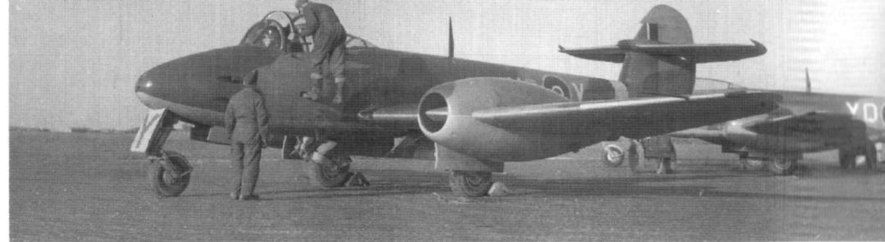
A pair of Meteor F 1s of No 616 Squadron on the PSP ramp of RAF Manston during 1944. The side hinged canopy was only used on the Meteor F 1. The aircraft individual code letter, Y, is repeated on the nose wheel door. (Imperial War Museum)
