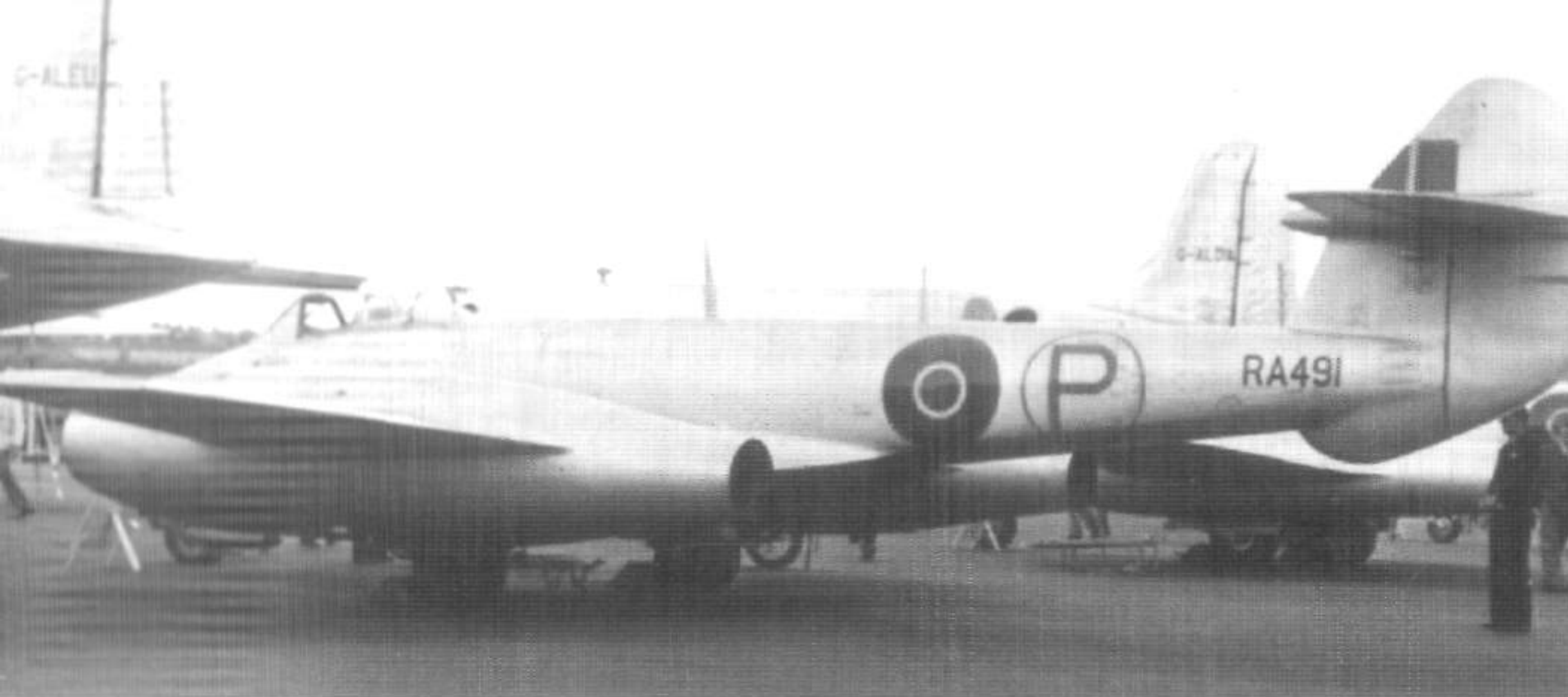
This Meteor F 4 (RA 491) also had modified engine nacelles marking it as an engine test bed. The aircraft was used by Rolls-Royce to test the Avon engine. (MAP)
