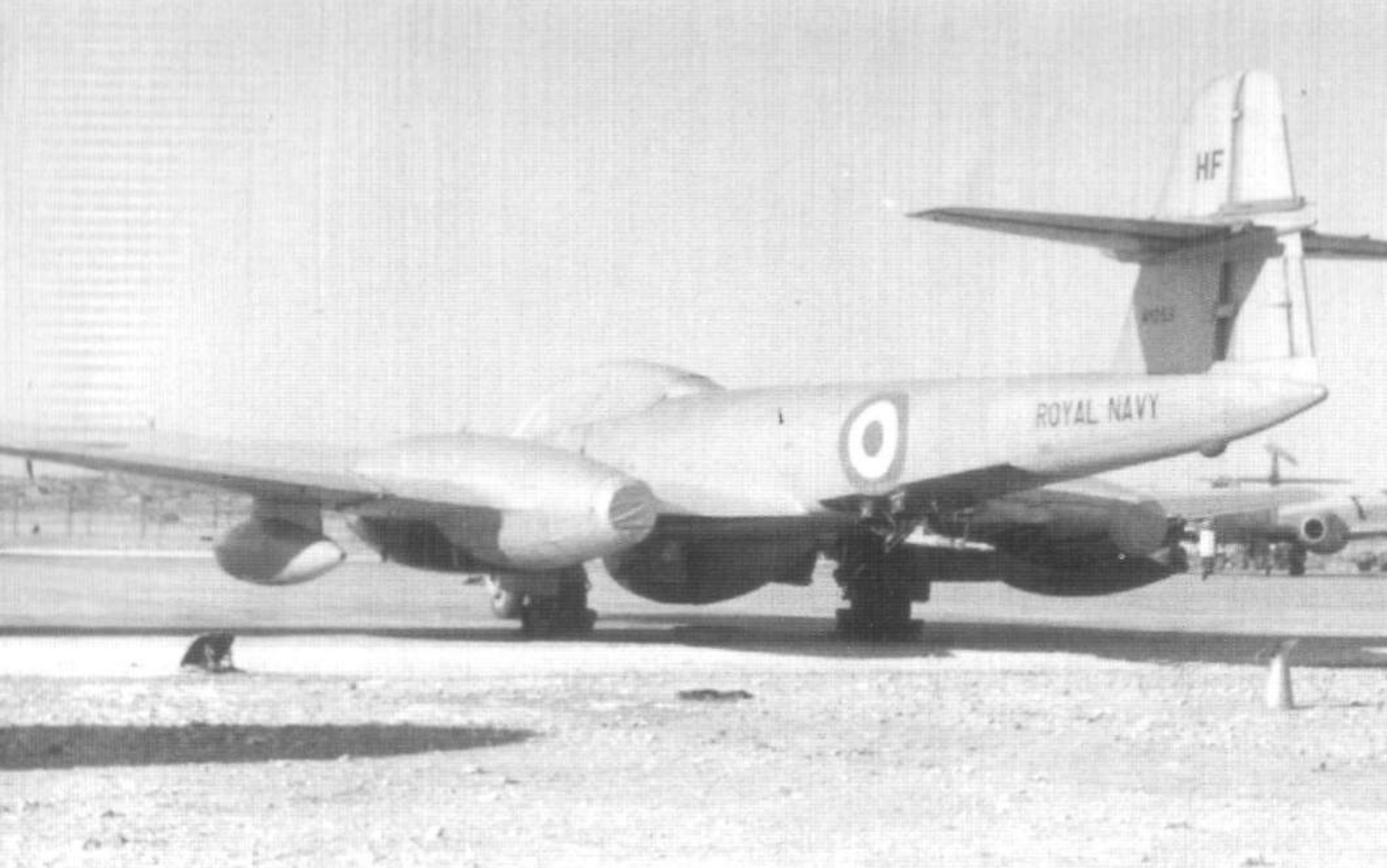
The lower fuselage target towing cable guide and target attachment point are visible on the Meteor TT 20 (ex-NF 11) of the Royal Navy Fleet Air Arm. The aircraft was flown by No 728 Squadron at Akrotiri during 1959. This aircraft was later sold to France during 1974. (MAP)
