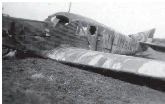
Junkers F.13 "Illimani" after a belly landing in the Bolivian orient. It was later repaired and returned to service. Note the tactic cammo applied. ( Fuerza Aérea Boliviana )
