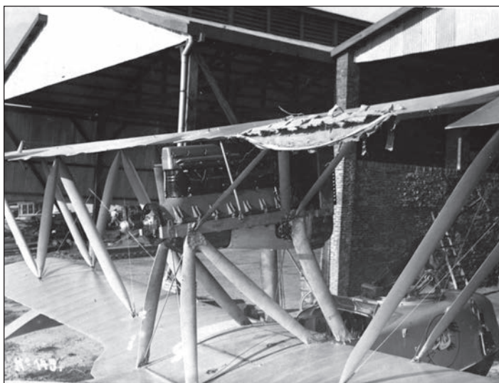
A Macchi M-18A.R. at Sajonia NAS showing some damage in the upper wing, probably due to AA fire. The propeller had been removed from the 250hp six-cylinder Isotta-Fraschini engine. (Archivo de la Armada Nacional)
