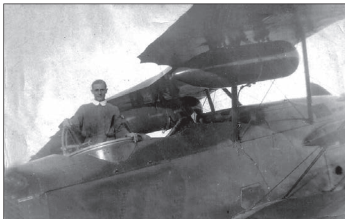
NCO MAM Evasio Perinciolo in the gunner's rear cockpit of a Potez 25A.2 bomber. The two auxiliary tanks can be seen under the upper wing. ( Instituto de Historia y Museo Militar del MDN )
