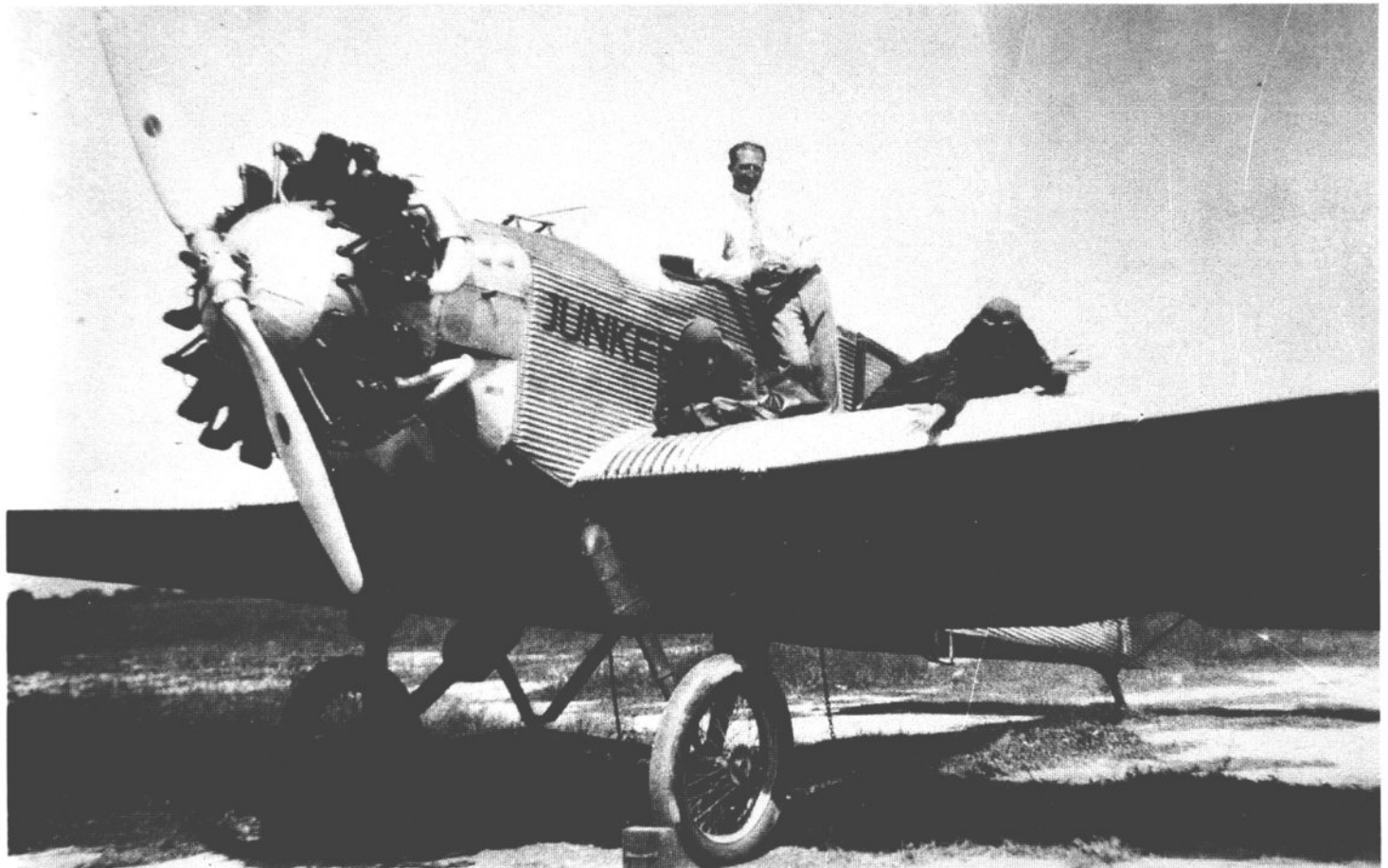
Another view of Junkers W 34ci "Vanguardia" also in 1934, but by which time its engine mount area, previously painted black, had been cleaned up and all paint removed from metal surfaces. (Antonio Sapienza Collection).
