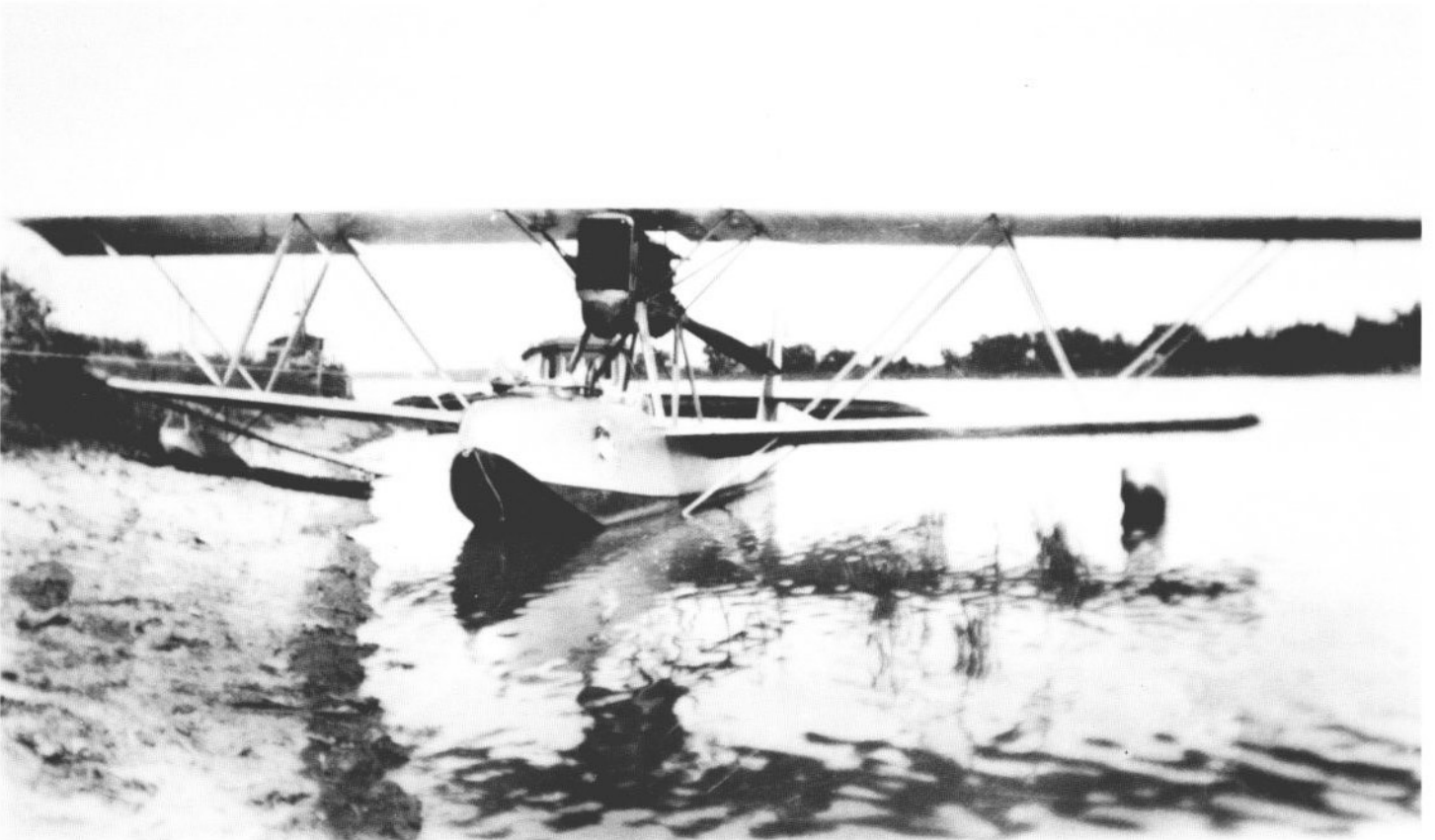
Head-on view showing the distinctive strut system of the Paraguayan Macchi M.18A.R., in this case serial R-5 at Sajonia Naval Air Station circa 1934 (Archivo Cnel Av. (S.R.) A. Pasmor).
