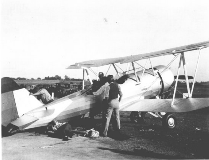
Believed to be the very first C14R “Osprey” for Bolivia in full Bolivian markings at the factory, minus serial number. Both the fixed forward gun and the rear gun were in place. Note the short tail wheel configuration, later altered in Bolivia to improve take-off and rough field handling (Hagedorn Collection).
