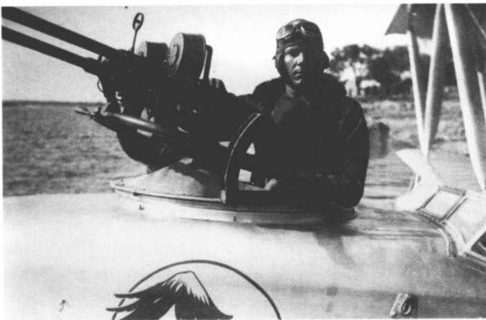
Another view of the bow turret of a Paraguayan Naval Macchi M.18A.R., in this case mounting twin Madsen 7.7mm guns. The officer at the guns is Lt.(Res). Job von Zastrow and the photo was taken at Bahia Negra in 1934 (Aviación Naval Paraguaya).
