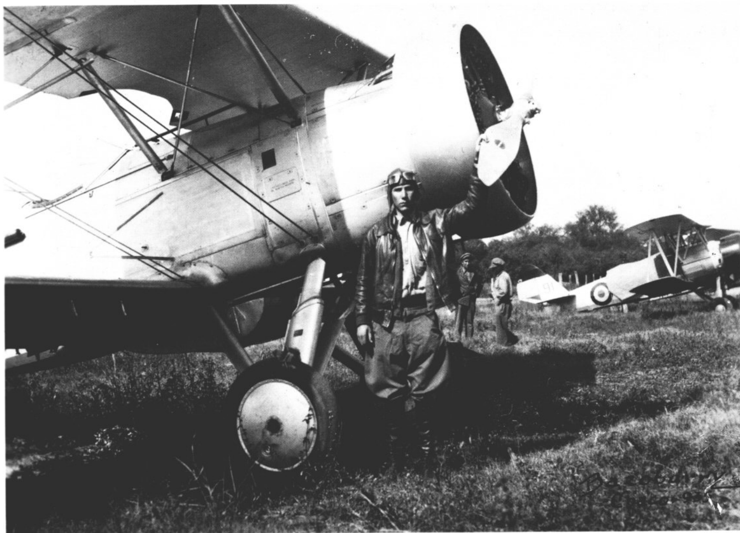
This photo proves that Bolivia received at least two distinctly different variants of the "Cyclone Falcon." Note the differences between the undercarriage members, belly slip-tank, and standard wind-screen on this example at Villa Montes during the war. (via Ramiro Molina Alanes).
