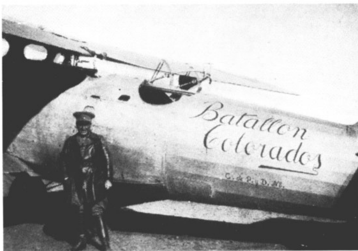
Another, closer view of Breguet 19 A2 "Batallón Colorados." The Breguet 19 was a much larger aircraft than commonly thought, and suffered from its narrow track undercarriage at the rugged El Alto aerodrome (Hagedorn Collection).
