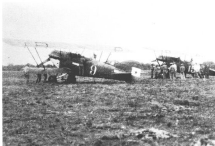
Potez 25 T.O.E.'s serials 9 and 15 (the former s/n 8, rebuilt after a major accident) at Isla Poí in 1934 fully marked. Note that, contrary to many previously published accounts, the forward lower engine cowl was left natural metal to aid maintenance crews in keeping the aircraft clean. (Archivo Cnel. Av. (S.R). A. Pasmor).
