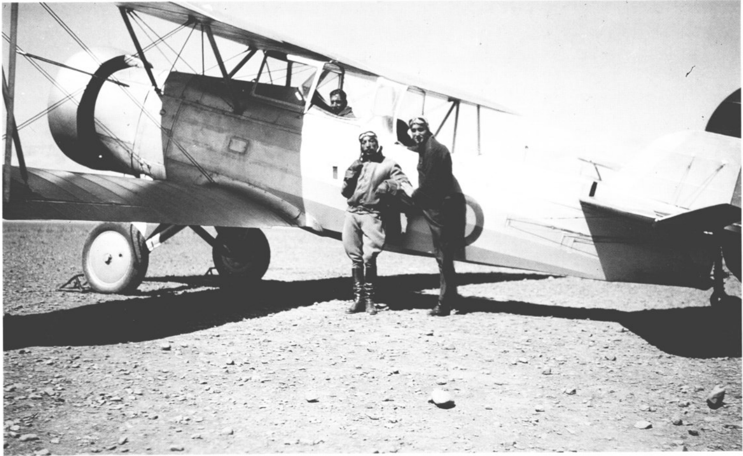
On this Bolivian "Cyclone Falcon," the national colors have been extended completely forward on the upper rudder and no individual serial has been assigned. The canopy, in an open position, slid forward as shown, giving a rather unusual appearance. One of the officers pictured is Tie. Claudio Lopez Cordova, and the picture was taken at El Alto in 1936, after the end of the war (via Ramiro Molina Alanes).
