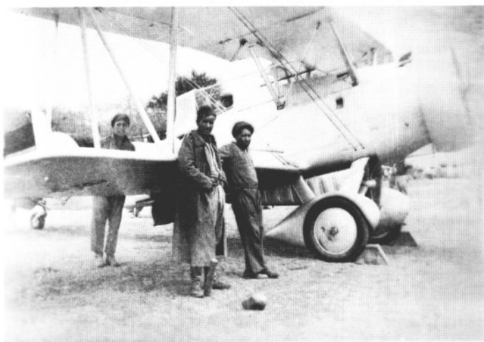
Evidence that Bolivia's "Cyclone Falcons" used the rarely seen ventral auxiliary fuel tank and wheel spats. This example, photographed at Villa Montes in 1935, is also noteworthy in that the national color apparently only occupied the upper-half of the rudder. Compare this image to the next photo (via Antonio L. Sapienza).
