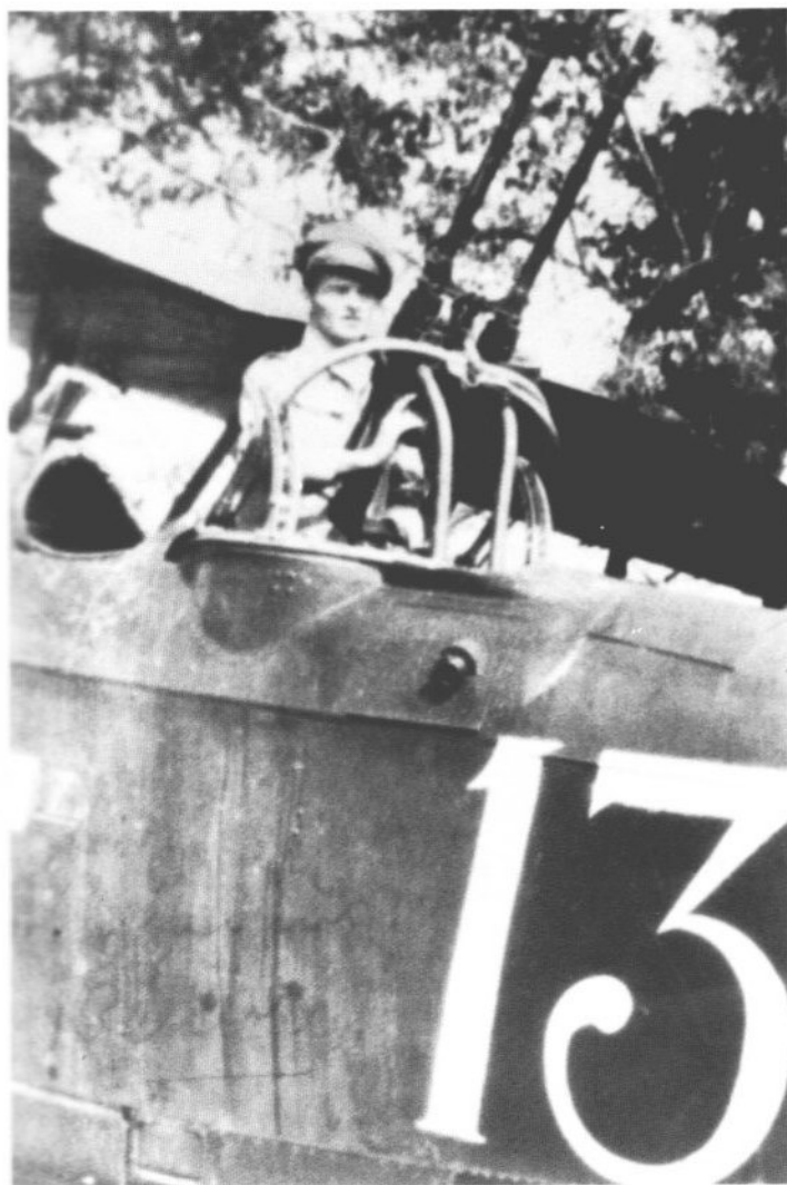
An excellent close-up view of the twin Madsen machine guns on Paraguayan Potez 25 T.O.E. serial 13 at Isla Poí in 1933. This form of stylized numeral was common on Paraguayan aircraft, whereas Bolivian aircraft tended towards more blocked numerals. (Archivo Cnel. Av. (S.R). A. Pasmor).
