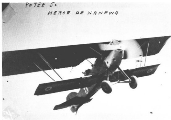
Potez 25 A2 serial 5 shown returning from a mission over Nanawa in January 1933. Note the seldom seen underwing "salvo" racks for up to six light bombs each and the standard national insignia roundels (Archivo TCnel Carlos R. Peralta).
