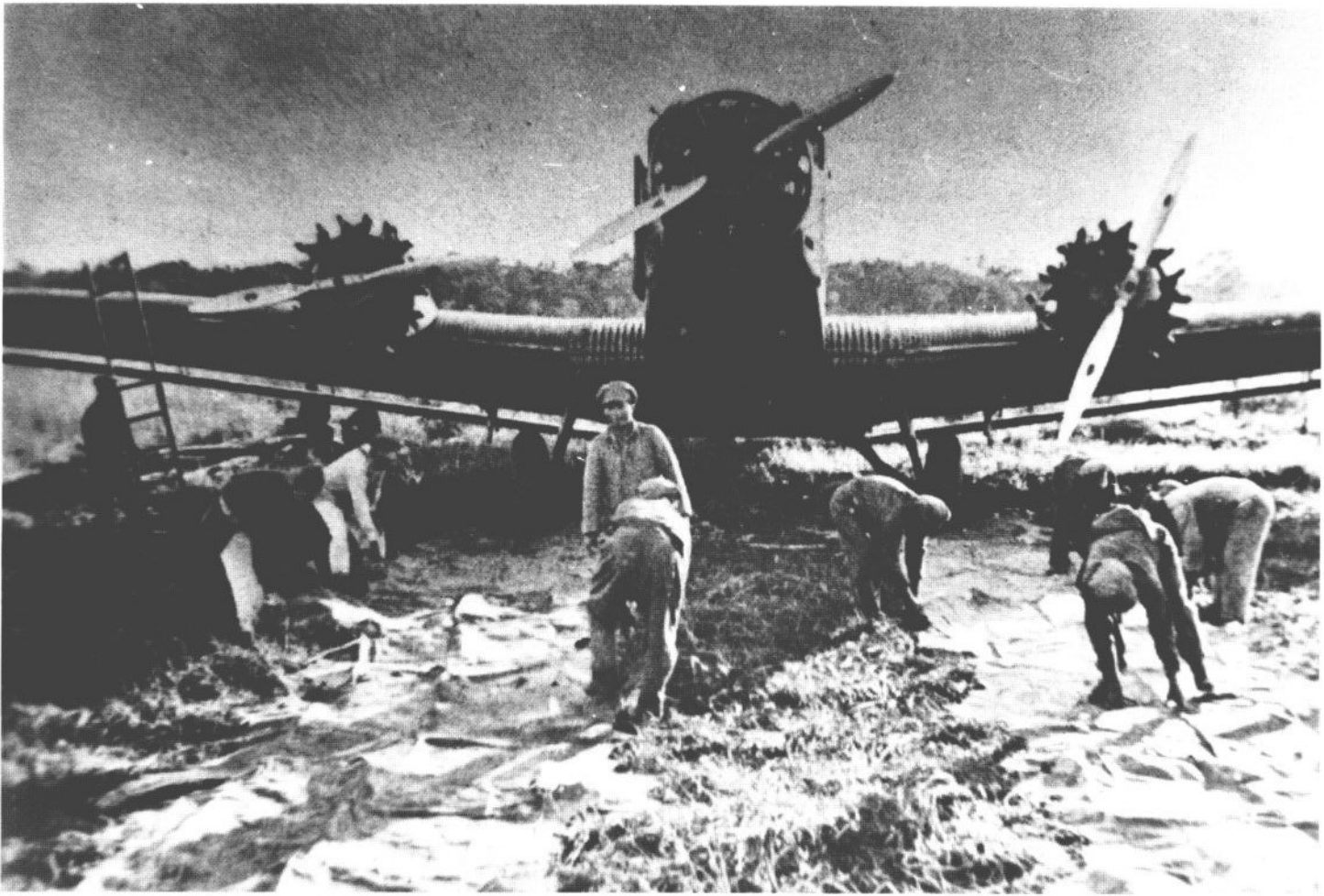
Perhaps the most prized Bolivian assets of all were the LAB Junkers Ju 52/3m transports, one of which is shown here being prepared for a crude-field take-off at Machareti, north of Villa Montes, in 1933. Note the absence of speed rings on the outboard engines. This is probably "Chorolque." (LAB via Juan Arraez Cerdá).
