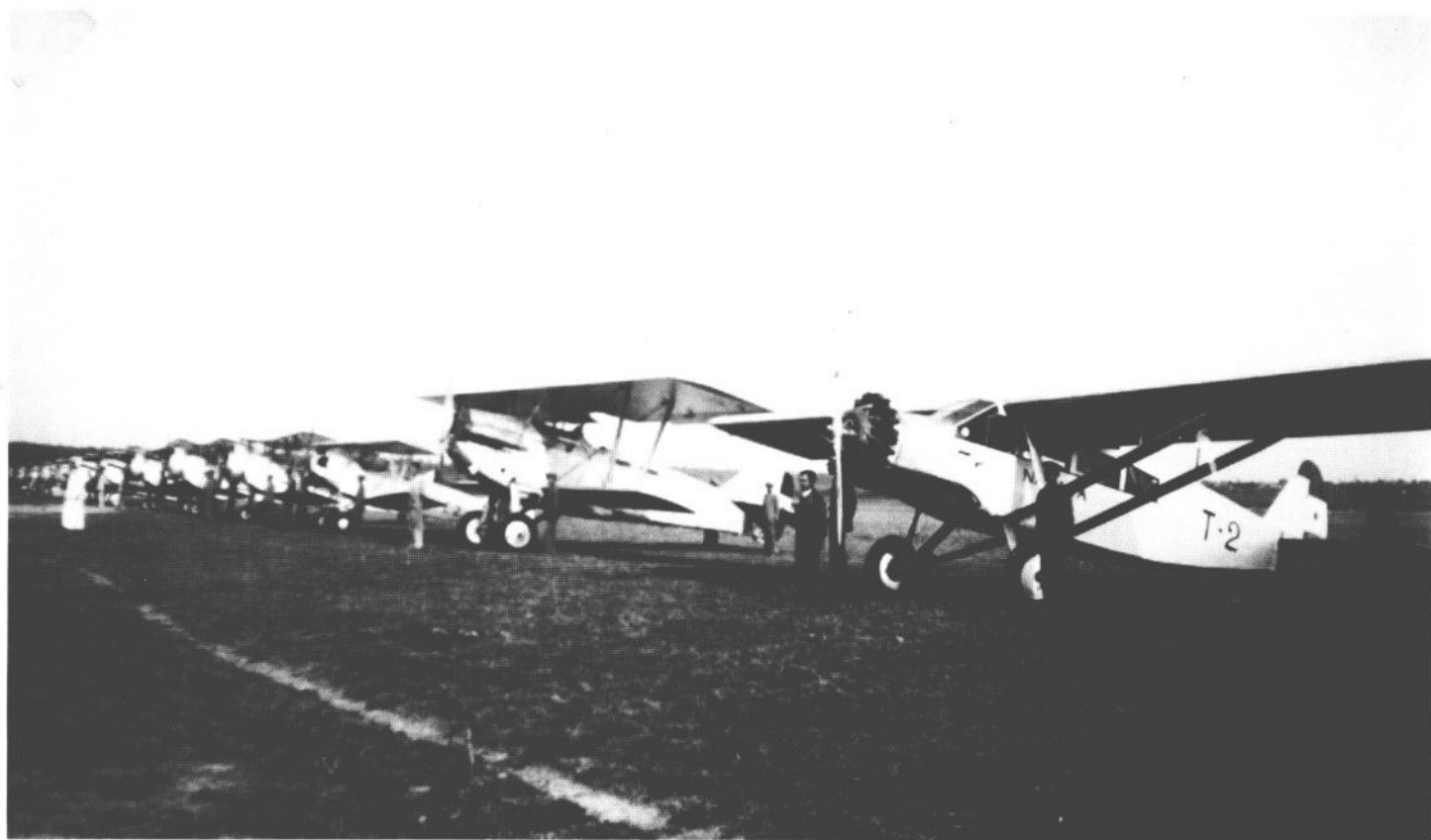
A second Travel Air Model S-6000B was also acquired by Paraguay and coded T-2 and, by the time of this April 1939 photo, had also gained the name "Nanawa." Note the doped aluminum colored Potez 25 second in line with the two cabin slit windows and enclosure for passenger carrying duties. Next in line is a Fleet Model 2 then three Breda Ba 25 trainers (Archivo Cnel. Av. (R.S). A. Pasmor).
